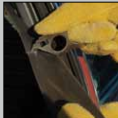
The Extrik-8-R quickly cuts through seat belts in one quick stroke with no risk to responder or victim.
