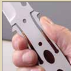
To release the knives, just press these two spring catches, which are integral with the blade tang.
