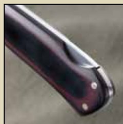
The butt showing the lockback lever, stainless steel back spacers and assembly pins, all hand polished flush.
