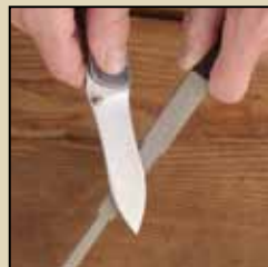
Use the flat side to put an edge on knives and tools with plain cutting edges, and to remove the burr on the back side.
