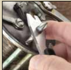
Just insert the hex bit into the 6 mm wrench to use the Ta-Bar Tool as a T-driver for flat and Phillips head screws.
