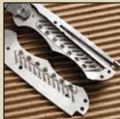
Diamond-coated springs hone the cutting edges at precise angles every time an Edgie is closed and opened.
