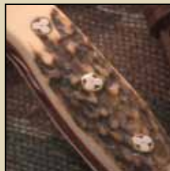
The Brow Tine features stag handles held by brass and stainless steel mosaic pins in the traditional manner.
