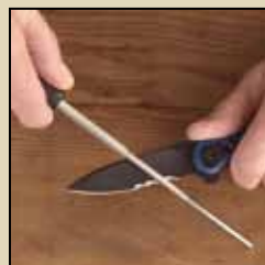
The six stepped-cylindrical sections of the sharpening rods give you the right size for almost any serration.
