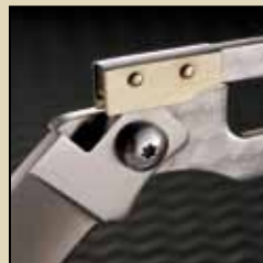
These polished brass “mini-liners” position the blade laterally in the open position, adding rigidity.
