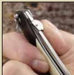
The OutBurst assisted opening mechanism cannot be actuated until you rotate the Fire Safe disk and nudge it up.
