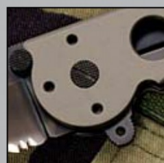
The trademark Carson Flipper speeds opening and acts as a blade guard. The thumb studs are also the blade stop.
