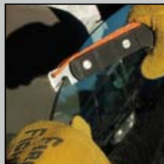
Use the M.A.K.-1 twist breaker for controlled breaking of windows or the carbide butt breaker for shattering.
