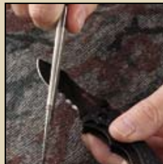
You can use the rounded tapered edges of the P.T.S. to sharpen a variety of serrations, including exclusive CRKT Veff Serrations.
