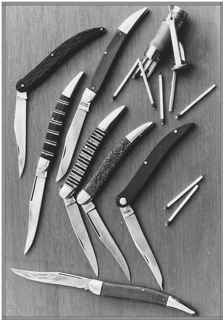
The Texas toothpick at bottom was made by Imperial in the 1920s. Above it to the right is a red celluloid KA-BAR with bird's-eye rivets and no bolsters. To the left of it is a mottled-celluloid Imperial model and a rare glitterstripe Kutmaster. The one at top was made by Wards, and the candystripe to the left of it was made by Imperial. The piece at the top left is unmarked. (White photo)
