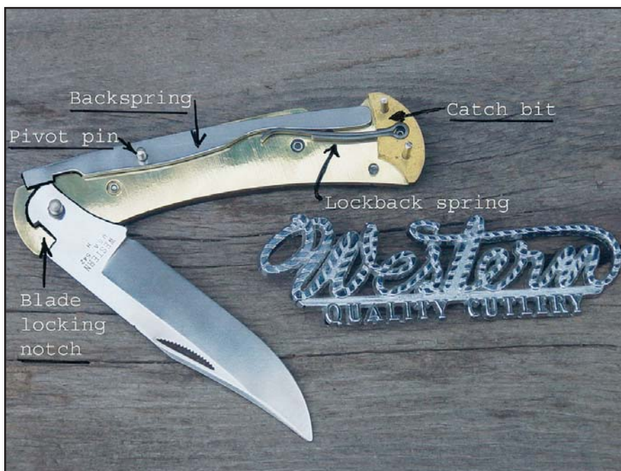
A partially assembled Western model 54 lockback folding hunter shows the backspring with its blade-locking notch, the notched master blade, and the brass catch bit that holds the tempered spring, which secures the blade in the open position. The spring must be strong enough to hold the blade open but flexible enough so that the user can press down on the back of the backspring and release the blade from the locking notch. (White photo)
