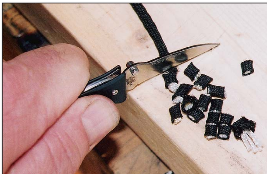
The 550 paracord offered little resistance to the Two Can's 420J2 stainless blade.
