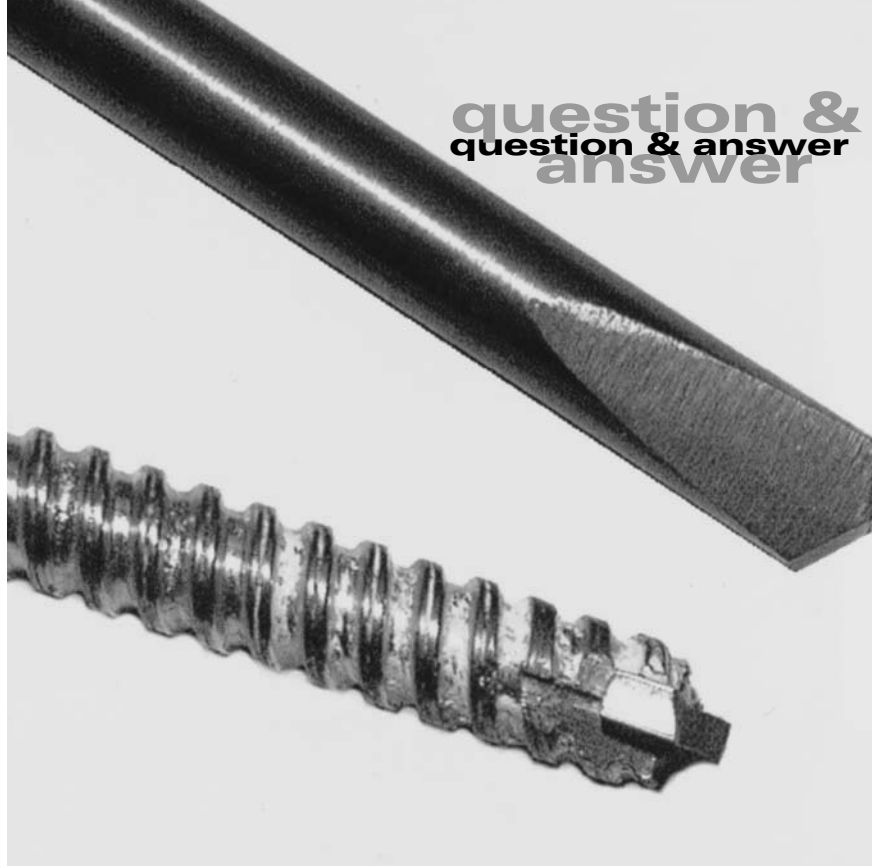
ILLUSTRATION #4 The bit at the top is a tungsten-carbide spade-type drill designed for use on hard steel. The bottom bit is the yard-sale masonry bit the author used to drill the planer blade as shown in Illustration #3 on p. 91. (Goddard photo)
