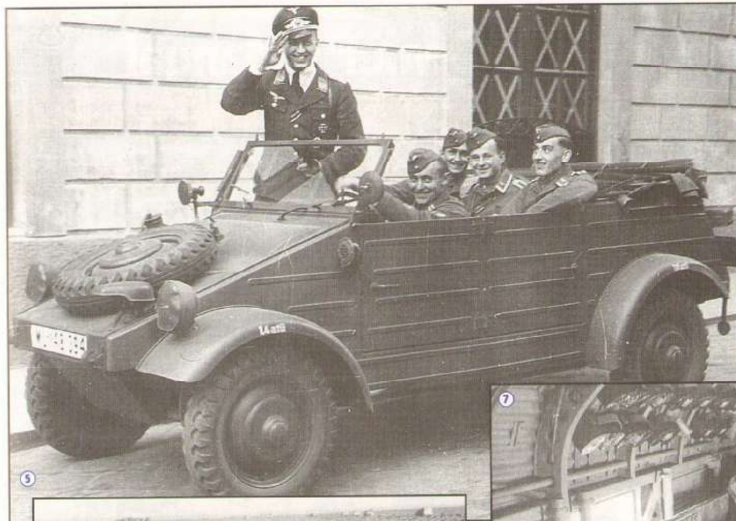
5. Fine study of an early Kübelwagen in Luftwaffe service. Note the hub-caps, spotlight, long spokes on the spare mount, short rear fenders, and turn signals on the windshield. The defining feature is the wiper cable emerging in front of the windshield, a feature introduced in 1941. The rear fenders would be lengthened in November of that year. (BA) 6. The driver of this Kübel operates the tire pump, normally stowed on the inside of the engine cover. With no jack holes and the shovel on the right side, this Kübelwagen is a 1941 model. (BA) 7. Squeezed into a Ju-52, this Wehrmacht Kübelwagen sports the treadless version of the balloon tires. Note that the wheels and fenders have been removed to transport the vehicle inside the tight confines of the aircraft. Interestingly, this Kübel features both long spokes on the spare mount and the curved reinforcement plate. (BA)
