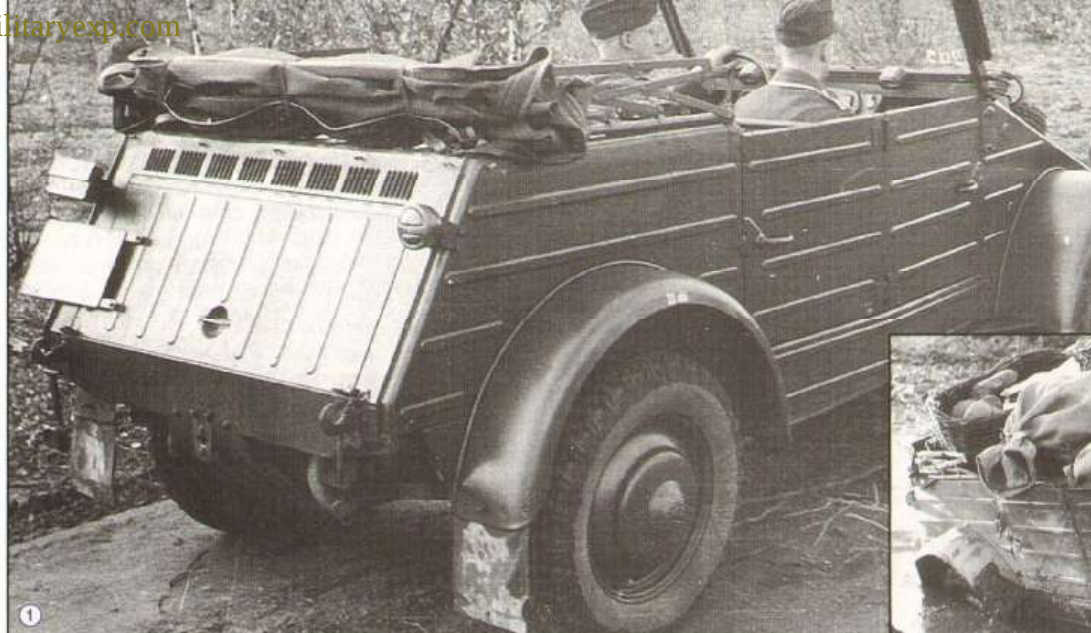
1. This sharp Kübelwagen is an early '42 model and is a fine example of how the round taillight was affixed. Note the lengthened rear fenders and narrower engine guard. 2. Supper's going to be late, boys! An early '42 Kübelwagen packed with groceries. 3. A schwimmwagen loaded to the gills. Note the tool box mounted beneath the right side of the dash.
