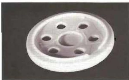
The inner rim on the 'close' road wheel conflicted with the guide horn on the track. At first I thought of just removing the slot as shown, but then I just look off the whole rim. The modification is completely invisible with the track installed.
