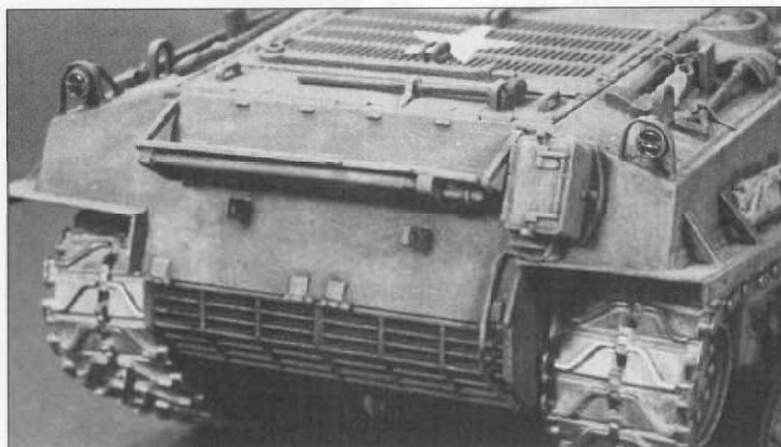
Left: the re-fill tube described in the text. Below and right: the rear vent supports.
