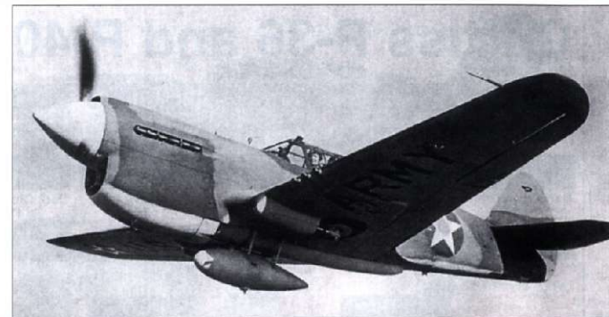
This is a fine example of a P-40E in British-style Temperate Land Scheme colours, but using US-manufactured equivalent paints. In this instance the colours consist of Specification 14057 Sand 26, (or possibly Red Brown 34), and Dark Green 30 uppersurfaces over Light Blue 27 undersides.
