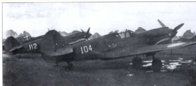
A line-up of P-40Es of the 23rd Fighter Group - the 'Flying Tigers' - which appear to be in the Olive Drab/Neutral Gray scheme. Note the Walt Disney Studios-designed 'Flying Tiger' decal on the fuselage sides and the continuation of the white identification numerals from the original AVG numbering sequence.
