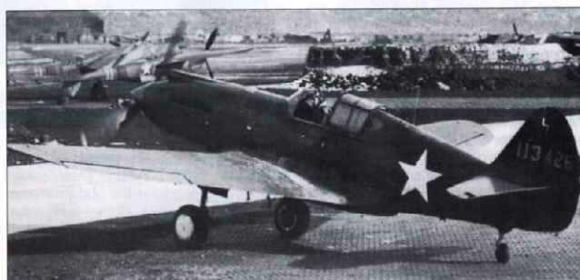
P-40C 41-13426 of the 33rd FS, 8th FG, was based in Iceland circa late 1941. Note the Radio Call Number across the fin and rudder, introduced in October 1941, probably in Identification Yellow 48, and the overpainted red centre to the star and disc national marking on the fuselage.
