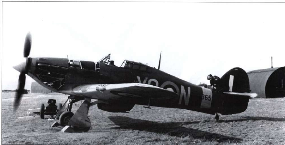
Above: Hurricane Mk IIB Z3658 YO-N was photographed undergoing a maintenance run-up on 24 July 1941. The location is thought to be RAF Digby. The white chalk marks on the fuselage and on the cowling panel on the ground are comments made by the groundcrew indicating various aircraft systems are ok.
