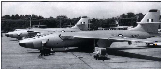
Above: WZ405 was a Valiant B(PR)K.Mk 1. These aircraft were outwardly generally similar to the standard B(K).Mk 1, except in the area of the bomb bay, where a number of windows allowed palletised cameras to 'look out'. (Via Glenn Sands)
