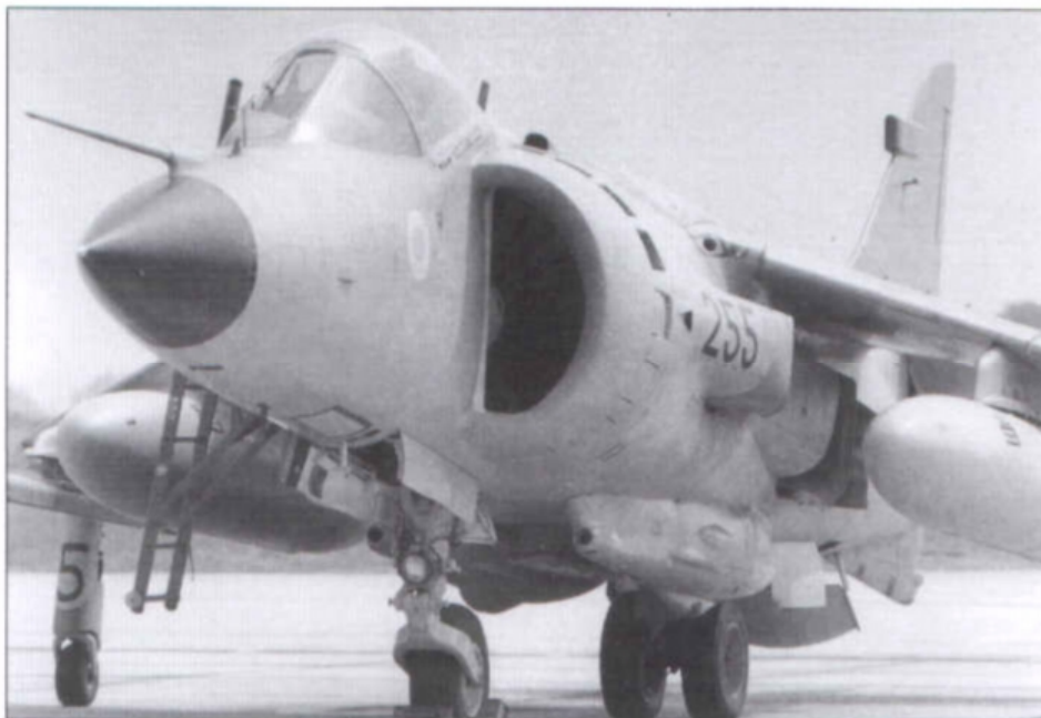
Left: Sea Harrier FRS.1, XZ499/255 of 809 NAS, at Yeovilton in July 1982. Note the detail of the 30mm ADEN gun pods and the nose wheel. (Andy Evans)
