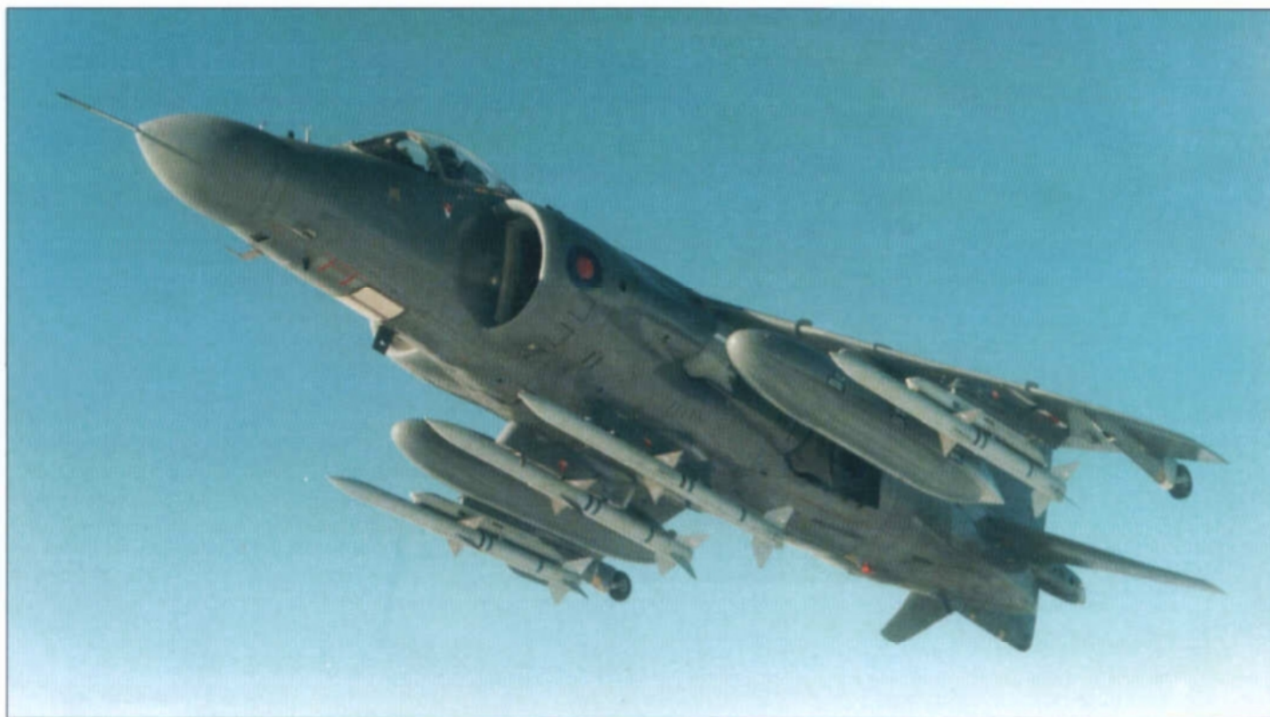
Above: The first development FRS.2, ZA195, carrying four AIM-120B AMRAAM (Advanced Medium Range Air to Air Missile), all-weather, fire-and-forget system. (BAE)
