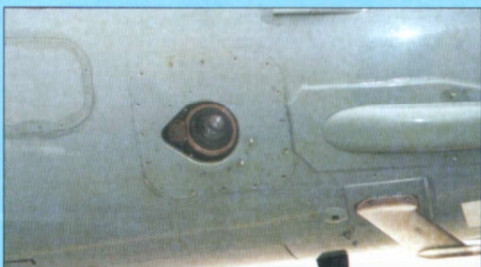
Top: Blue Vixen radar nose radome. Note the additional air scoop. Above: F.95 oblique camera port - note teardrop shape. Below: Air vents below the tail and dielectric panel on fin strake. Above right: Forward 'cold' nozzle and fire access detail Right: Nosewheel gear details Bottom right: Upper nose blade aerial and yaw vanes (All photos Andy Evans)
