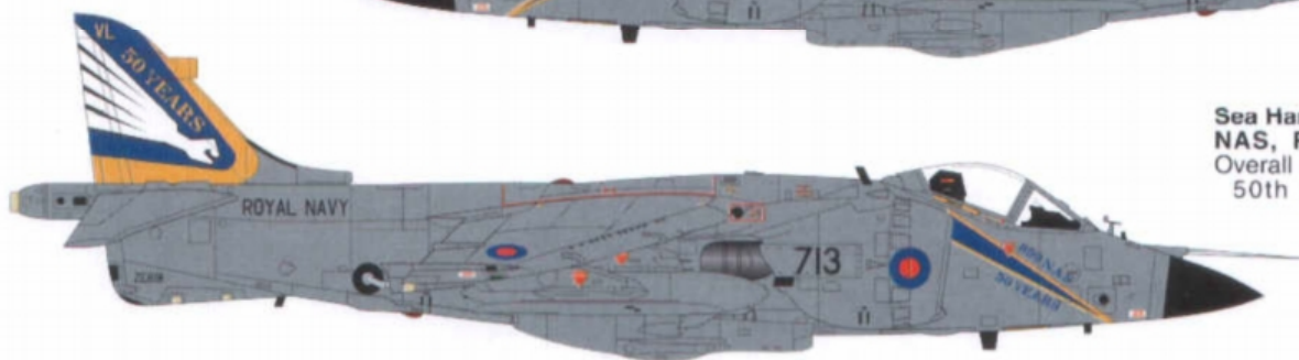
Sea Harrier FRS.2 ZA195, BAE Dunsfold 1988 Prototype FRS.2 aircraft finished in overall Dark Sea Grey. Pitot tube originally fitted to nose. Dummy AMRAAM missiles fitted on later flights.
