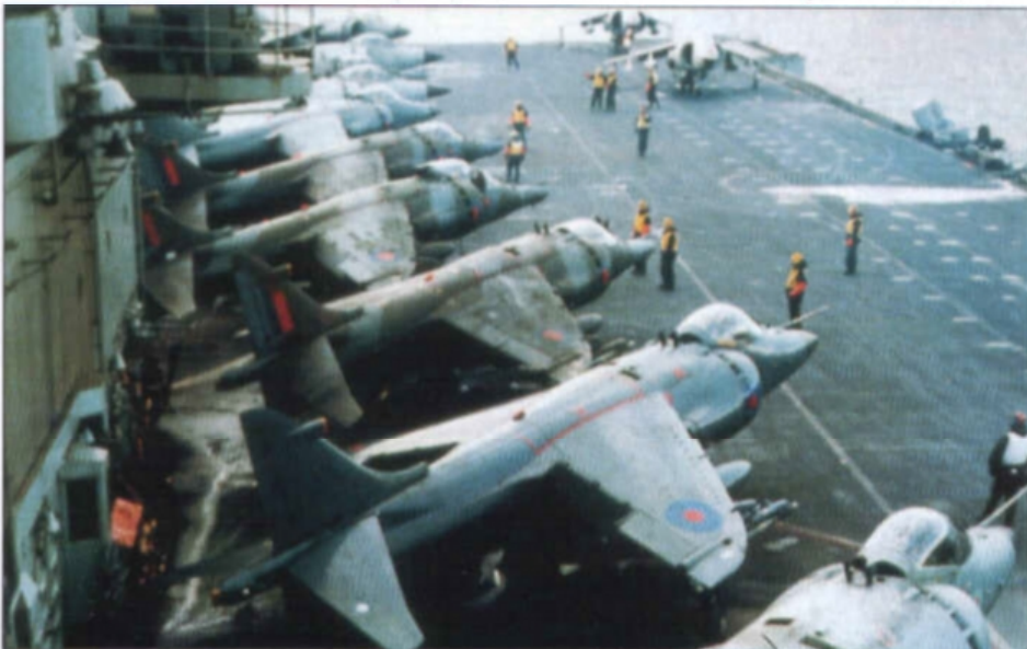
Below: A mix of Sea Harrier FRS.1s and Harrier GR.3s ranged on HMS Hermes' deck, with two CAP armed Sea Harriers waiting to take off in the background. Note the Sea Harrier in the foreground with the damage repair plate on the starboard tailplane. (BAE)
