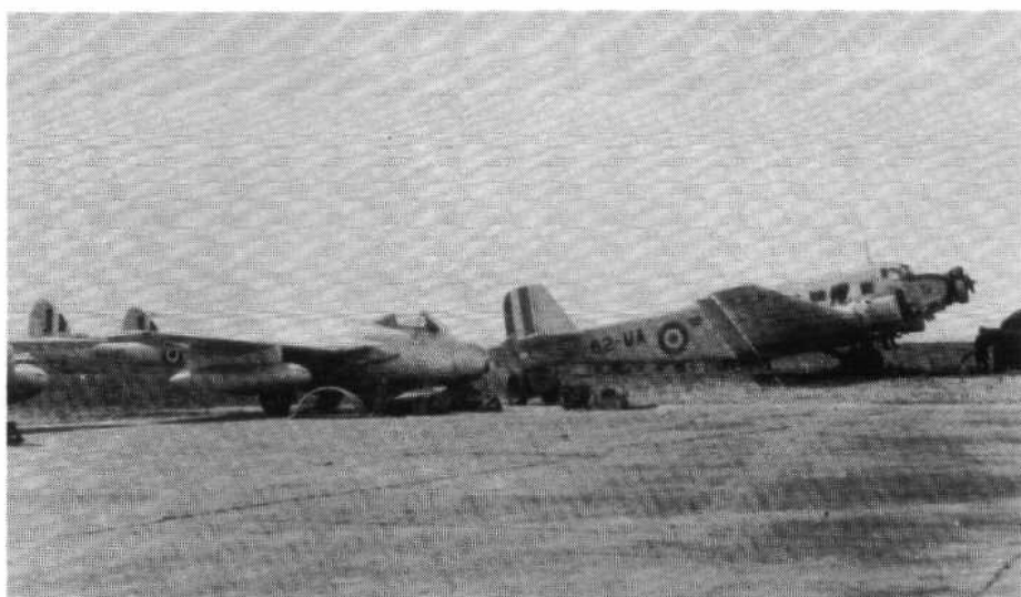
Vampire FB.31 in Royal Australian Air Force service. Most of these aircraft were reworks of earlier F.Mk.30s and were fitted with Rolls-Royce Nene engines.
