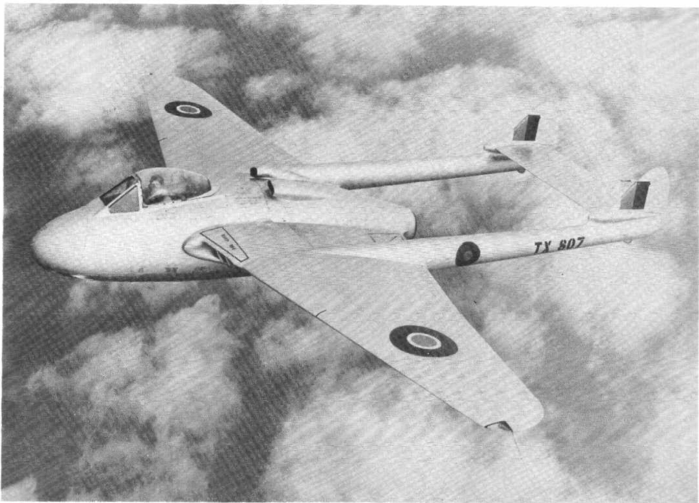
Vampire T.Mk.II TX807 was the first to be fitted with a Rolls-Royce Nene turbojet. The nickname 'elephant ears' has stuck as may be imagined. This aircraft subsequently went to Australia as the prototype for the Mk.30 and Mk.31.
