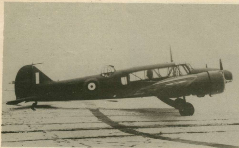
The original Anson Mk.IV was converted to Wright Whirlwind engines in England and then shipped to Canada. Serialled R9816, it is seen in prototype markings at Boscombe Down.
