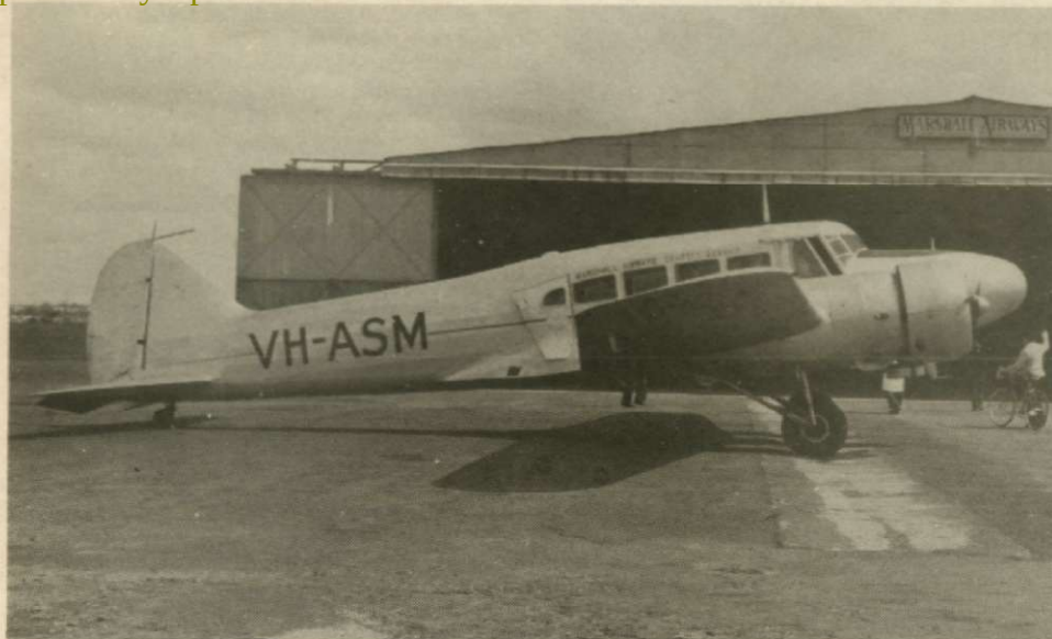
An Australian Anson converted by Marshall Airways into a six-seat passenger transport. (APN)
