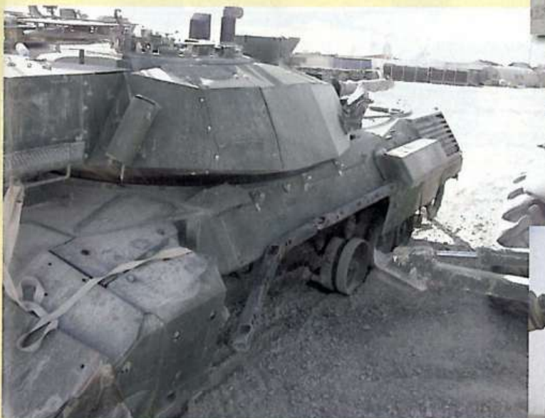
◀ The damage caused to call sign 198 by an anti tank mine strike is clearly visible in this photo taken in June 2007. Damage was caused to the suspension, MEXAS, and the main gun barrel. Note how the MEXAS armour support has become bent and twisted.
