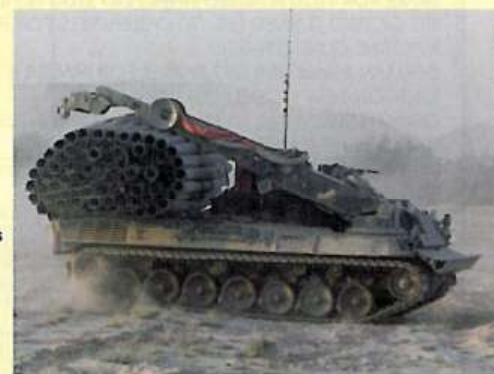
▲ A very unique photo of a Taurus ARV in June 2007 carrying a fascine roll. The crane arm is being used to hold the fascine in place on the back deck. The ability of the crews to adapt to new missions and tactics provided the battle group continual momentum during operations.
