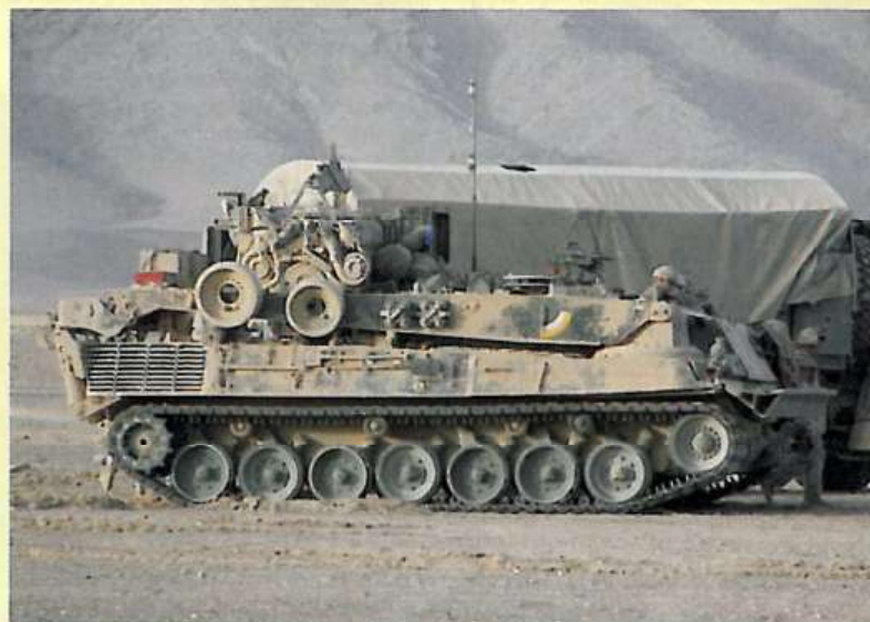
▲ The crew of call sign I1C have just completed changing the left track in July 2007. Note how worn the track pads are on the right track compared to the left side. Clearly visible on the turret is the tan coloured cooling unit and folded combat stretcher strapped to the back of the left turret bin.
