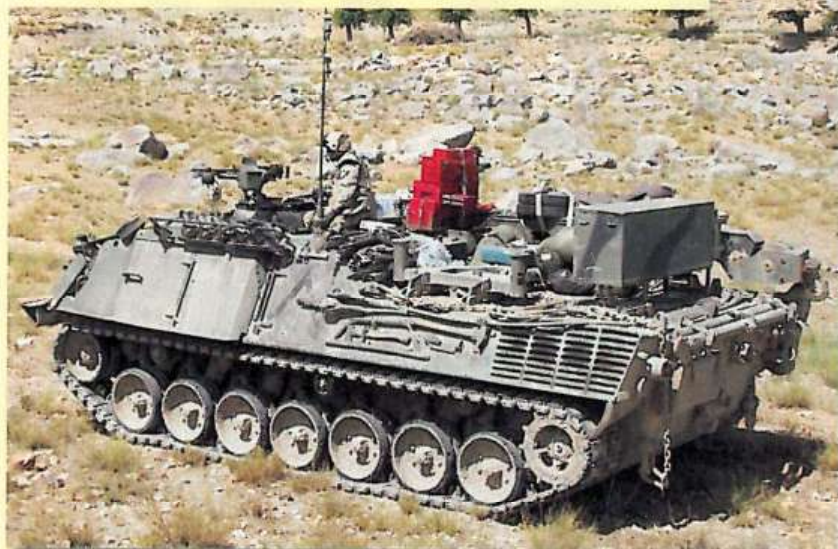
Call sign 18E, a Taurus ARV, in June 2007 in support of the Leopard Squadron during an operation. Visible is the frontal MEXAS armour and a large variety of toolboxes, crew kit, and chains on the back deck.
