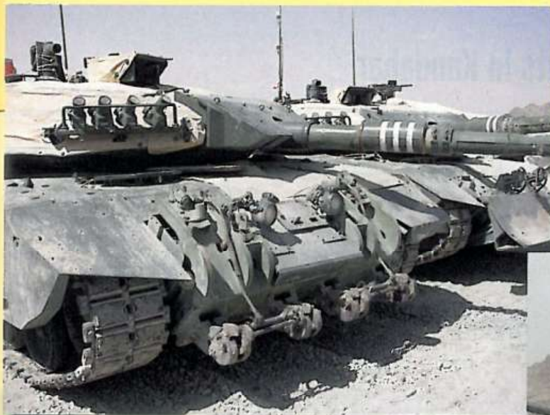
◀ Call sign 13A in August 2007 mounting the mine roller attachments and the thermal cooling blanket. Note that additional armour has been mounted between the headlights on the mine roller attachment.
