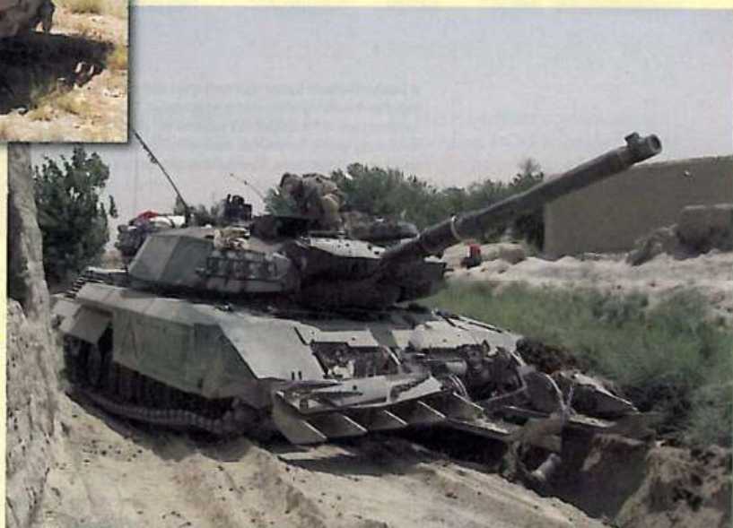
Call sign 11C mounting a mine plough sits idle while temporarily disabled by a thrown right track during a clearing operation in a village in May 2007.
