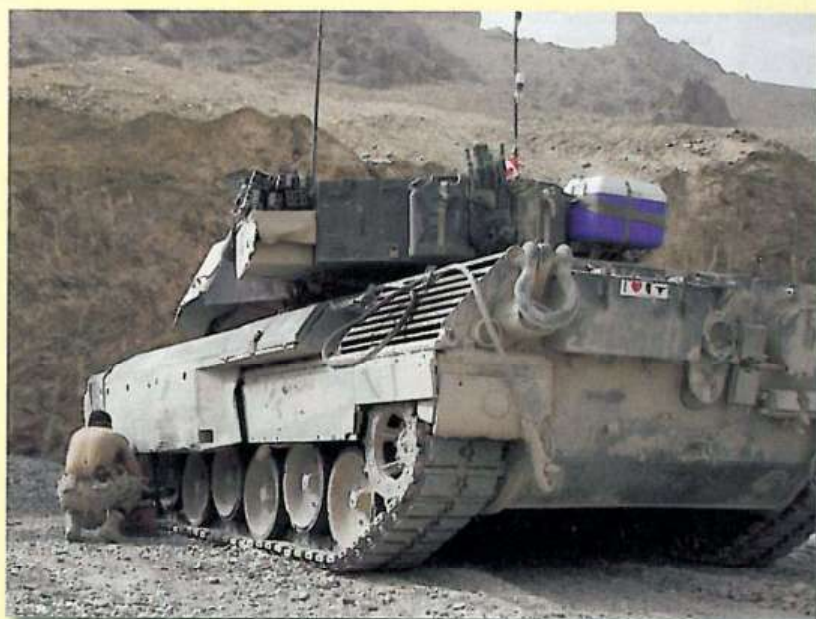
Call sign 12B's crew attend to the road wheels at a Forward Operating Base. The tan painted box mounted on the left side of the turret storage bins contains the cooling unit for the crew cooling system. This cooling unit box was damaged after the tank was backed into a house during an operation. Note the collapsible combat stretcher stowed between the jerry cans and the blue civilian pattern cooler.
