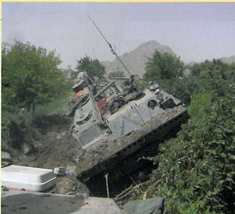
▲ A Taurus ARV sits in a very awkward position during a recovery operation. The Taurus is carrying a bank of mine rollers on the back deck.
