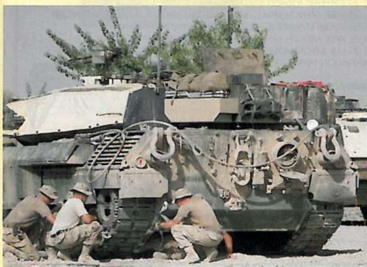
▲ The crew of call sign I1C have just completed changing the left track in July 2007. Note how worn the track pads are on the right track compared to the left side. Clearly visible on the turret is the tan coloured cooling unit and folded combat stretcher strapped to the back of the left turret bin.
