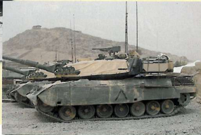
◀ Call sign 13A in August 2007 mounting the mine roller attachments and the thermal cooling blanket. Note that additional armour has been mounted between the headlights on the mine roller attachment.
