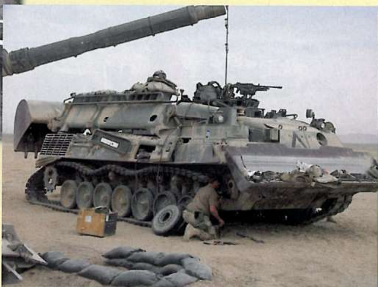
◀ The damage caused to call sign 198 by an anti tank mine strike is clearly visible in this photo taken in June 2007. Damage was caused to the suspension, MEXAS, and the main gun barrel. Note how the MEXAS armour support has become bent and twisted.
