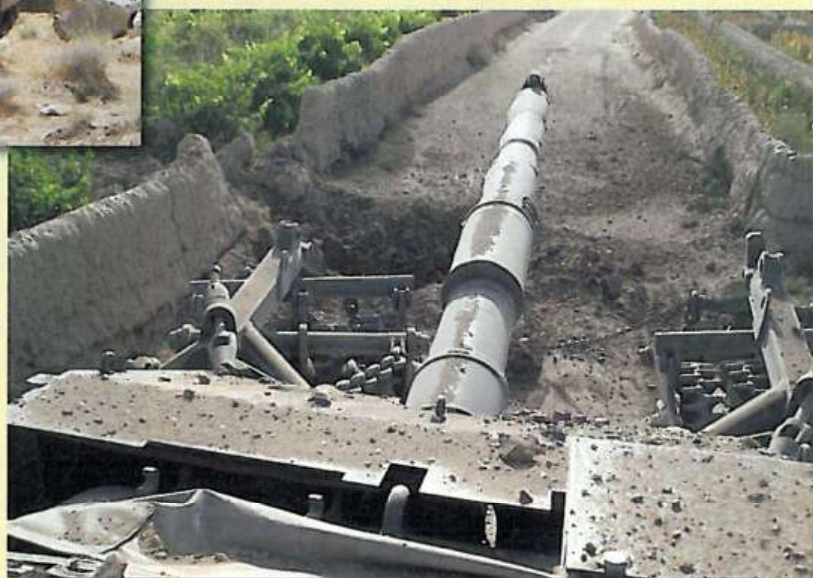
▶ A crew member's view from the turret of a mine roller mounting Leopard C1 after detonating an anti-tank mine or IED in February 2007. Note the crater and the dirt thrown up on the mine rollers, barrel, and mantlet.
