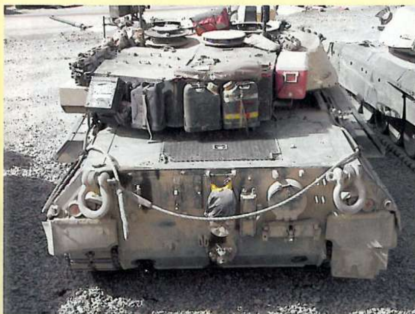
◀ The upper rear deck of call sign 11 while stopped at a Forward Operating Base. Note that the rear hull driver's tool bin has been ripped off and the variety of kit carried on the turret. This tank had an IED strike on August 5, 2007 and sustained minor damage but no injuries to the crew.
