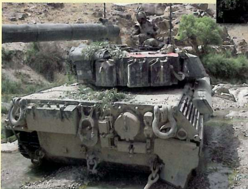
◀ Call sign 12A prepares to tow a disabled tank on a creek bed. Note the branches on the turret and back deck and the torn off left rear mud flap from travelling through heavy brush. Clearly visible on the turret is the red air recognition panel.
