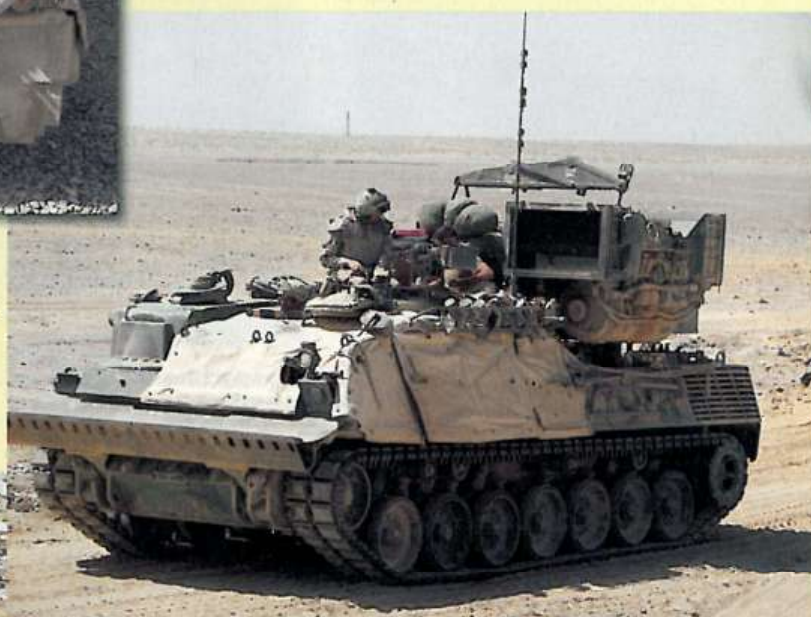
▶ The thermal cooling blanket covered Taurus ARV, call sign 1BE, is seen following up the tank Squadron in August 2007. Attached to the rear deck is a complete Leopard I power pack. The Taurus has a C6 machine gun in a ball mount on the left front and another mounted on the crew commander's hatch ring.
