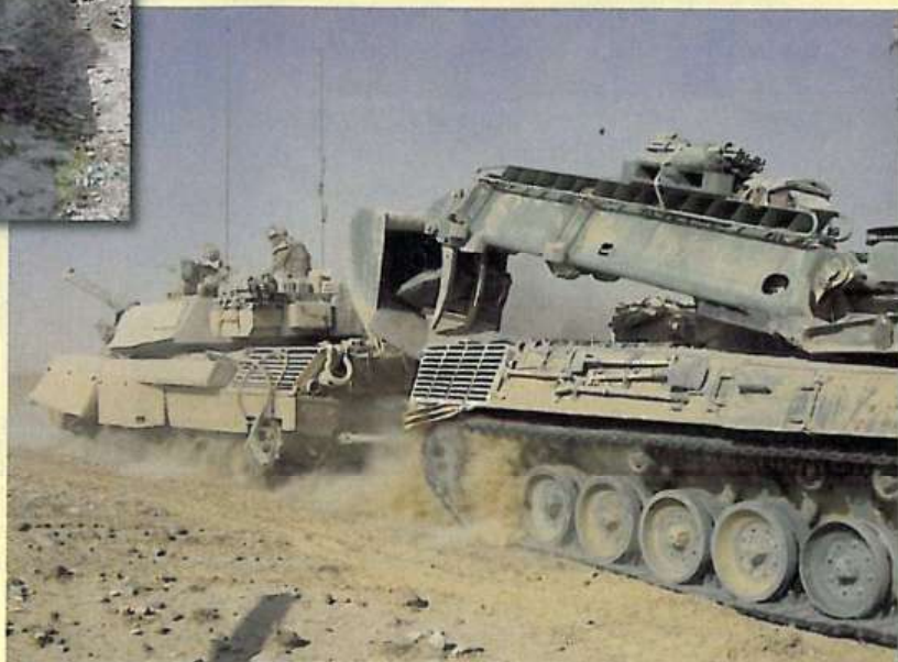
▶ An incredibly dusty damaged Leopard C2 is towed by a Badger AEV. Note that the Leopard is missing the complete left track and the damaged appearance of the left side MEXAS modules. This photo was taken in July 2007 and clearly visible is the cooling unit mounted on the left side of the turret stowage bin. Note also the tyres missing from one of the Badger's road wheels.
