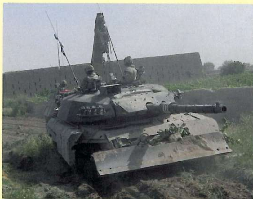
◀ A Taurus ARV recovers call sign 13B, a dozer tank, after damaging the right track. Note that the right front MEXAS modules are missing and the glacis plate is strewn with debris.
