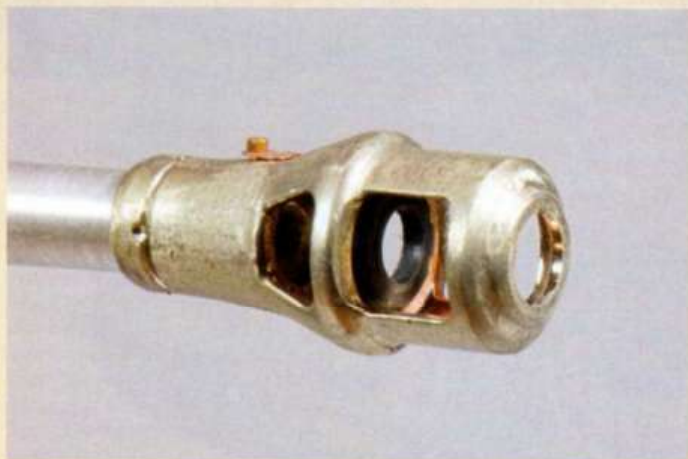
The muzzle brake supplied in the kit has been cast from brass. Note the tiny locking tab and retaining bolt, which prevents the muzzle from being unscrewed from the barrel.
