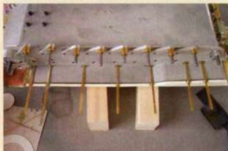
The lower hull has been constructed from aluminium. At this point the torsion bars and suspension arms were installed. Note also the brass strips which will form the skirt armour hangers.
