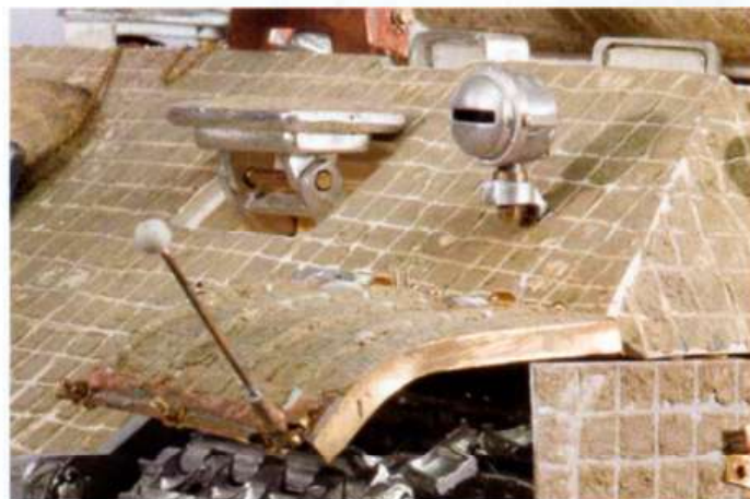
The width indicators were scratch built using brass wire and tube. The ball on the end was fashioned from Magic Sculpt. The fender was constructed from copper sheet, brass strips and thin plastic card.
