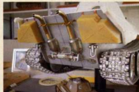
To form the brass tube into the correct shape, the author filled them with sand before bending, which prevents kinks appearing in the bent section. Note the tiny 1:35 Panther at the bottom of the picture!
