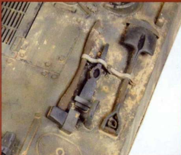
The pioneer tools received new etched brass holders and tie-downs complete with a lead foil securing strap, which the author had to delicately thread through the tiny tie-downs!
