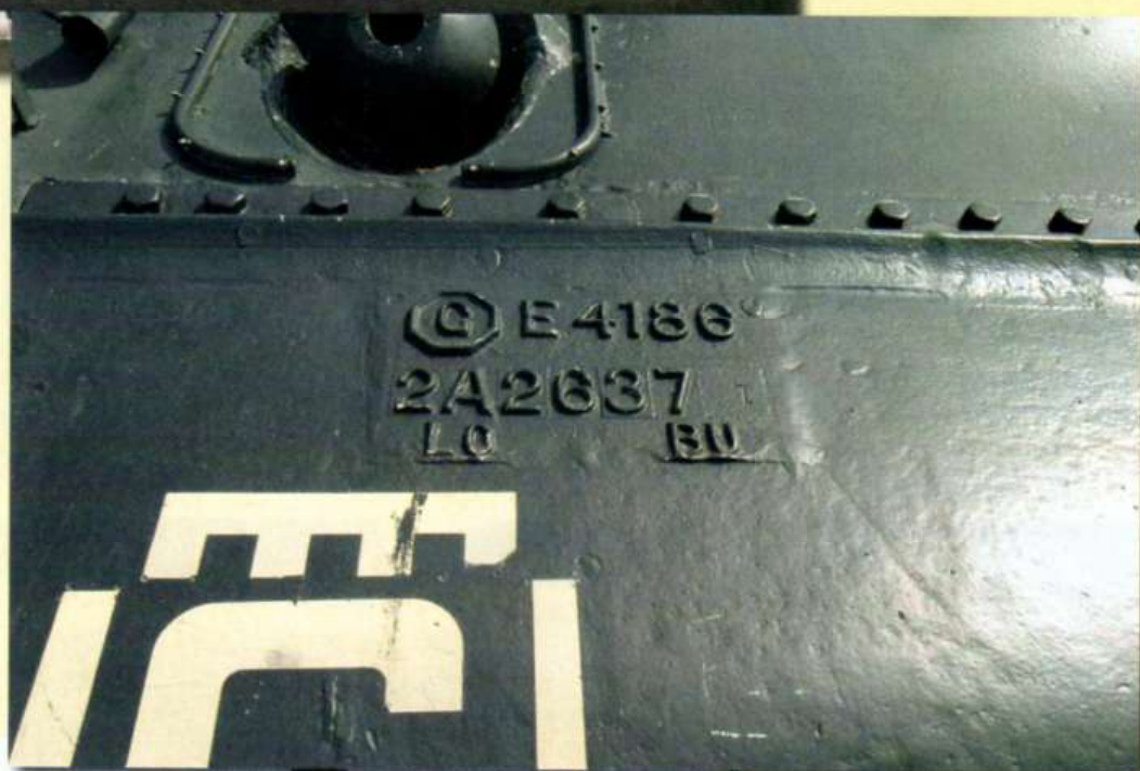
▶ This transmission was produced by the American Foundries, Granite City plant. Note the popper studs used for attaching the waterproof cover over the bow machine-gun housing.
