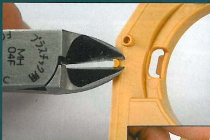
The turret halves are attached to the sprue in a slightly different way to the other parts. Once the component has been removed, a small tab is left on the mating surfaces, and again the side cutters are used here, followed by some careful sanding with a fine grade sanding stick.
