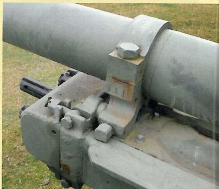
▲ The barrel 'strap' is a hefty item and is fixed securely to the cradle with a large bolt. Note the two small adjusters immediately behind the strap.
