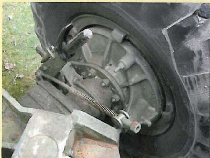
▲ Detail shot of one of the hand brake mechanism. The spring and nut assembly in the foreground is the brake adjuster used to take up any slack as the brake shoes wear down with use.
