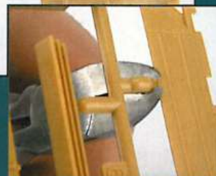
As a tip for anyone new to the hobby, when using sidecutters make sure the flush side of the cutters is nearest the kit part. This way the cut will be nice and neat with very little sanding required to remove any excess sprue gate. The photo to the right is the wrong way to cut.
