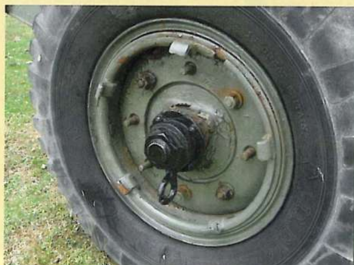
▲ Wheel details. Note that four of the retaining nuts are missing from this wheel. The loop below the central nut is used to tie-down the gun when being transported by rail or sea etc.
