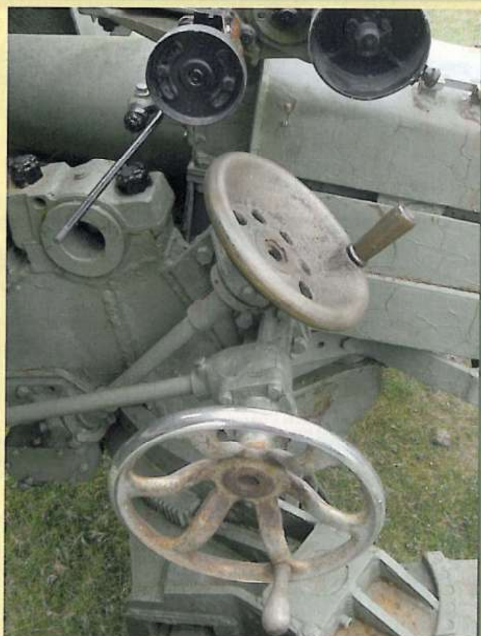
▲ Close-up of the gunner's traverse and elevation wheels. On vehicle mounted 17 pounder guns, the lower wheel is fitted with an electrical firing button in the centre of the handle.
