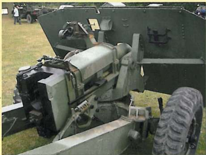
▲ A clear view of the gun shield showing the various metal fittings, braces and rivet detail. The shield not only protected the crew from small arms fire, but also limited the effect of the muzzle blast.
