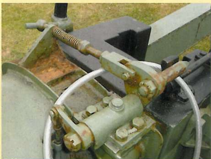
▲ These components make up the mechanical linkage from the gunner's trigger to the firing pin at the rear of the breach. The silver coloured locking cable is not standard WW2 equipment!
