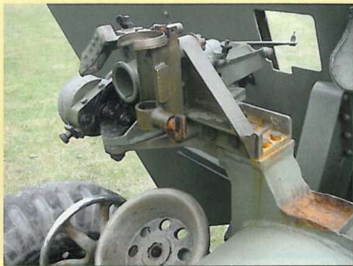
▲ Gunner's sight unit mountings - unfortunately the actual sights are missing.
