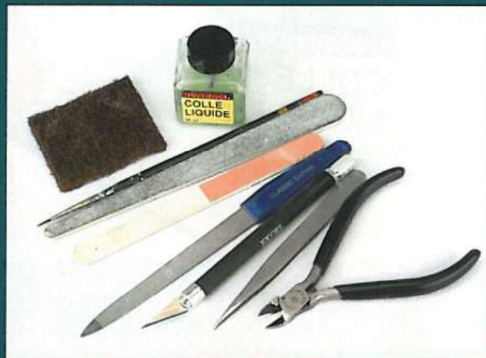
Apart from a tube of instant adhesive for attaching the plastic roadwheels to the metal lower hull, these are all the tools needed to build the Crusader: a couple of sanding sticks, a file, a piece of Scotch Brite, tweezers and a good quality pair of side cutters and craft knife.
