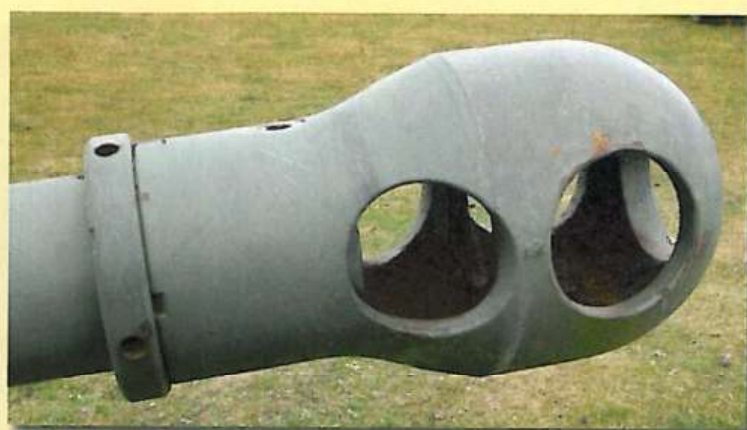
▲ The distinctive muzzle brake of the 17 pounder is sometimes incorrectly shaped in aftermarket gun barrels for models.
