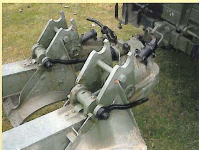
▲ The thick gauge of steel used on the trail leg uprights of clear to see here. In use, these areas would quickly become chipped and scraped, with an accumulation of dust and mud.
