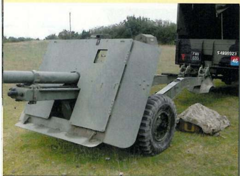
▲ The 17 pounder shield features spaced armour and a drop-down lower shield as used on the German Pak 40 75mm anti-tank gun.
