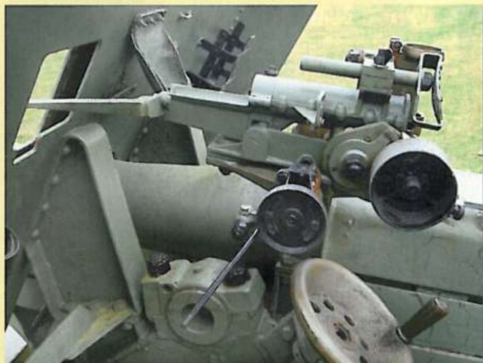
▲ The gun sight mount is seen here, with bronze gun control wheel at the bottom of the shot. The smaller black painted wheels are for adjusting the gun sight.
