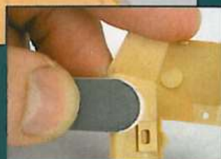
The turret halves are attached to the sprue in a slightly different way to the other parts. Once the component has been removed, a small tab is left on the mating surfaces, and again the side cutters are used here, followed by some careful sanding with a fine grade sanding stick.
