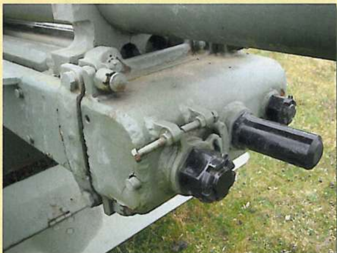
▲ The end cap of the recuperator can be observed here, complete with a multitude of small fittings and adjusters. Of note is the texture on the cap's shoulder - either a welded seam or a cast steel item.
