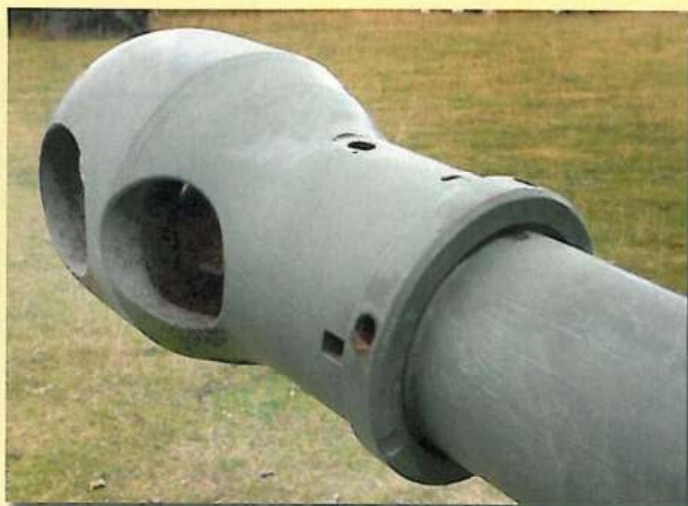
▲ Close-up of the muzzle brake locking ring. In this and the view to the right, the thickness of the metal from which the muzzle brake is made is noteworthy.
