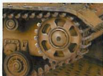
The sprocket teeth have received a metallic sheen where they come in contact with the tracks.
