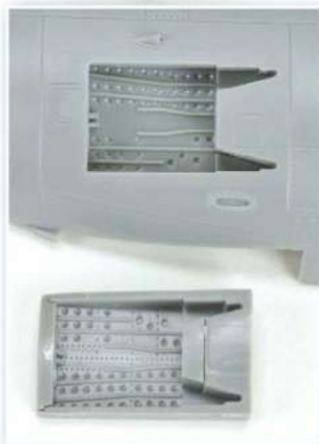
The bays for the air-brake units are separate items that need careful positioning
