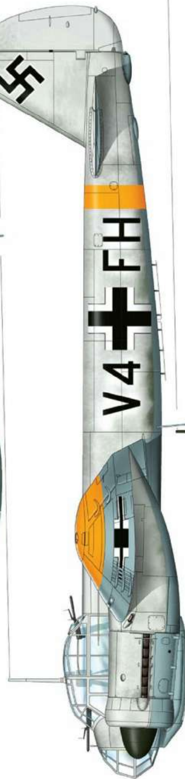
Junkers Ju 88A-4, V4+FH, /NG.I 'Hindenburg' shot down near Dawydecha (Russia), 12 January 1943. Temporary white applied over the upper RLM 70/71; undersides in RLM 65. Codes in black: RLM 04 band around rear fuselage and undersides of wing tips. RLM 70 spinners
