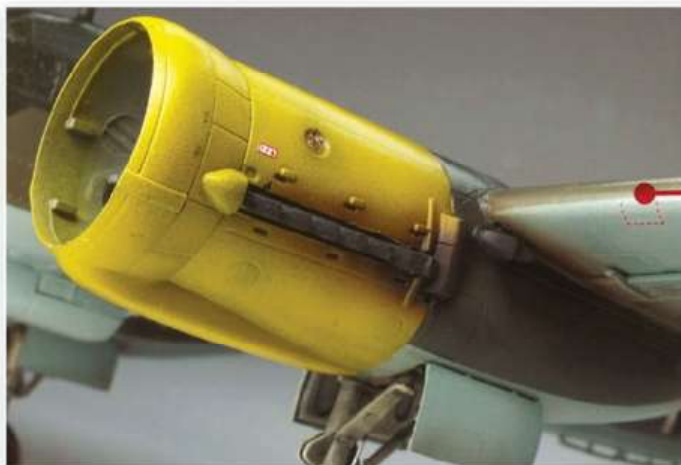
The exhaust stains were sprayed on
