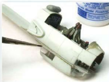
The ventral gondola and windows were bedded in with Kristal Klear
