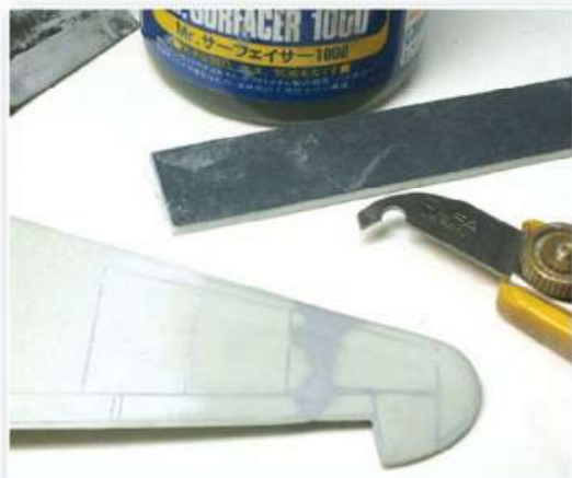
The filled wingtip joint is sprayed with filler, then rescribed
