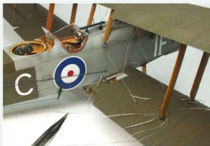
Silver grey and dark grey coloured elastic threads were used for the rigging
