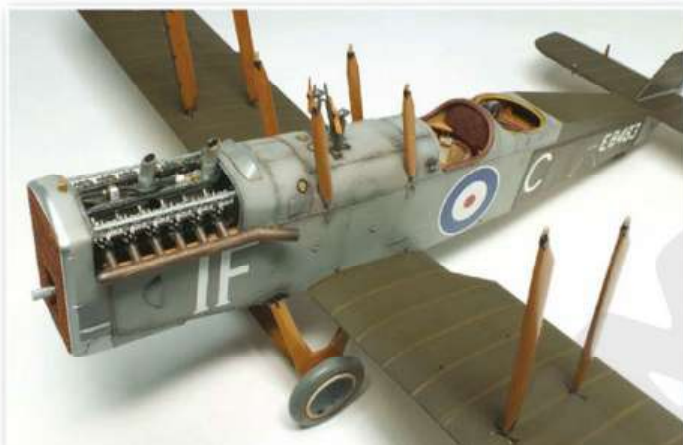
The struts glued in position in readiness for the addition of the top wing
