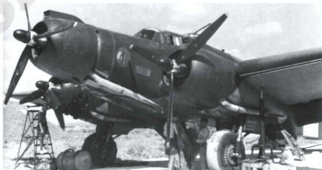
Features that distinguish this SM.84 as a 'bis' variant include the extended flame damping exhaust pipes, larger air intakes above engine cowlings and completely revised cabin framing. A uniform Verde Oliva Scuro2 on all upper surfaces replaces the previous three-tone camouflage (R.J. Caruana Archives)
