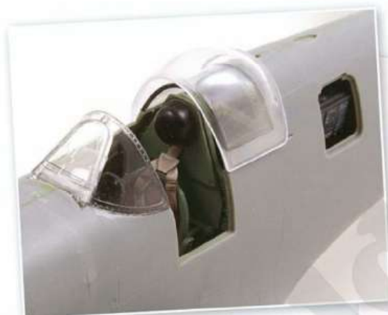
This angle shows off the revised shape in front of the windscreen and also the windscreen with the large separate inner armoured glass
