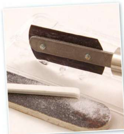
Removing clear parts is best achieved with a very thin razor saw, any rough edges are sanded smooth and polished before the item is installed
