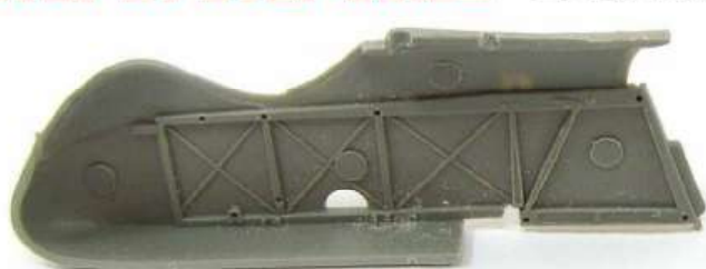
The ejector pins were particularly brutish in the interior
