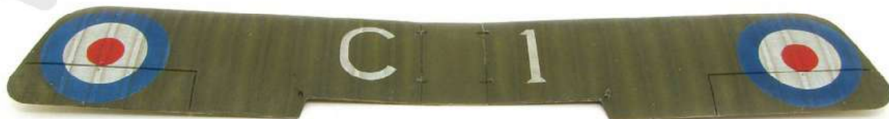
The upper side of the top wing, painting finished. Linen decals have again been toned down by misting the PC 10 mix
