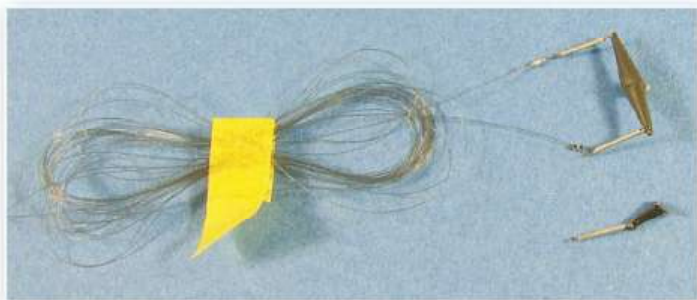
As much as possible, control lines were pre-assembled before they were added to the model
