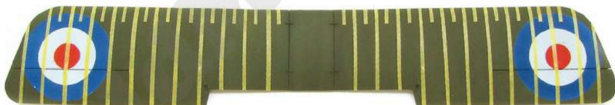
The upper side of the top wing. The PC 10 base coat has been applied and the roundels painted. The ribs have been masked for post-shading
