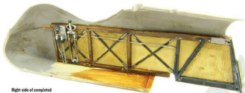
Closed nacelle with stitching and forward sheet metal details replaced with sheet stock
