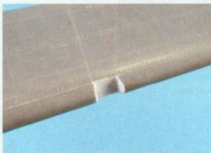
The landing light is in the port wing leading edge only, for all the options in the kit, and here you can see the area boxed off with plasticard
