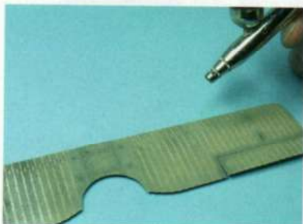
The next stage is to apply light passes of the thinned final colour
