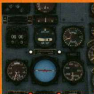
In this close-up of the centre of the panel you can see the PIK/13 master compass indicator, as well as the ZVF-FF cannon round counter, artificial horizon, turn and bank indicator, vertical speed indicator and airspeed indicator
