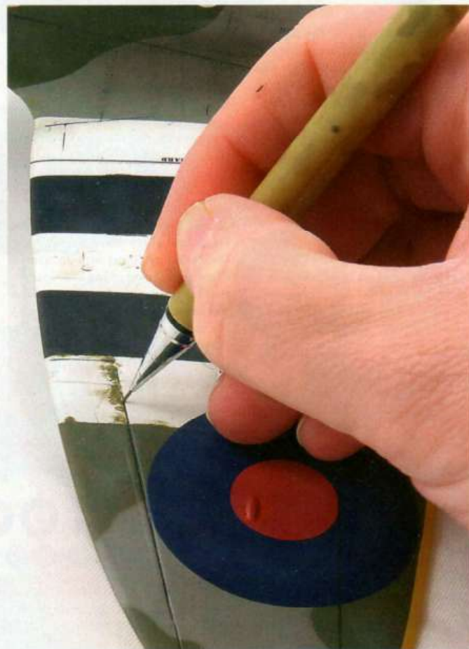
Final weathering was achieved with the aid of a 2B lead pencil which helps to accentuate things like hinge lines. This final finish will need some varnish over the top in order to take out the shine of the graphite
