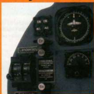
On the left side of the panel are the propeller pitch control switches, undercarriage position indicator and control handles plus the compressed air pressure gauge
