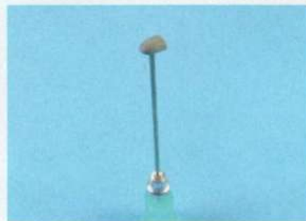
The upper front decking lacks the two prominent air scoops in this area, so a mould was carved from plastic stock...
