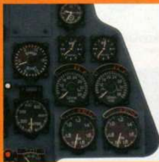
On the right side of the panel are the pairs of engine RPM indicators, pressure gauges and propeller pitch indicators along with the clock and magnetic compass
