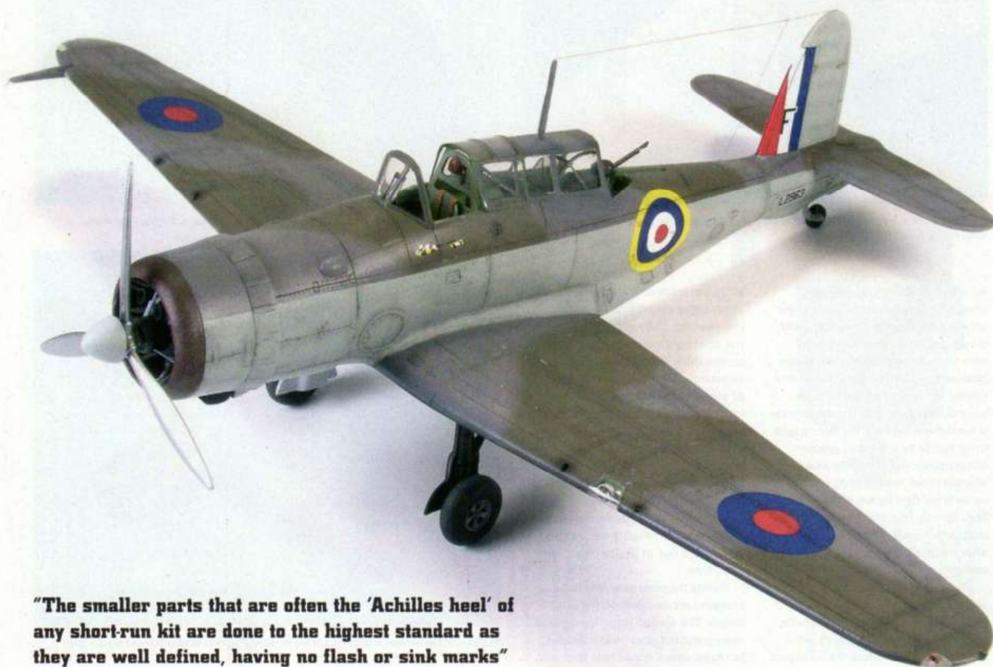
The completed model with the canopies masked ready for paint. Note the scoops added to the upper decking, the boxed-in landing light and the cowl straps reproduced with strips of plasticard to replace those removed by sanding
