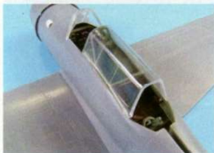
The canopy was chopped up and the windscreen and mid-section secured in position
