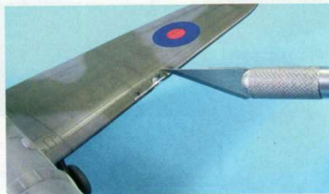
The landing light was glazed with clear adhesive tape carefully trimmed with a new blade in the knife
