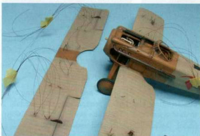
All the rigging tied in position
