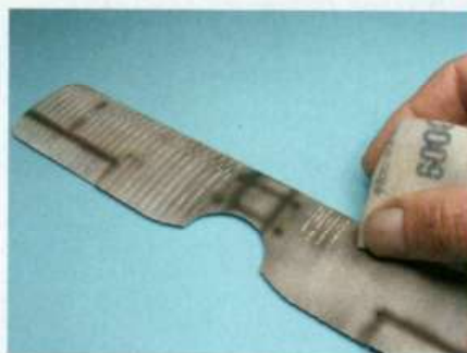
The ribs on the wings are rubbed down after the NATO Black has been applied
