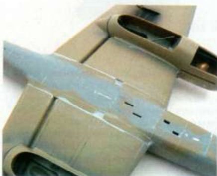
There is a step on the wing join that was reduced using filler. The fuselage inserts are a good fit but are quite fiddly to get into place without getting steps or gaps
