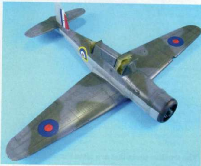
The paint and decals complete; as you can see the camouflage was applied freehand to get a soft demarcation
