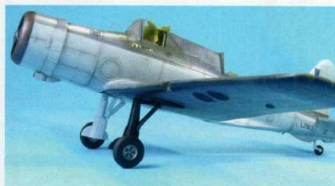
The undercarriage legs are not at 90° to the wing, they slope backwards slightly
