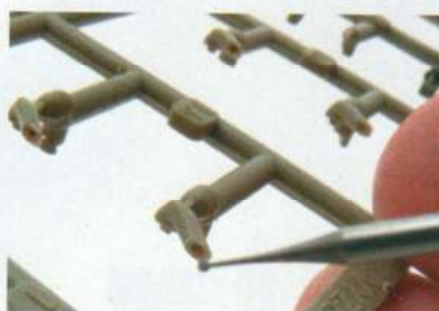
I used the trusty motor tool with an engraving bit to ream out the exhausts. These were a pain to be honest, so you're better off getting the Quickboost set
