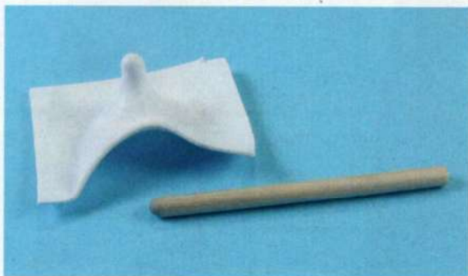
The parabola for the landing light was crash-formed using a profiled stick as the mould
