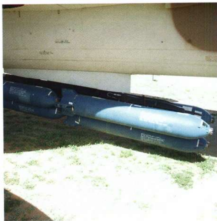
The TER (Triple Ejector Rack) on the centerline position carrying cluster bombs
