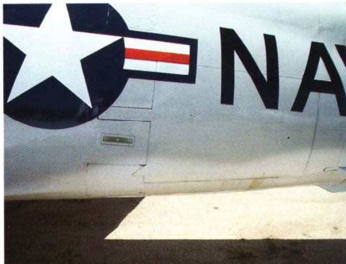
The air brakes on the lower fuselage on the port side, which apply to both -4 and -4B versions
