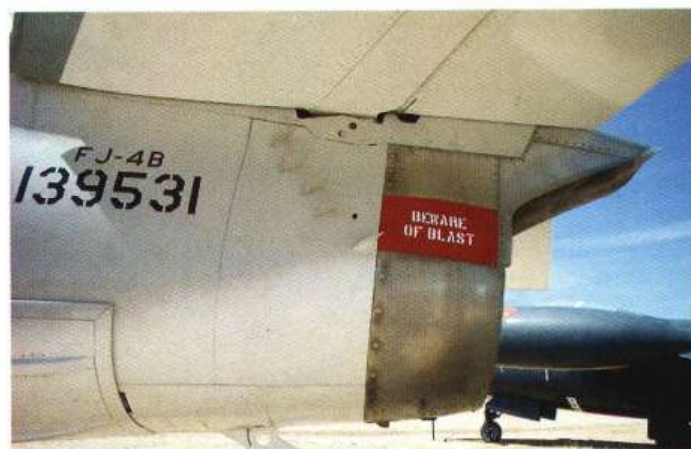
The exhaust outlet with the line of vortex generators forward of it
