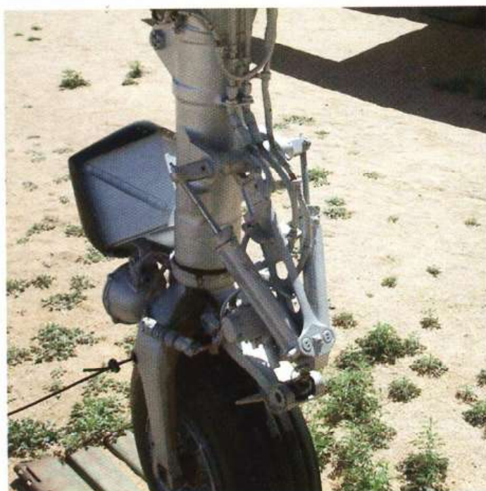
A look at the rather complex linkage at the back of the nose oleo leg. The oleo is fully deflated due to the lack of hydraulic pressure in this preserved example
