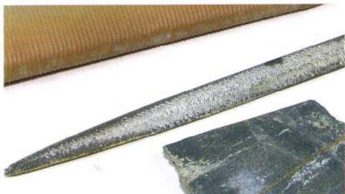
Once the wings were joined they were painted brown an oval file plus wet 'n' dry was used to sand out each corrugation
