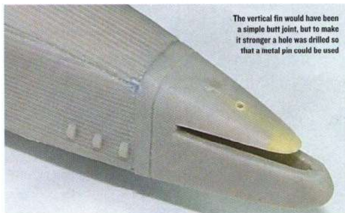
The tail surfaces along with the vertical fin with the mounting pin in position
