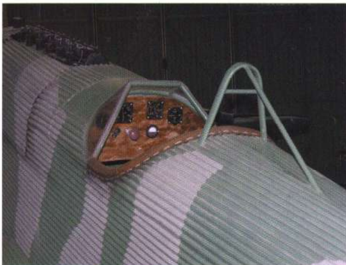
This shot into the cockpit shows the very basic instrument panel; in this replica it is wooden
