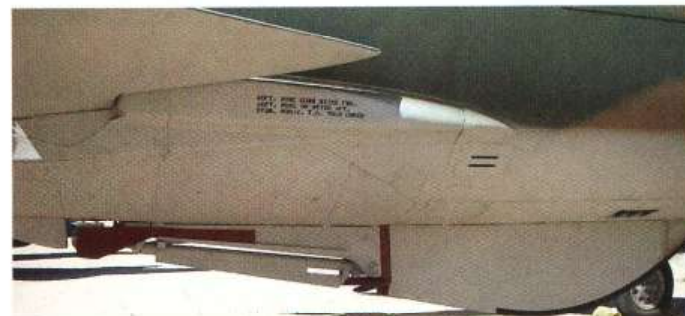
Here you can see the large ventral fin and the airfield emergency arrestor hook behind it
