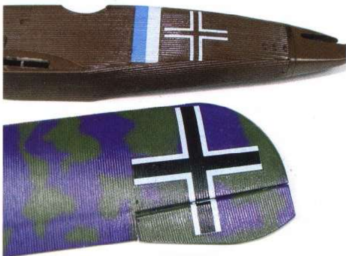
The complex nature of the corrugations meant that the decaling had to be done before everything was assembled; here the markings have been applied to the fuselage and wing
