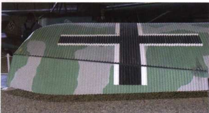
The ailerons, with the crosses painted over wing and aileron. Once again the corrugations on ailerons of this replica match those of the wing
