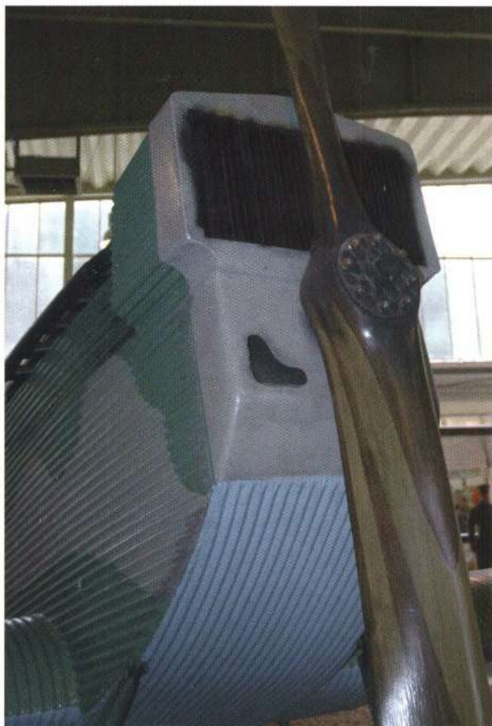
The front cowling with the radiator in the upper section and the two intakes below, note the use of the corrugation edges for the demarcation
