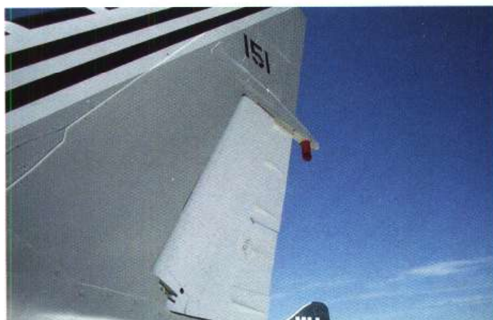
The vertical fin and rudder; the ribbing on the latter is noteworthy
