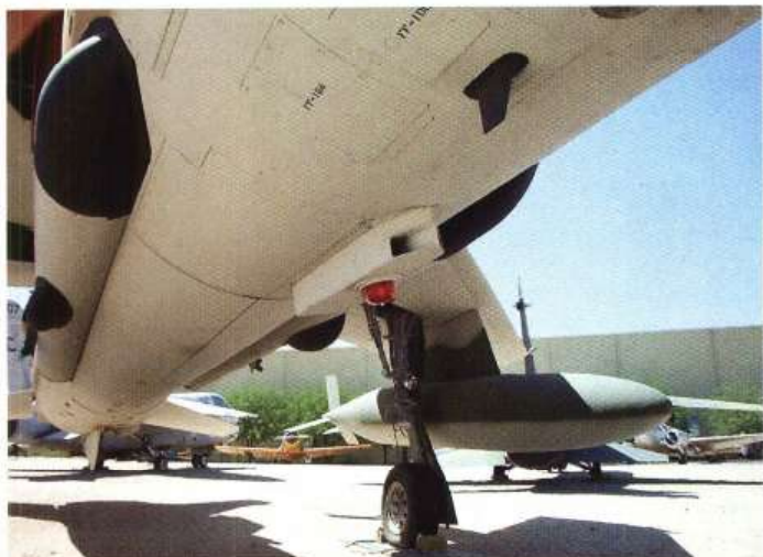
This view on the mid-fuselage underside shows the blade aerial, formation light and anti-collision beacon and the wiring tunnel on the port side
