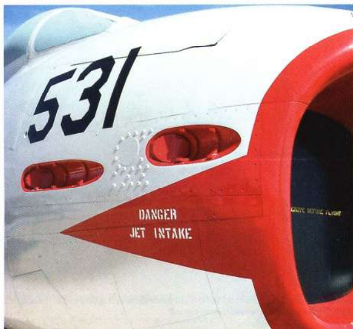
The main gun port, in this instance on the starboard side of the nose
