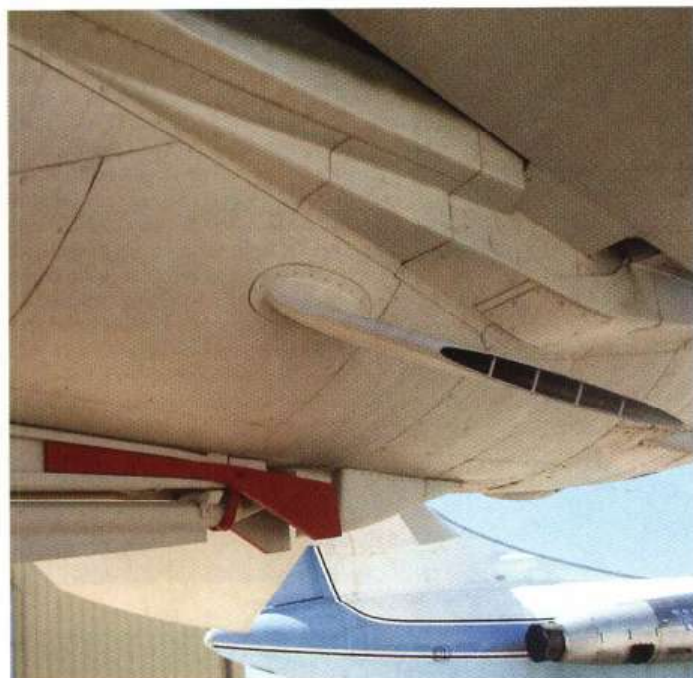
These are the two prominent fuel dumps under the aft rear fuselage
