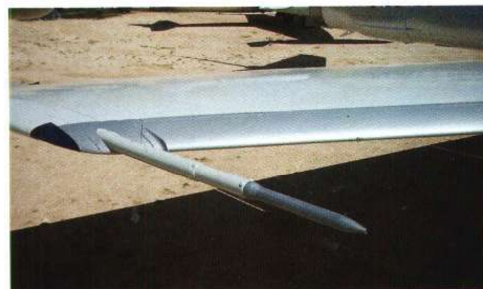
The pitot on the tip of the starboard wing
