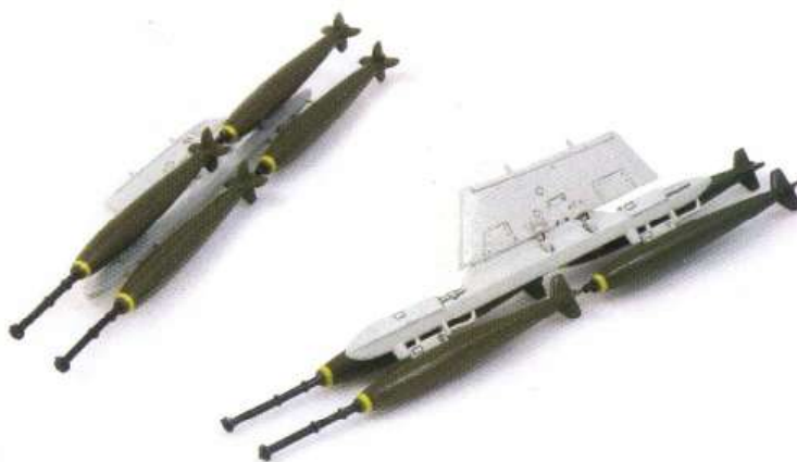
The incorrect MER racks with the Mk 82 (long fuse) bombload
