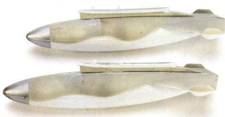
The silver bits, courtesy of the amazing Alclad II metal lacquer. Aluminium shade in this case
