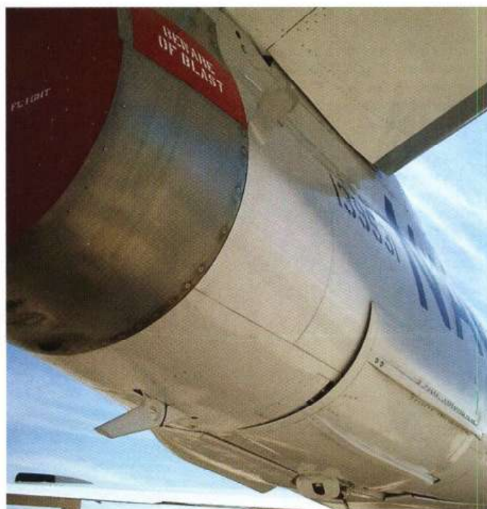
A useful shot under the rear fuselage, showing the ventral airbrakes (-4B only), the arrestor hook and the fuel dump pipe. You can also see into the all-moving tailplane mechanism at its root
