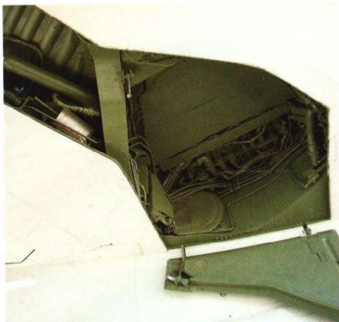
A look into the mainwheel well, this view looking inwards towards the fuselage
