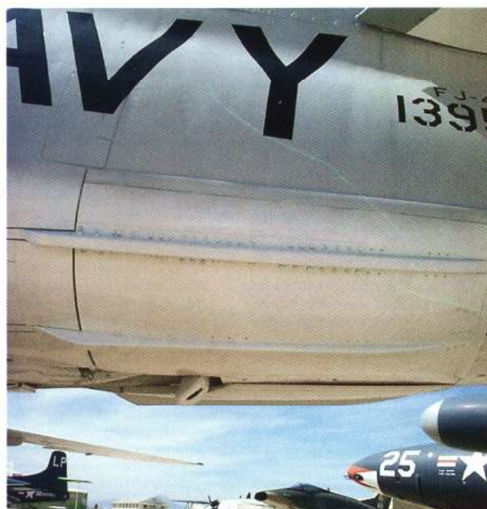
Further aft under the rear fuselage are these additional airbrakes; these apply ONLY to the -4B version
