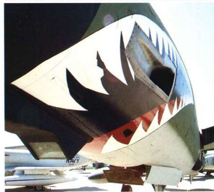
A close-up of the cannon port in the port side of the nose
