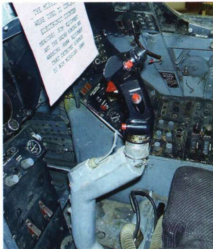
This shot shows the starboard sidewall and the control column
