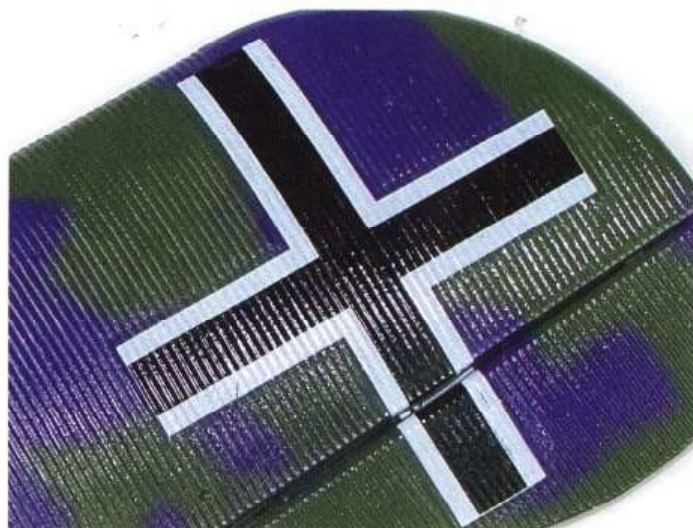
As can be seen, with perseverance the decals will fit into the corrugations
