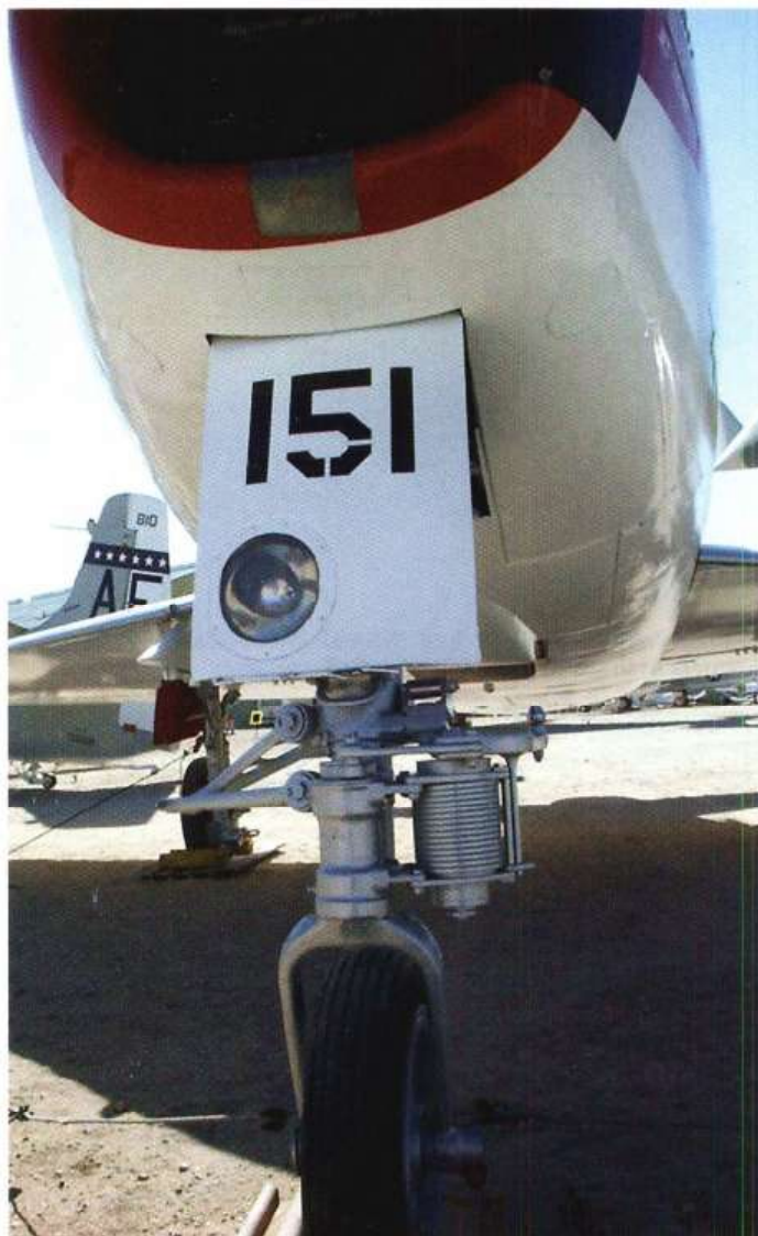
The nosewheel door has the prominent landing light mounted into it
