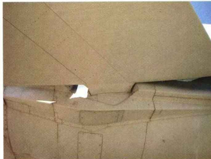
This is the swivel joint for the tailplane, viewed from underneath
