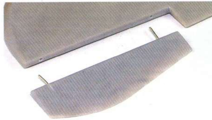
The ailerons were also installed using pins secured into pre-drilled holes
