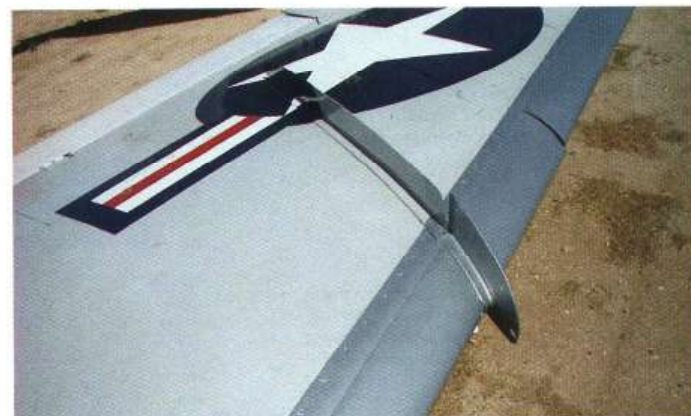
The wing fence, in this instance on the port wing
