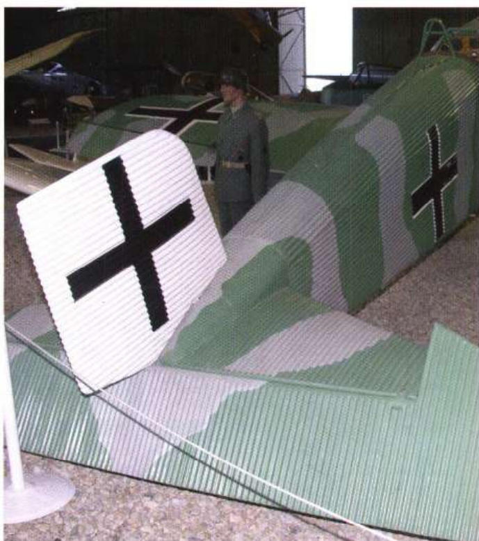
The vertical fin (no rudder) and the elevators, note the flat skinning for the tail cone section. On this replica the corrugations of the elevators match those of the tailplanes
