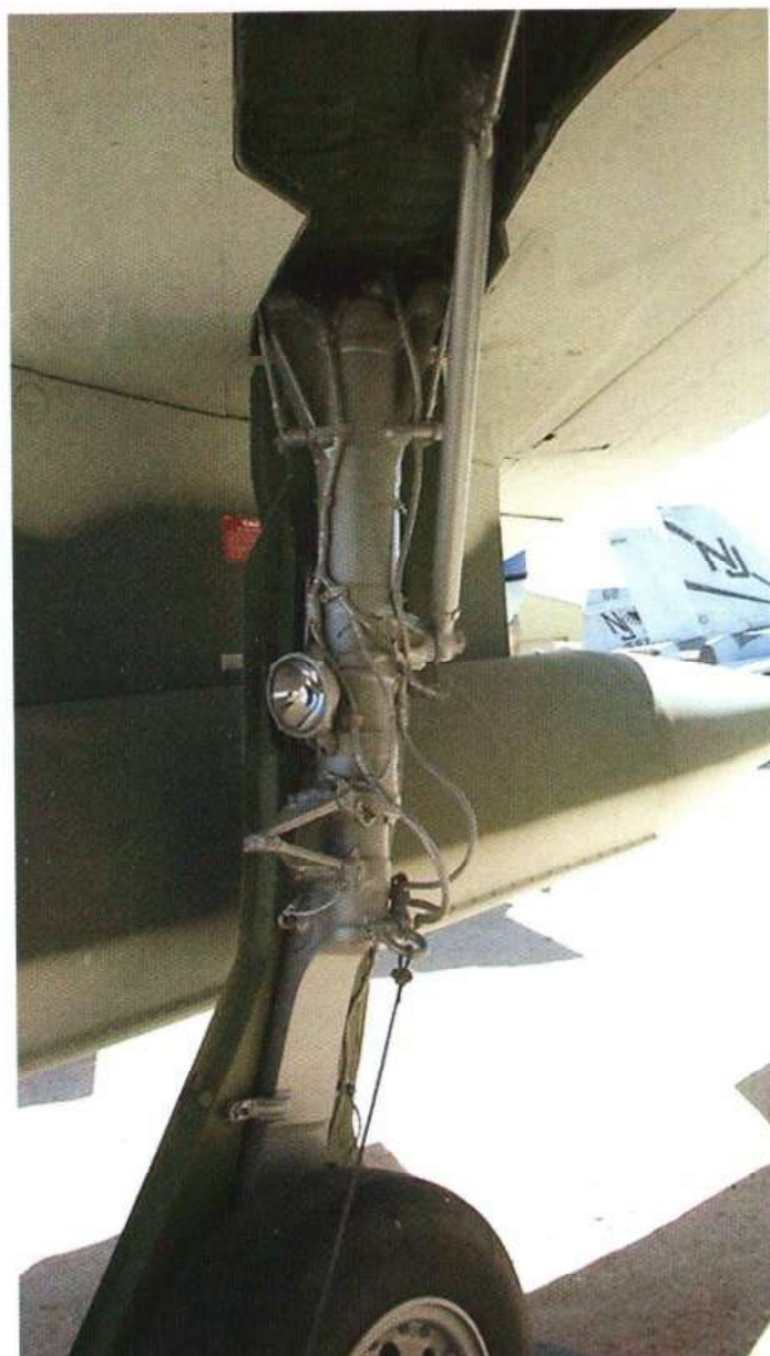
The inner face of the main oleo leg, with all the various hydraulic pipes
