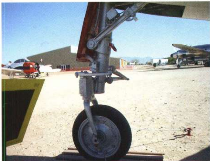
This view of the port side of the nosewheel oleo and wheel shows the various small details in this area omitted from the kit
