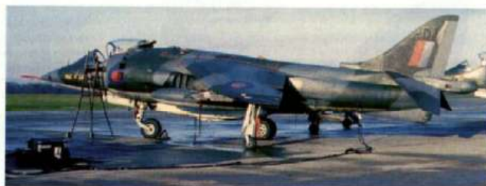
No.4 Squadron Harrier GR Mk 1, XV784/D, photographed on 6th December 1975. It is finished in the intermediate scheme, that is in matt colours but still retaining its Light Aircraft Grey undersides; note how the pattern of the Dark Green on the fin does not continue onto the rudder, ensuring that each detachable part of one aircraft could be fitted onto another without mis-match (Dennis Robinson)
