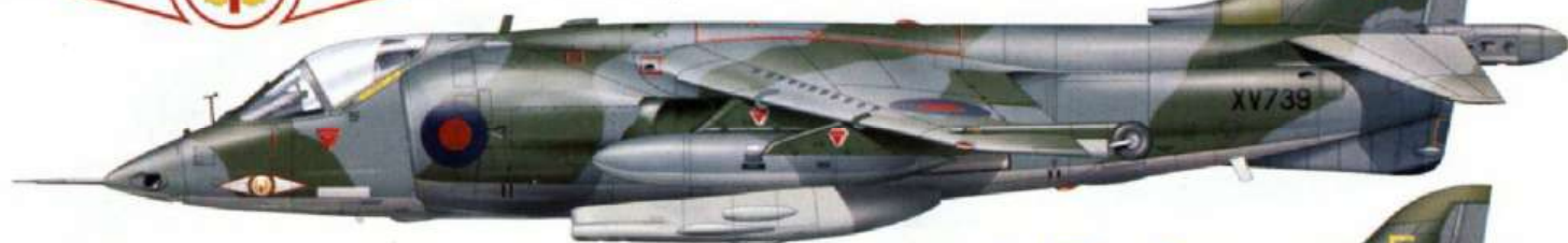
Hawker-Siddeley Harrier GR Mk 1, XW767/F, No.3 Squadron, 1975. Dark Sea Grey/Dark Green/Light Aircraft Grey finish with blue/red national markings; black serial, repeated below wings. Code 'F' in yellow on fin; white nose cap and wingtips; unit badge on nose, flanked by green/yellow bars. When recorded at Malta it carried a No.111 Squadron zap on the rear fuselage.
