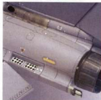
Here you can see the Chaff dispensers on the rear fuselage mentioned by Pierre in this review
