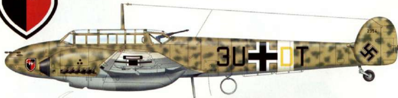
Messerschmitt Bf 110E-2, 3U+KT of 9./ZG 26, North Africa, March 1942. RLM 78/79 scheme with Gelb 27 engine cowlings and rudder. Broad white fuselage band and extreme end of tail. 'K' of code is also in Gelb, outlined in black. Note thin black line on spinner
