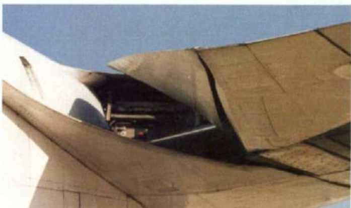
This shot up into the hinge area of the starboard wing illustrates the big hydraulic ram in this area, as well as the droop to the inboard flap
