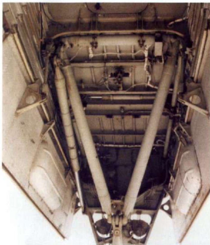
Here is a view of the rear section of the nosewheel well on a current Tu-160 photographed recently at Zhukovsky. The access hatch that comes up in front of the crew's toilet can be seen to the top
