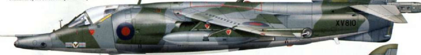
Hawker-Siddeley Harrier GR Mk 3, XV810, No.20 Squadron, 15th October 1976. Dark Sea Grey/Dark Green/Light Aircraft Grey finish with blue/red national markings on intake sides, upper main planes and fin with 36in. red/white/blue roundels under wing. Black serial, repeated below wings. Code XX in black on outrigger fairings. Unit badge on nose, flanked by light blue bars, with red/white/green stripes at centre. Note US Marine Corps style aerial fitted for evaluation by the British Army in Germany
