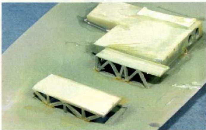
Here are the gun bays viewed from 'inside.' A few blobs of Araldite were placed on the underneath of each gun bay and the top and bottom sections of the wings were then joined using Tamiya Extra Thin Cement.
