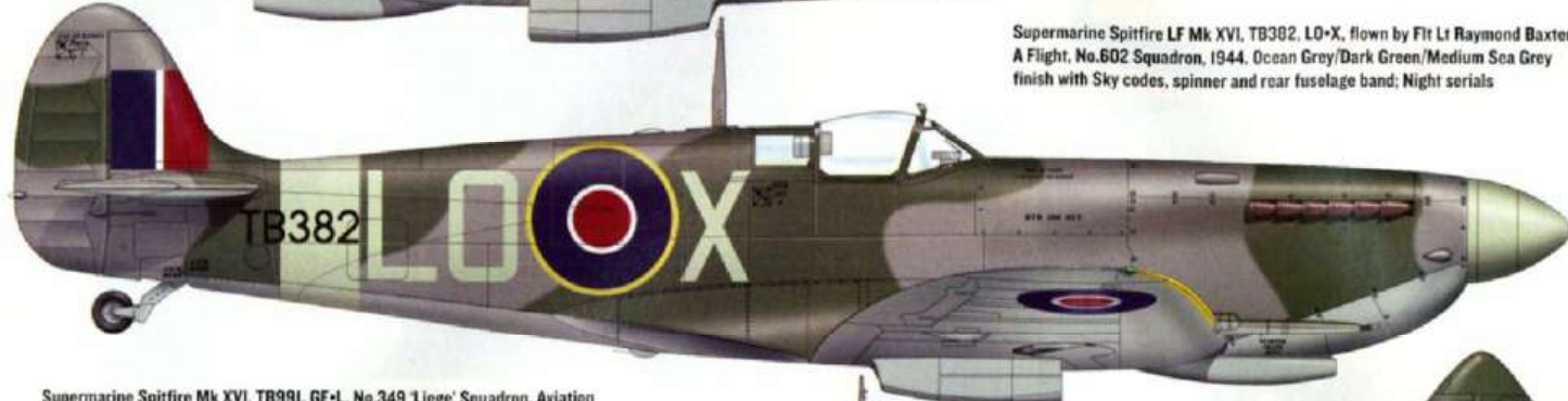
Supermarine Spitfire Mk XVI, TB991, GE-L, No.349 'Liege' Squadron, Aviation Militaire (Belgian Air Force). Ocean Grey/Dark Green/Medium Sea Grey finish with red spinner; Sky codes and Night serial. Roundels in six positions; 'Liege' in white on engine cowlings
