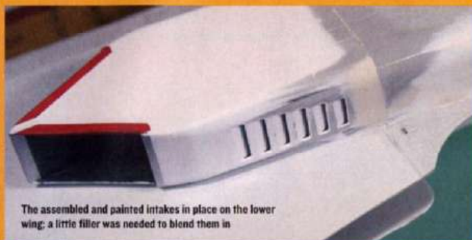
Here the assembled and painted engine intakes can be seen, along with the blow-in doors taped up at the back (inside) to stop overspray when the outer colour is applied to the airframe
