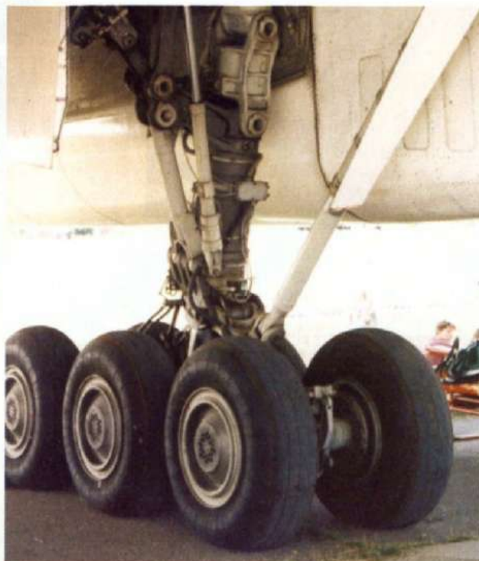
One of the main undercarriage legs, showing that this assembly is not dark grey but dark metallic grey for the main central leg, light silver for the upper section and light grey for all the other struts
