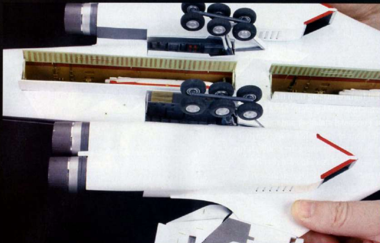
The Tu-160 has two bomb bays and a lot of main wheels! Spend time detailing these areas, as they are some of the only details on this otherwise big white bird!
