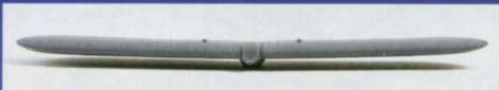
... and after. The central fuel tank prevents the wing being totally flattened and retains just enough dihedral to be accurate
