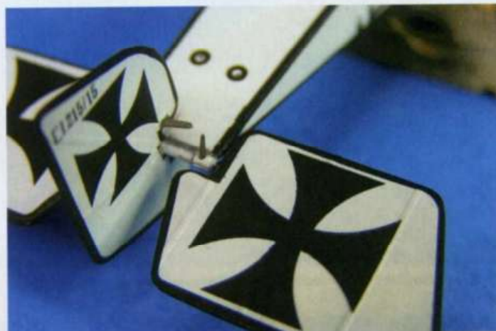
The tail section and control wire horns were all secured with epoxy resin for a no-worries bond
