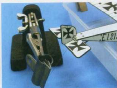
A shortened version of 'Helping Hands' to provide tension at any angle...
