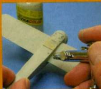
Xtracolor primer provides a good solid base coat and is a lot cheaper than aerosols
