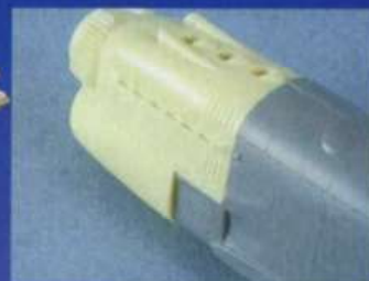
A test fit of the nose after much grinding of the inside fuselage halves. It does require a lot of fiddling but eventually can be made to fit quite well, although some filling and sanding is inevitable
