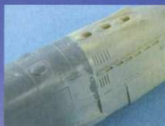
After sanding, priming and more of the same the nose fits smoothly into the fuselage. I've also rescribed the panel lines on the upper cowling where sanding had erased them
