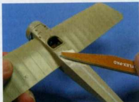
The small step behind the cockpit is sanded, starting with a medium grade sanding stick...
