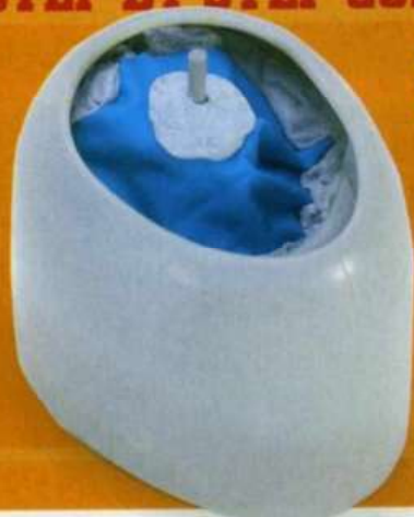
Masked off for painting with a little circle of rubber sheet to keep the Blu-Tack away from the wires, otherwise it would just rip them off
