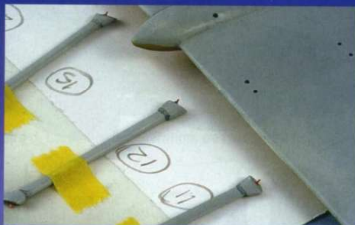
Small holes have been drilled in the wings and tiny wire locators installed at each end of the struts. As the article explains though, it didn't quite work out as planned...
