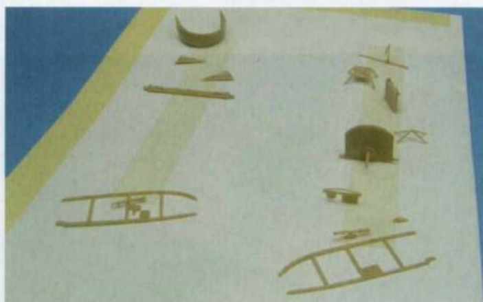
Double-sided tape is useful for holding small parts during painting
