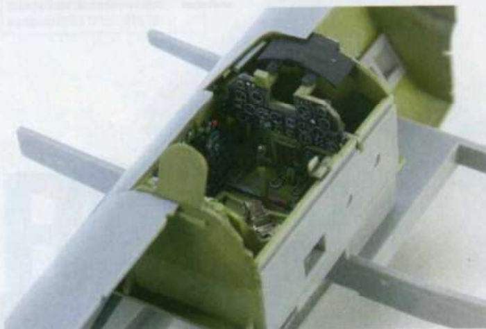
The built-up cockpit and wing spars fit neatly and securely into the fuselage halves; the big wings are going to need the support that the twin-spar arrangement gives it.
