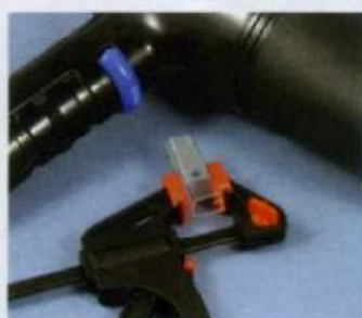
Once folded, the part must be glued and clamped to the transparent part to ensure the correct cross-section. The hair-dryer was used to warm the part while bending, but even so you can see the white lines on the kit part where the plastic is ultra-thin, and in fact it did split in a couple of places
