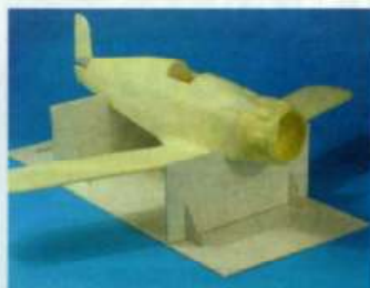
It is simply glued from cut cardboard with profiled cut-outs made for the fuselage or wings
