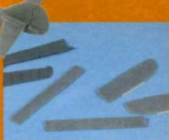
Control surfaces ready to install, after much thinning of the trailing edges. The trim tabs are supplied as photo-etch items, which I chose to replace with thin plasticard
