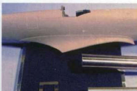
Before the hatch template can be used you need to curve it using something like the Roll Assist from the Small Shop
