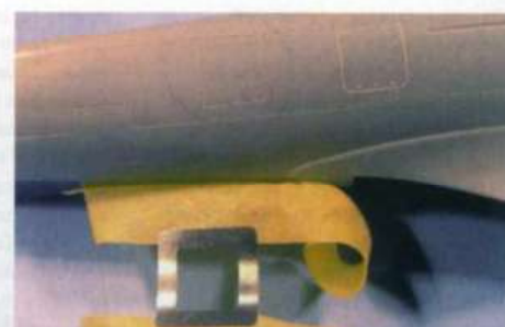
Here the photo-etched template has been used to rescribe the radio hatch in the correct place for the F Mk 24
