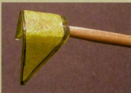
The first coat has been brush applied, and left to dry. This coat is translucent, but will act as a key for subsequent coats.
