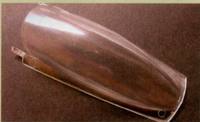
Not easy to discern in this photo but after work with the 8000 grade cloth the canopy no longer shows any sign of the seam and clarity is being restored.
