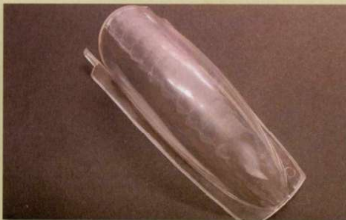
The polishing cloths are now used to work the roughened plastic back to a smooth, and consequently clear surface. Wet polishing is preferred and under way in this photo. Wipe the canopy clean periodically with a clean dry cotton cloth to check on progress.
