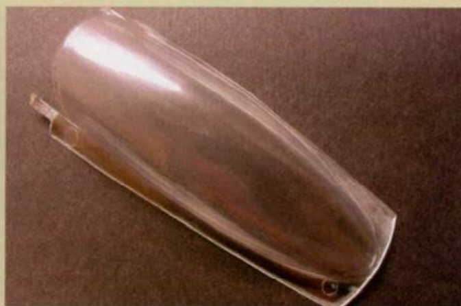
The cloths are used in order starting with the 3600 grade and working up to the 12000 grade, with the polishing action being back and forth (rather than the more usual circular action) with each grade being worked at right angles to the previous. When purchased, instructions are normally contained with the cloths. This photo shows the canopy after about 5 minutes' work with the 3600 and 4000 grade cloths
