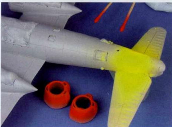
These parts needed painting first before applying the camouflage, for my chosen scheme at least
