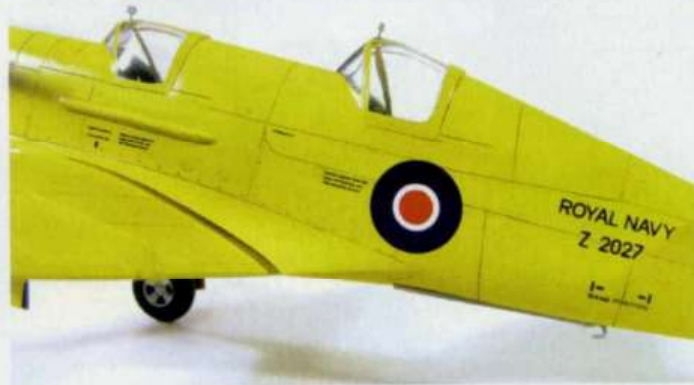
The two-seat fuselage is the main new part in the basic Firefly kit, combined with a new cockpit interior for the 'back seat' and a new canopy
