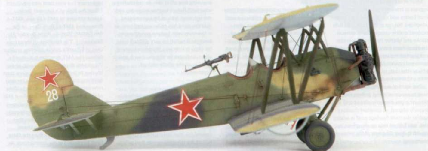
The struts are positioned correctly by using a jig made of plasticard to simulate the top wing. This has the holes drilled at the correct locations
