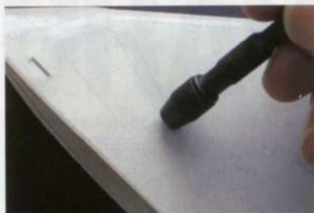
A 0.3mm drill bit is used to enhance the larger moulded rivets
