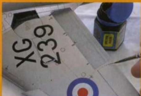
Citadel Brown Wash ink is used to enhance the panel lines and rivet detail
