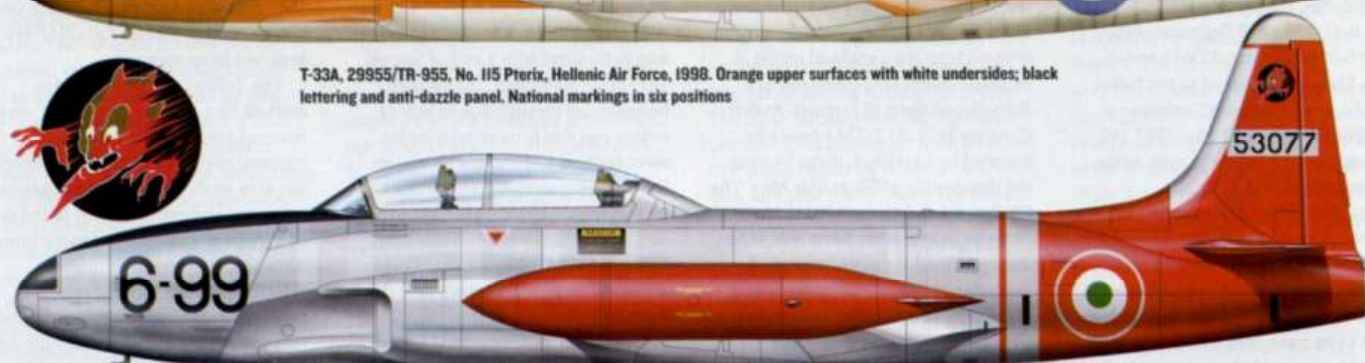
T-33A, 53077/6-99, 6° Aerobrigata, Aeronautica Militare Italiana. Natural metal overall with black anti-dazzle panel and lettering; red outer halves of wingtip tanks and tail unit. Inner halves of wingtip tanks in black; unit badge on fin
