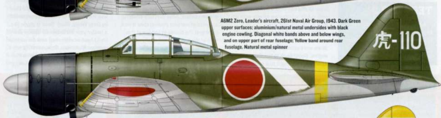
A6M2 Zero (Nakajima-built), Kounoike Flying Group, Kounoike (Japan), 1944. Green upper surfaces with Light Grey undersides; black cowling. Polished metal spinner and propeller (with black facing pilot)
