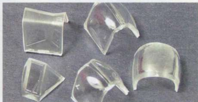
The kit windscreen and canopies, note the prominent moulding seams. The hood on the right has had the seam scraped off with a scalpel and polishing (using Micromesh) has begun
