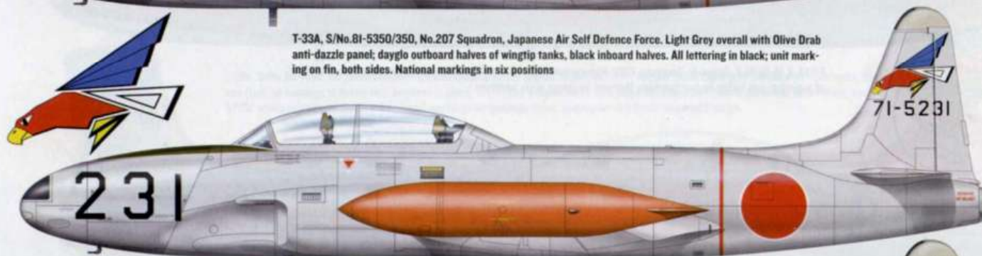
T-33A, S/No.71-5231/231, No.302 Squadron, Japanese Air Self Defence Force. Aluminium overall with Olive Drab anti-dazzle panel; black lettering. Dayglo outer faces of tip tanks, inner halves in black; unit badge on fin, both sides. National markings in six positions
