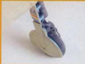
Opting to use resin 'weighted' wheels does give you piece of mind in knowing that these won't degrade as rubber does
