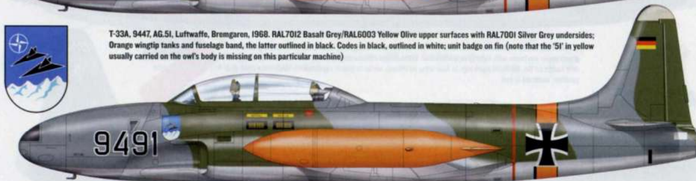
T-33A, 9491, JG34, Luftwaffe, 1975. RAL7012 Basalt Grey/RAL6003 Yellow Olive upper surfaces with RAL7001 Silver Grey undersides; Orange wingtip tanks and fuselage band, the latter outlined in black. Codes in black, outlined in white; unit badge below windscreen
