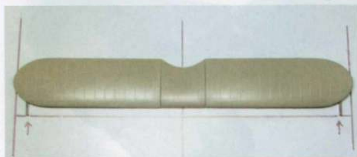
Using the same card and strips the same dihedral can be given to the top wing
