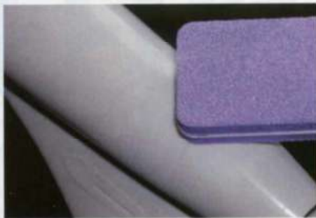
A medium sander from MasterCasters is used to sand all the joins
