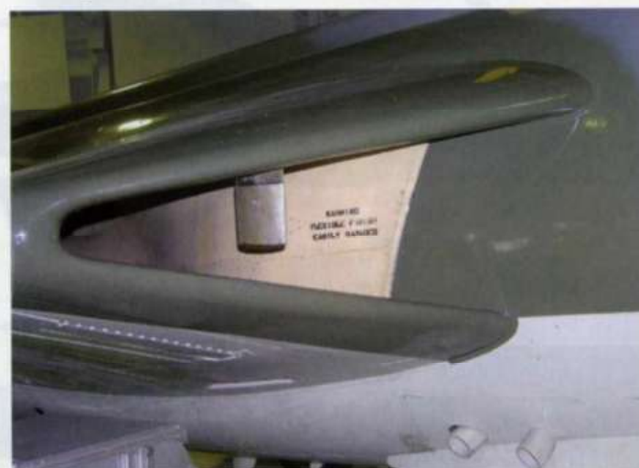
A look into the intake, showing the 'flexible' paint in this area (note warning stencil) and the wrap-around of the exterior colours
