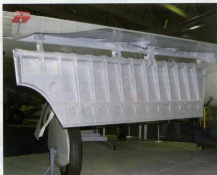
The inboard flap area, only exposed like this because the hydraulic pressure has drained away causing them to hang down at 90°
