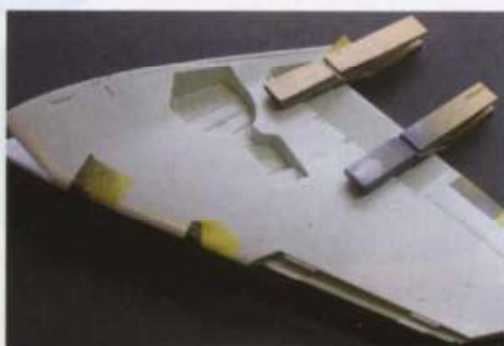
Clothes pegs are very useful for holding the joint while the cement cures
