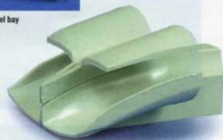
Here you can see the resulting central seam inside the intake
