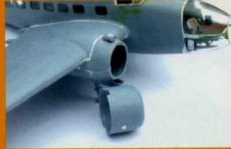
I had to saw off a lump of the nacelle to get a better fit for the engine cowl
