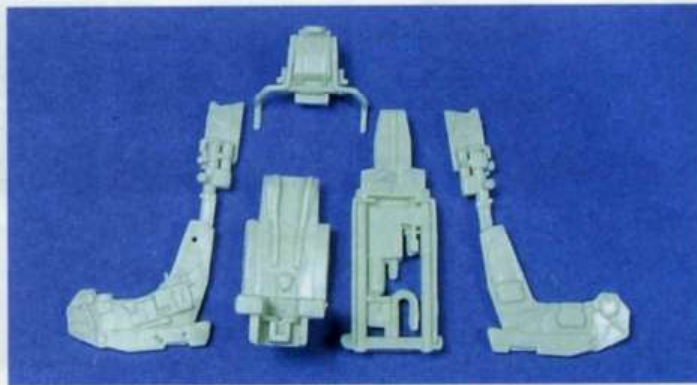
The seat is made up of five parts. Note the moulded-in seat belts
