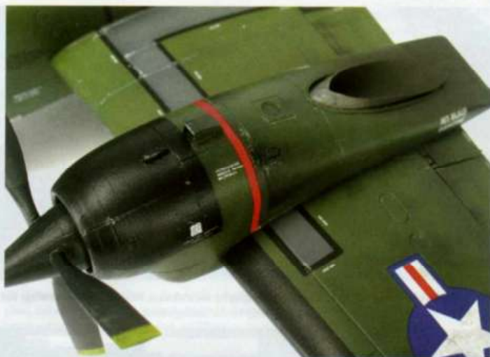
The new photo-etched exhausts for the engines are probably one of the most daunting aspects of the detail set, but their addition is well worth it
