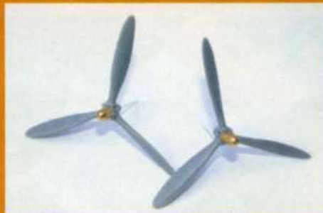
New hubs, turned on a lathe, were fitted to each propeller
