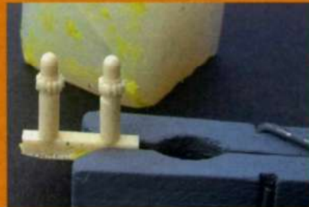
The new hubs were then set in rubber and new copies cast in resin
