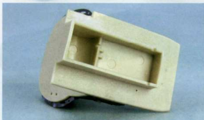
Above left & right: Fairly simple additions to the front wheel well include the new interior skin and some pipes along either sidewall
