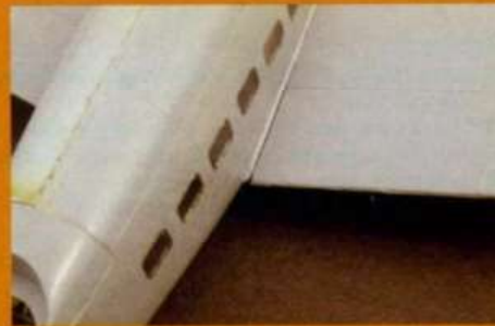
The fit of the wing at the root/trailing edge was not good either
