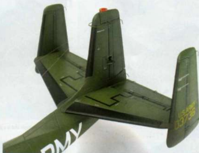
The three-fin assembly of the Mohawk is quite unusual and with all the deicing boots and walkway stencils plus the addition of static wicks from the Eduard set it is very busy indeed
