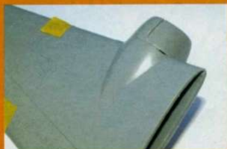
These two views illustrate very clearly just how poorly the engines nacelle components fitted
