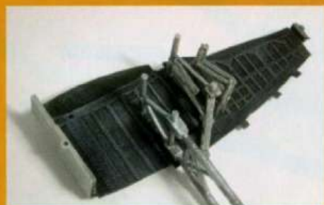
Here you can see the combination of plastic, photo-etched and white-metal parts that make up the undercarriage
