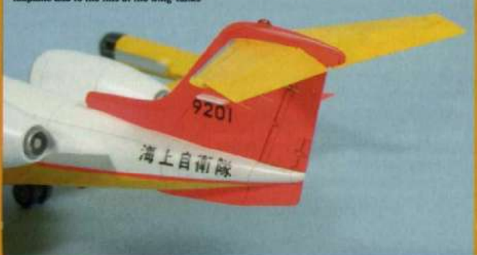
Static-wick dischargers made from stretched sprue have been added to the tailplane and to the fins of the wing-tanks
