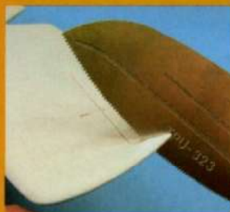
Cuts are made in the wings at the ends of each aileron
