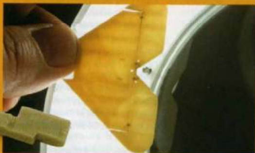
Once the elevators are cut and deflected you can locate the control cable holes by holding the assembly up to a bright light source
