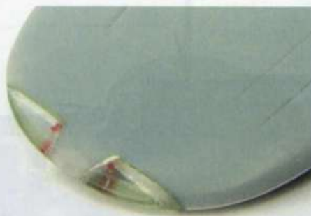
The wing tip lights were replaced with clear plastic and will later be polished to restore their clarity
