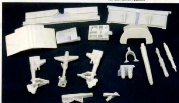
Here are the smaller parts, including the undercarriage, doors, air brakes, tail hook and refuelling probe
