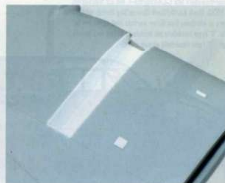
The 'trench' made in the lower wing panel within the confines of the wheel well
