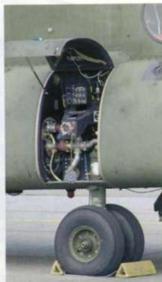
One of the many ground access panels on the type, this one being above the front oleo unit on the starboard side
