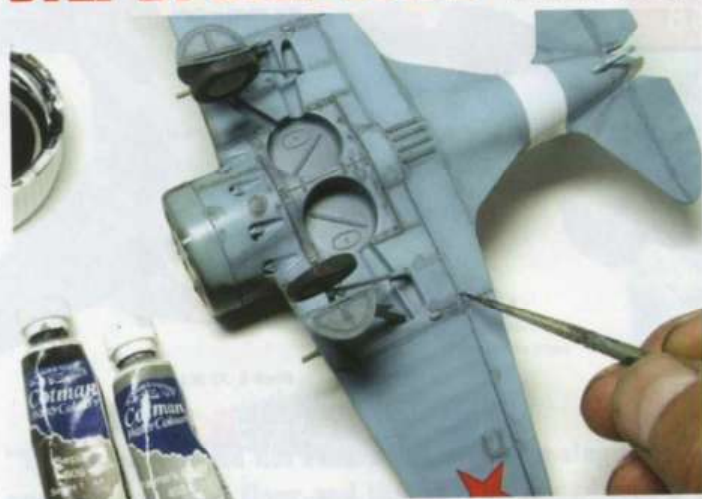
A watercolour grey wash was added to the underside, the gloss varnish coat helping its application
