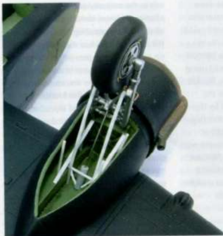
All the retraction arms and linkage were added to each wheel well
