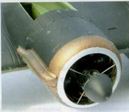
The support stays for the collector ring have been added
