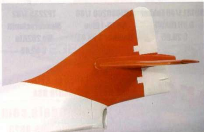
Careful masking is needed before the orange areas are sprayed on. Here the vertical fin is shown
