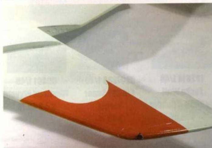
The wing tips need careful masking otherwise the orange will bleed through the white of the national insignia
