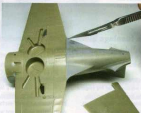
The rear wing-to-fuselage joint was slightly high at the corners
