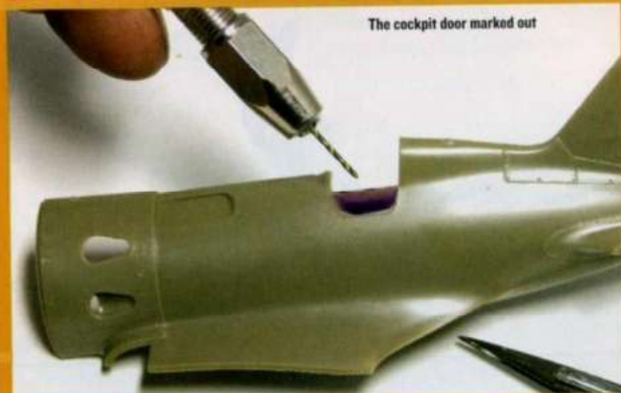
Drill around the area to be removed, then join holes with scalpel
