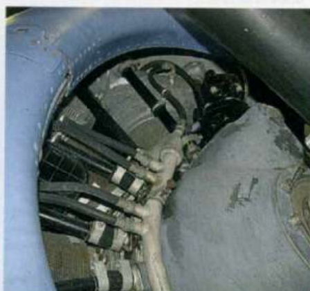
The ignition harness around the engine is prominent here
