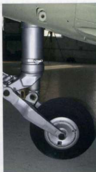
Overall view of the nose wheel leg. The square tube is just to stop the scissor link collapsing, it is not original!
