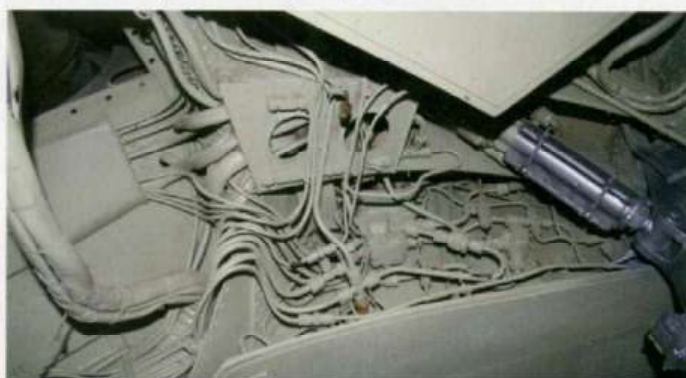
A look inside the starboard main undercarriage bay. The uniform Sky colour is presumably the result of repainting during restoration work
