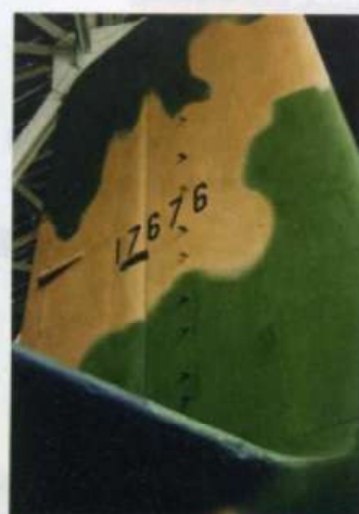
The vertical fin, complete with little plates (vortex generators) to create 'dirty' air to make the rudder and trim tab more effective
