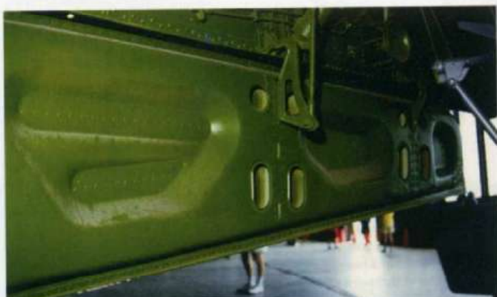
Closer view of the structure of the nose wheel doors
