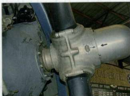
Close-up of the propeller boss, note the alignment marks on both boss and hub
