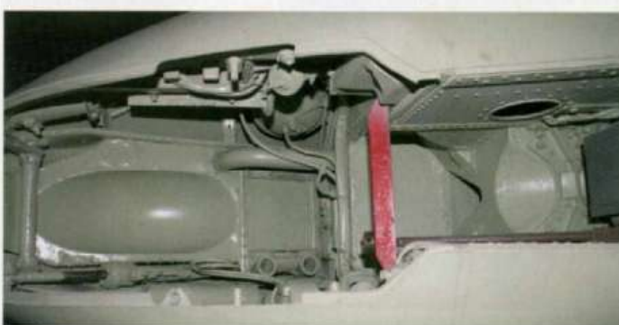
Looking up into the nosewheel bay. Note the tyre recess up front. The red bar appears to be a type of locking pin
