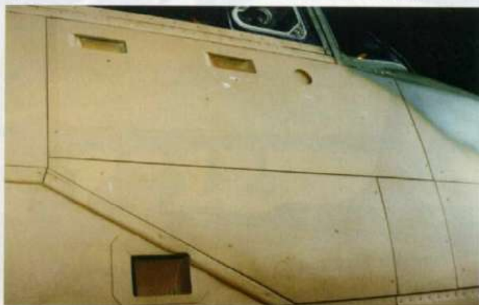
The appliqué armour on either side of the cockpit area on the A-26K has wooden beading along the bottom to reduce sharp edges and thus airflow disturbance
