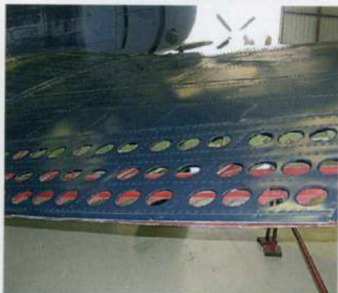
Overall view of the upper surface of the split flap/dive brakes. The interior was painted red to make their operation easily visible to other aircraft
