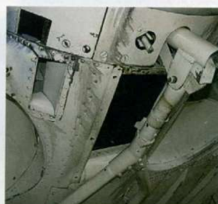
Here you can see the sighting window in the fuselage underside, the chutes for the cartridge cases and the cradle for the bomb
