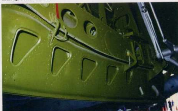
A close look at the structure of the inner faces of the main undercarriage doors
