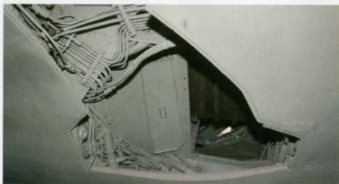
The port main undercarriage bay. Note how it is possible to see right through to the other side beneath what is probably the engine housing
