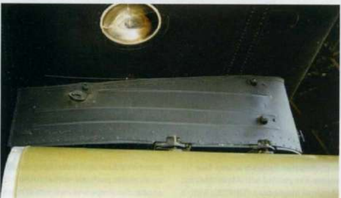
One of the underwing pylons, fitted with a rocket launcher. The overall finish is black, but as you can see it is really a very, very dark grey
