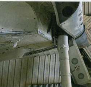
Overall, inside view of the port oleo. The bays would have been the same colour as the underside, to prevent saltwater damage in these areas
