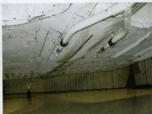
A look back along the underside, you can see the steady plates for the bomb in line with the arms of the cradle
