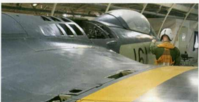
View of the starboard forward fuselage, with auxiliary air intake louvres and an open fuselage panel. Note also the open panels above the wing fold mechanism
