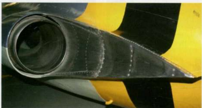
The port jet pipe. The engine turbine is just visible
