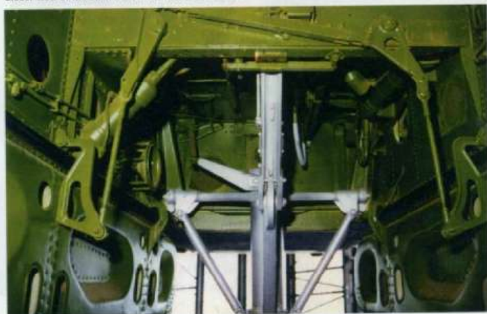
Up inside the nose wheel well, looking forward, you can see the single hydraulic ram on the port side that via linkage closes both doors
