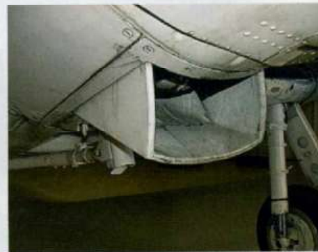
The carburettor air intake drops down into the airflow underneath the cowl
