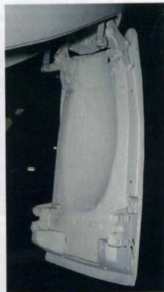
This is the nose wheel door, seen from behind with the linkage at the top and locks at the bottom
