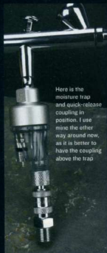
The in-line moisture trap has a tyre valve set into it (visible at the top), which allows you to vent out moisture
