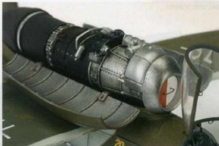
The kit gives the option to build the kit so the engine you see here can be taken in and out, with the blanking plate in the intake stopping that see-through effect
