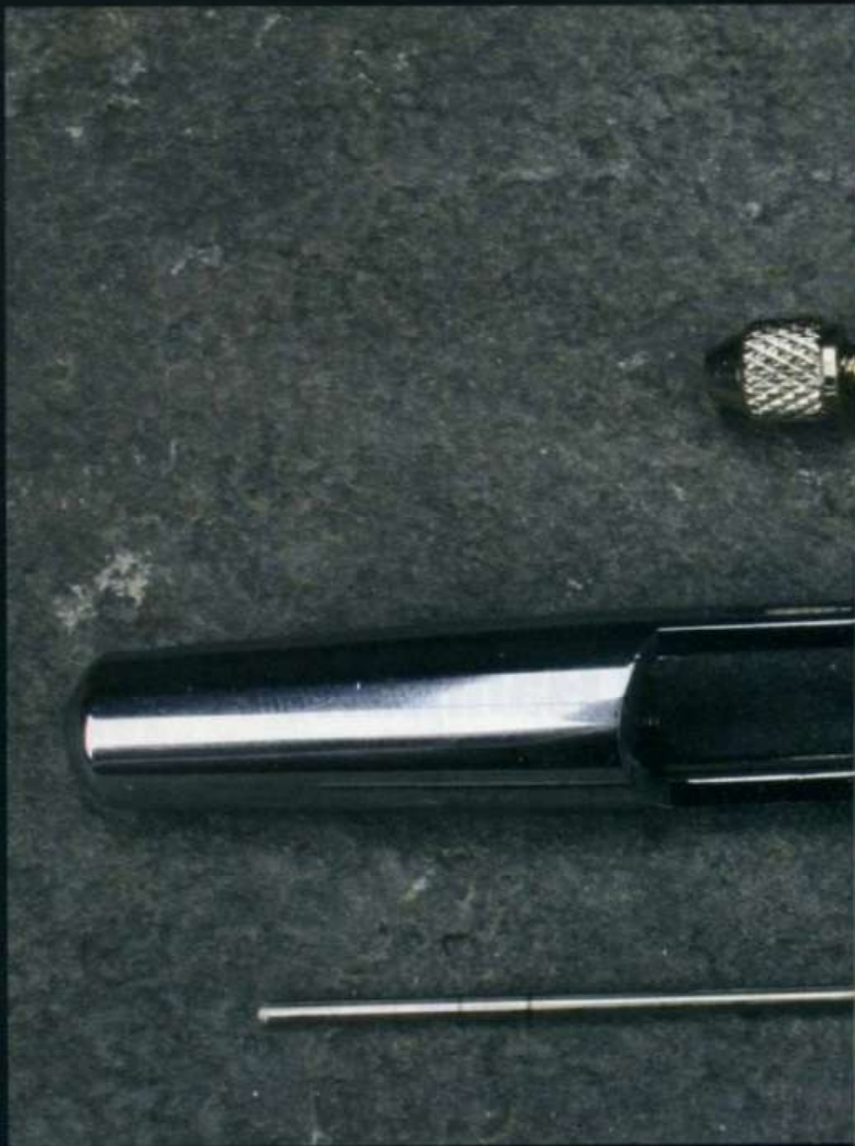
The airbrush broken down into component form. The only item not visible is the fluid tip in the body which I had not wanted to remove without suitable (plastic) tweezers to avoid damage!
