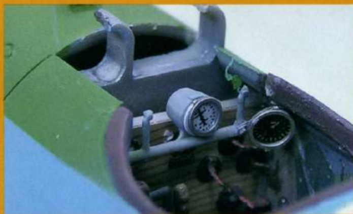
All the gauges are from the kit's pre-painted photo-etched
