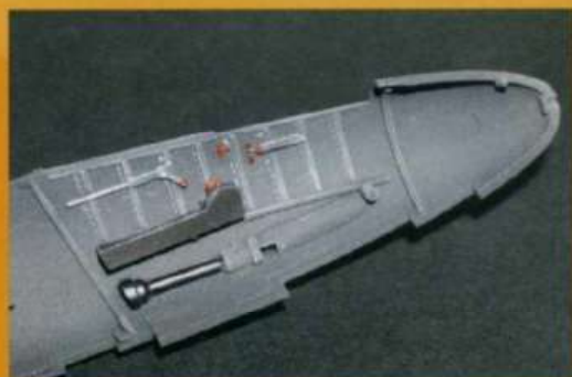
Left fuselage half painted RLM 66 and drybrushed in a lighter shade of grey. Some basic details are picked out in red as on the real machine
