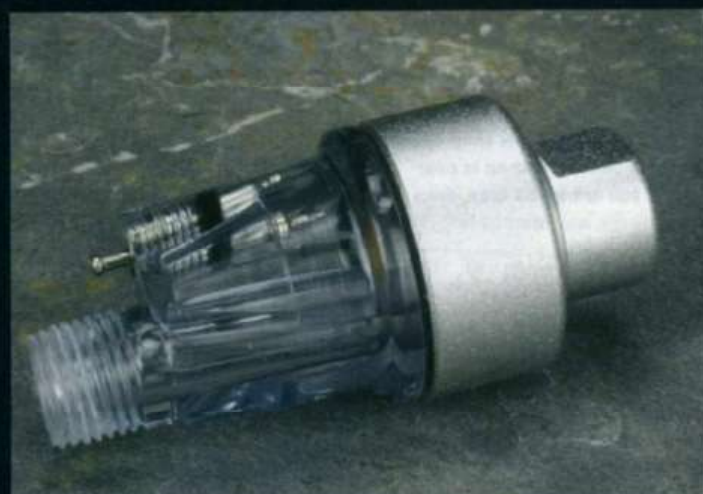
The in-line moisture trap has a tyre valve set into it (visible at the top), which allows you to vent out moisture
