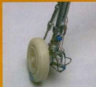
Adding some hydraulic plumbing to the main gear struts
