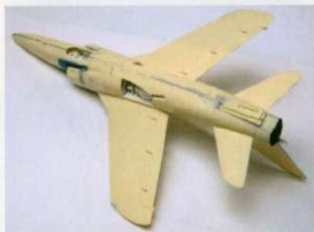
The large wing tip beacons were replaced with clear sprue sanded to shape and glued over a Bare-Metal Foil background
