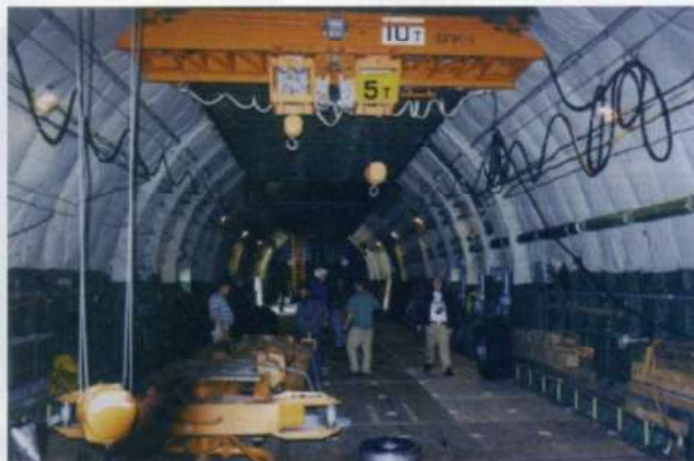
The cargo area again, this time looking towards the front. Note the crane built into this area
