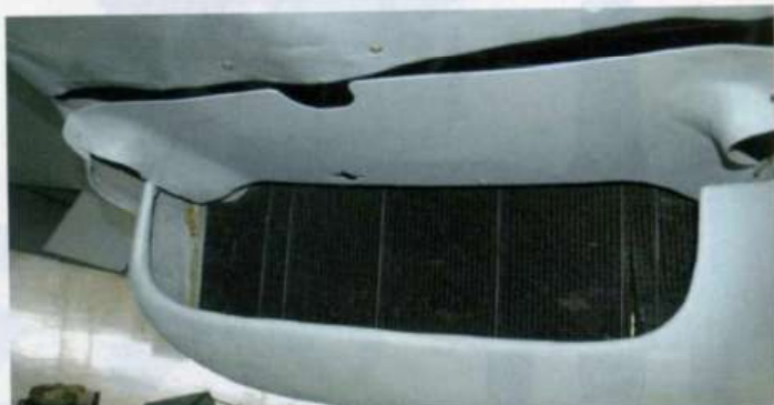
This view shows the front of the radiator under one of the engines. The slightly less than perfect fit of the cowls is all down to their repair during restoration, as this was an aircraft that crash-landed and was outside for 40+ years
