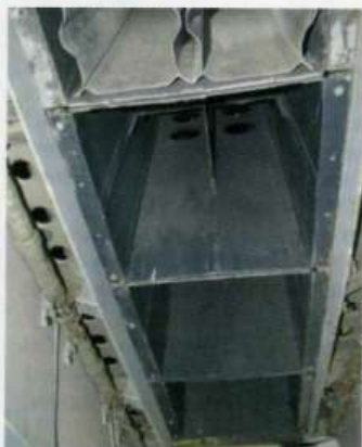
A very useful shot for those of you using the Eduard bomb bay set, this shot is looking up into the vertical bomb cells
