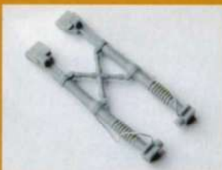
Electrical wire will help the look of the oleo forks greatly
