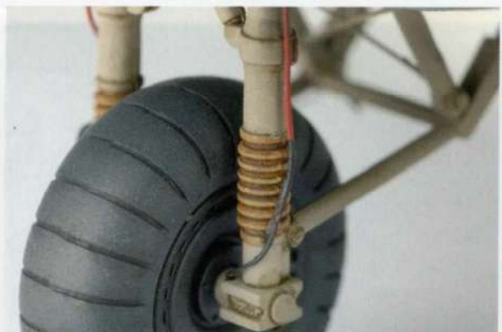
Little needs to be added to the undercarriage legs, just the brake line made from wire. The wheels are better in the kit than the aftermarket ones produced by True Details, so were retained here
