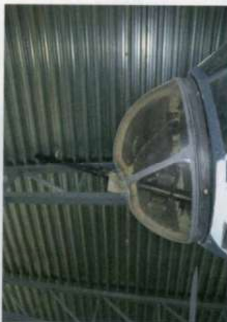
Close-up of the rotating cupola in the nose of the He III
