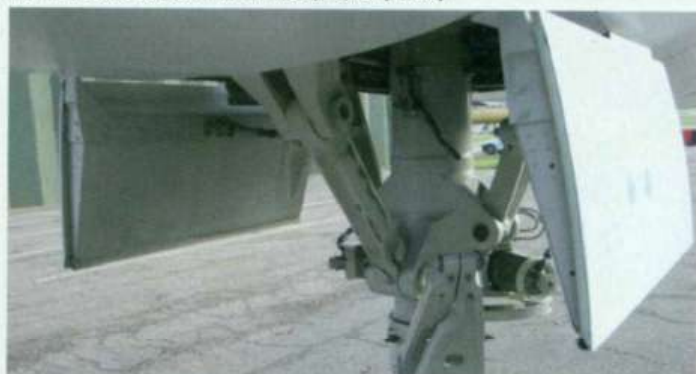
The top of the nosewheel oleo and associated linkage viewed from the back, looking forward
