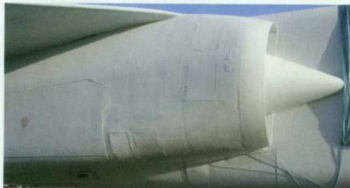
The intake viewed from the starboard side. The stressed skinning is nicely high-lighted in the early morning sun, as are the two intake bleed doors. You can also get a feeling for the correct profile of the wing and its leading-edge from this shot
