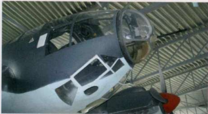
This overall view of the nose area clearly shows the 'sucking in' that occurs behind the cupola, as mentioned by John in his article and lacking on the Hasegawa kit
