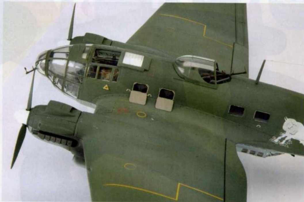
The access panels open alongside the bomb cells add interest to the otherwise drab RLM 70/71 camouflaged fuselage
