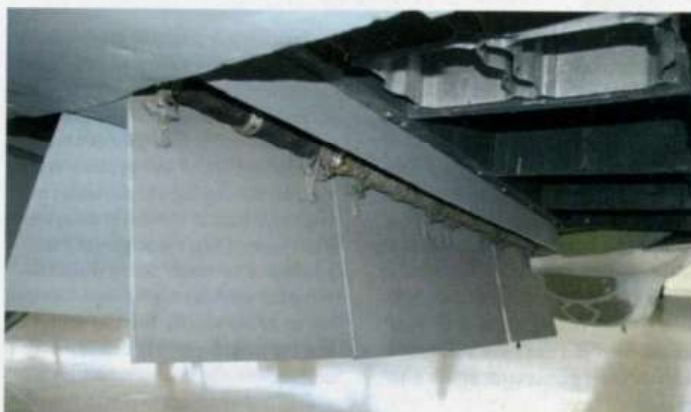
This slightly lower perspective shows the doors and their hinge points. The deflection correctly seen in the Eduard set and on John's model no longer exist on this machine
