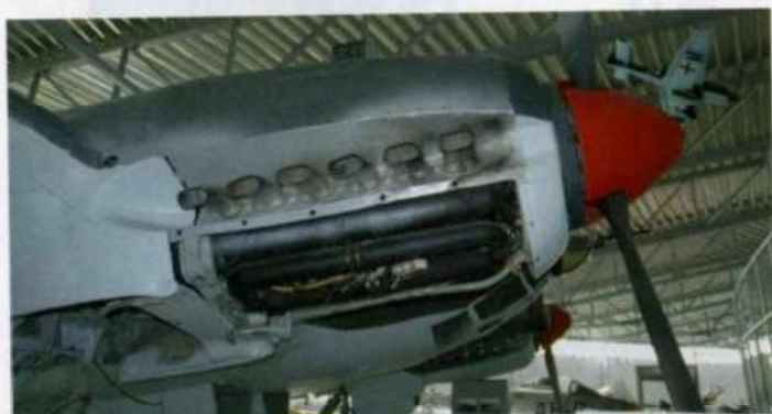
The outboard face of the port engine nacelle, this time with the upper cowl section in place but the lower one removed
