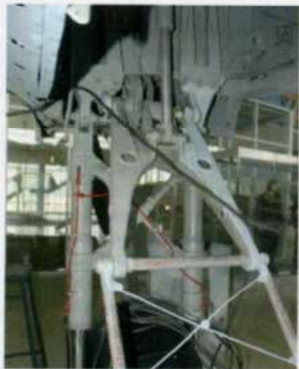
While this view from the back of the undercarriage shows all the framework and bracing wires, as well as the warning stencils
