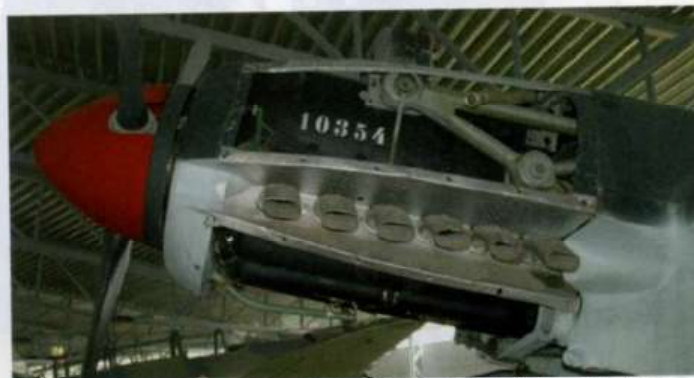
The same engine looking outboard (note the Northrop N3P in the background). This machine lacks engine cowls for this engine, or undercarriage doors, as these are parts that were either removed from or destroyed at the crash site
