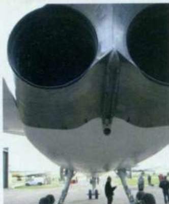
Viewed directly from behind here you can see the exhaust cans projecting slightly aft of the unpainted tail cone and the connection between the engines for the braking chute
