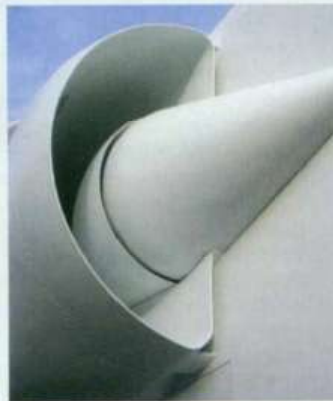
A close look into the starboard intake. The little spacers at the bottom and top connecting it to the fuselage side and the way the shock cone slots into the inner element resulting in a gap are all very helpful
