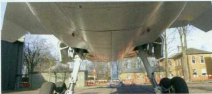
An unusual view underneath and looking backwards. The various access panels, gear and bomb bay doors are all visible as are the two little vent pipes forward, and either side of the undercarriage bays
