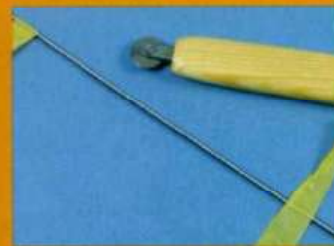
I wanted to recreate the rivet detail along the framework, and using 'Rosie the Riveter' on the reverse side of the plastic strip I was able to easily manage this task. Mind you, keeping the Microstrip in the tiny 'U' channel whilst running Rosie along its length was no easy task
