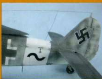
The aerial arrangement for the rear fuselage; wires above and a little whip aerial below
