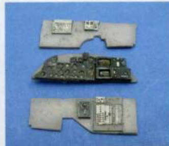
The dials on the instrument panels come from various spare decal sheets and were covered with gloss varnish
