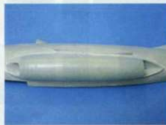
A view of the whole nacelle-to-fuselage joint
