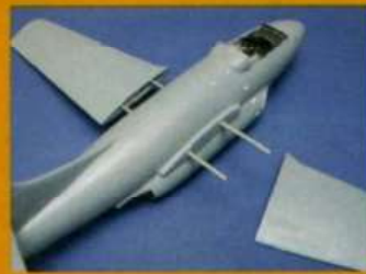
Reinforcing the wing joint with two aluminium tube spars that go through the fuselage
