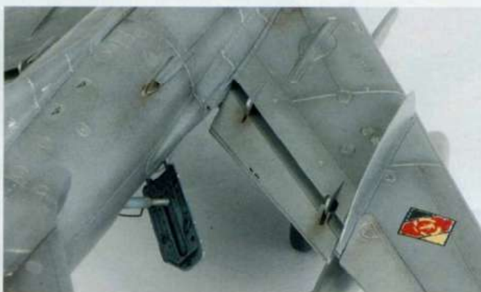
Wing fences and big air brakes on the fuselage sides, it just has to be a MiG!
