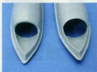
The exhaust lips before (left) and after intensive sanding (right). Note the over-flat aspect of the left section, which, although incorrect was left 'as is'
