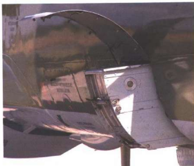
One of the ammunition boxes for the ventral gun seen partially removed
