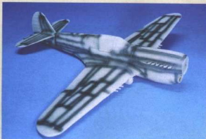
First steps in the painting process. A base coat of grey primer has been applied with the airbrush and panel lines have been shaded with a random application of gloss black paint
