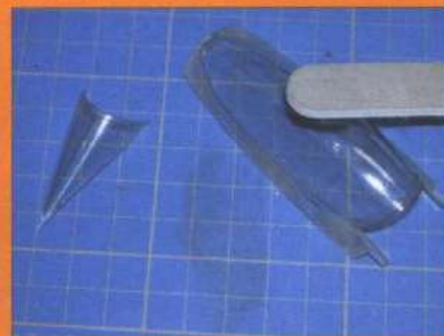
The bulged canopy and clear rear section are very clear and fit well. The thin mould seam line is readily removed with a nail buffer as you can see here and given a final polish with MER car polish
