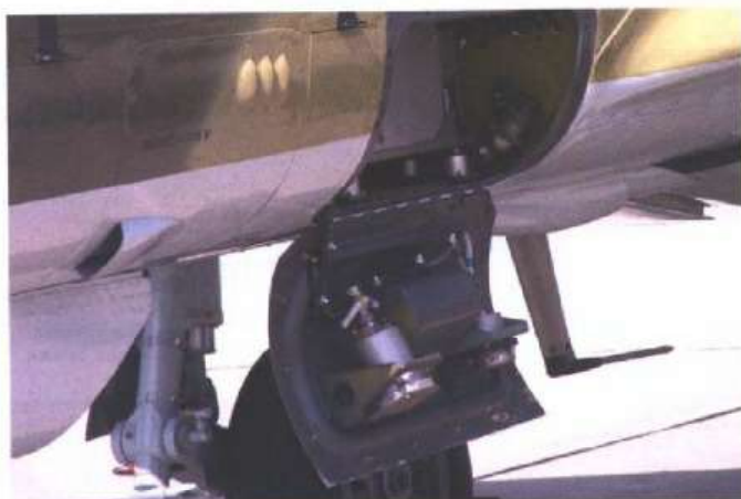
Close-up of the hinged access panel on the port fuselage side
