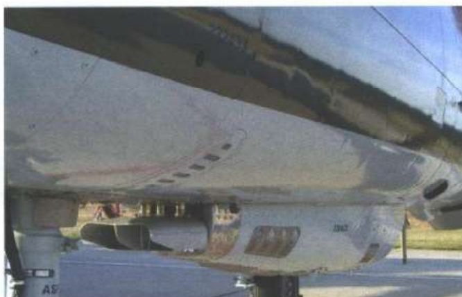
A look up underneath the forward fuselage, showing the twin gun pack in this area
