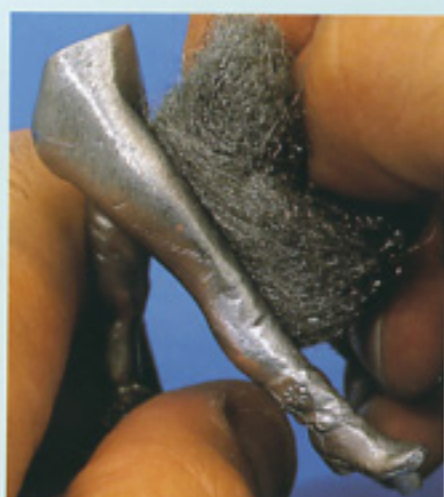
Polishing with steel wool.
