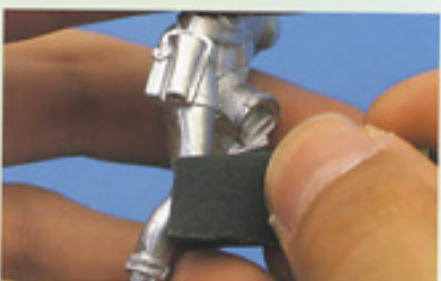
Retouching pieces with blade, file and fine sandpaper.
