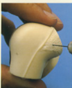
Retouching and sealing joints.
