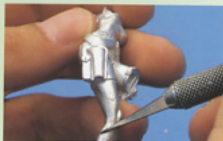
Retouching pieces with blade, file and fine sandpaper.
