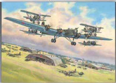
The TB-3 heavy bomber was the workhorse of the pre-war Soviet offensive bomber forces. This aircraft became the basis of many experiments. One of them was the "Aviamatka" air carrier system created in 1935. This system included the TB-3 carrier with two I-5 and two I-16 parasite aircraft.
