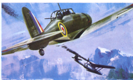
F.162 BLACKBURN SKUA This was the Fleet Air Arm's first operational monoplane and it claimed the first German aircraft (a Do 18) destroyed by the Fleet Air Arm in World War II. Entered service in 1938 on the carrier H.M.S. Ark Royal. Total production was 190 aircraft.
