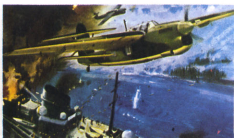
F.161 FAIREY BARRACUDA This versatile aircraft entered service in 1943 as the British Navy's first monoplane torpedo bomber. It could carry bombs, mines, depth charges, torpedos and lifeboats and was used to attack the Battleship Tirpitz off the coast of Norway in 1944. Total production was 2,582 aircraft.
