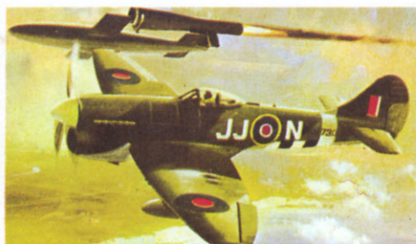
F.189F HAWKER TEMPEST MK. V The only version of the Tempest to see War service. It is best remembered for destroying 638 Flying Bombs over Southern England between June and September 1944. 805 Tempest V's were produced and they entered service in January 1944. Top speed 435 mph, range 1,530 miles.
