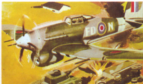
F.209F HAWKER TYPHOON This aircraft was probably the best ground attack aircraft on either side during the Second World War. The Typhoon could carry two 1,000 bombs—the heaviest load of any single engine aircraft at that time—or eight rocket projectiles. On one day—7th August 1944—they destroyed 135 enemy tanks.
