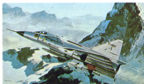
F.264 SAAB VIGGEN (THUNDERBOLT) This impressive aircraft was made especially for Sweden's 500 metre trunk road airstrips. It was first flown in February 1967, and has a maximum speed of 1320 mph. It carries air to surface and air to air guided missiles and can operate at a height of 60,000 feet.
