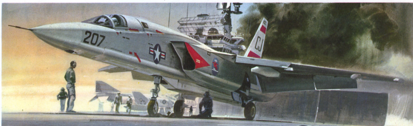
F.275 NORTH AMERICAN RCA VIGILANTE The largest attack bomber ever built for operations on board U.S. Navy aircraft carriers. It was converted to a reconnaissance aircraft in 1962 and was first operational in the South China Sea. It has a maximum speed of 1385 mph and a combat range of 2,000 miles.
