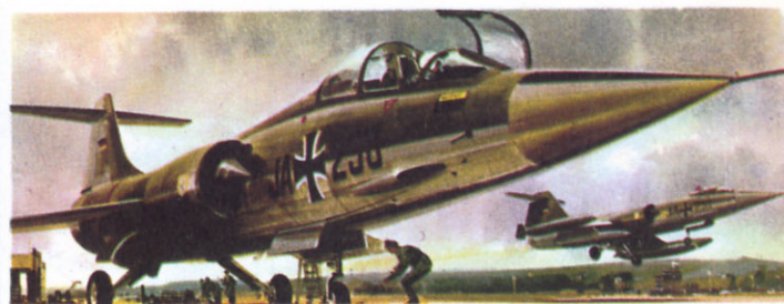
F.268 LOCKHEED F.104 STARFIGHTER First flew in February 1956 it was destined to become one of the most widely operated fighters of the 1960's and it has been manufactured in Japan, Canada, Germany, Holland, Italy and Belgium. It has a maximum speed of 1450 mph and a combat range of over 1,000 miles.
