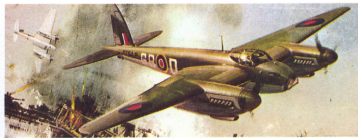
F.187 DeHAVILLAND MOSQUITO MK.4 OR MK.6 This was one of the great British combat aircraft of World War II. Very versatile it remained the fastest type in Bomber Command for nearly ten years until outpaced by the Canberra jet. Mosquito fighters shot down 600 V-1 Flying Bombs in two months. Maximum speed 380 mph.
