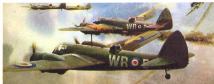
F.190 BRISTOL BLENHEIM MK.1 OR MK. 1F This light bomber went into service in 1937. Of the 1,552 produced some 200 were converted to the Mk. 1F night fighters. It was faster than the fighter aircraft of the day having a maximum speed of 260 mph and a combat range of 1,125 miles.
