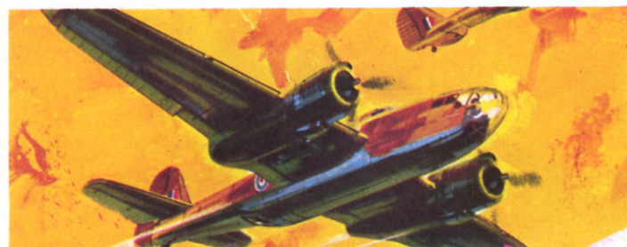
F.339 MARTIN BALTIMORE First flown in June 1941 it was operational with at least seven R.A.F. and two S.A.A.F. Squadrons from 1942 onwards and served exclusively in the Middle East. It has a maximum speed of 308 mph and a combat range of 1,082 miles.
