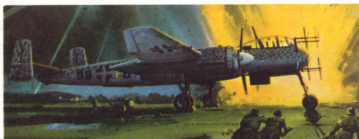
F.177 HEINKEL 219A-2 UHU (OWL) This was the first production model of the series and carried a crew of two and an armament of 2 cannon and 4 machine guns. It was powered by two 1750 hp DB 603A liquid cooled engines. Total production of the A series was 268 aircraft.
