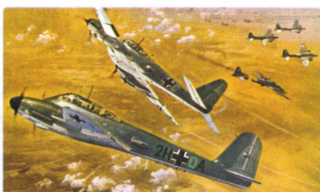
F.178 MESSERSCHMITT 410A-1 OR A-1/U4 This aircraft named the Hornisse (Hornet) was developed as a fighter bomber and a "heavy" fighter with extra "cannon" in the bomb bay. Total production was 1,121 aircraft of which over 100 were built in Hungary. It had a maximum speed of over 380 mph.
