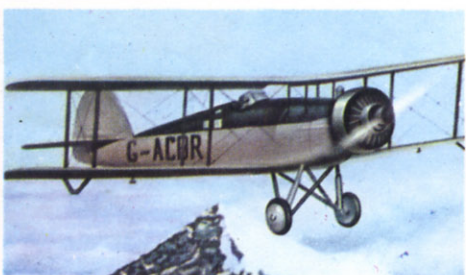
F.167 WESTLAND WALLACE A record breaker from the golden years of daring exploits. In 1933 it became the first aircraft to fly over Mount Everest. It became the first R.A.F. aircraft to have a canopy enclosing both cockpits giving greater comfort and allowed the gunner to be more effective.
