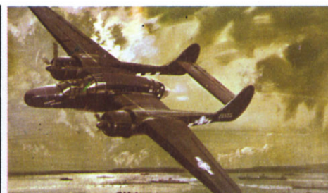
F.170 NORTHROP P. 61 BLACK WIDOW These all black aircraft were appropriately named after the venomous North American Spider. Designed as radar equipped night fighters they first saw operational service in the South Pacific in the early summer of 1944. The aircraft had a maximum speed of over 300 mph.
