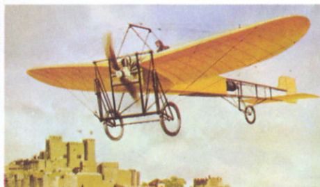
F.173F BLERIOT XI The aircraft used by Louis Bleriot to make the first cross-channel flight from France to England on 25th July, 1909. If rain had not cooled his 24 hp 3 cylinder engine he would probably have failed in his attempt.
