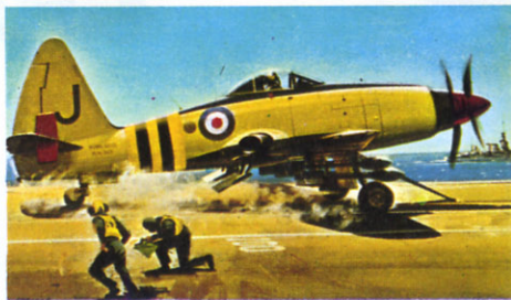
F.198 WESTLAND WYVERN The Wyvern was single-seat carrier borne strike aircraft which first flew in December 1946. Standard armament was four 20 mm cannon, a 20 inch torpedo, bombs or mines, or a combination of depth charges and rockets. It had a maximum speed of over 380 mph at sea level.
