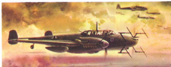
F.202 ME. BF. 110 The first Messerschmitt designed warplane to use twin engines, first flew in May 1936. It began to enter service in 1939 and over 500 aircraft were in use by the end of the year. It had a maximum speed of 349 mph and a combat range of 565 miles.
