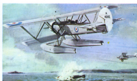
F.179 BLACKBURN SHARK Powered by an Armstrong Siddeley Tiger engine, the Shark was a two/three seat torpedo-spotter-reconnaissance aircraft designed as either a land-plane or sea-plane. After being superseded as a first line aircraft by the Swordfish in 1938 it was used for training duties.
