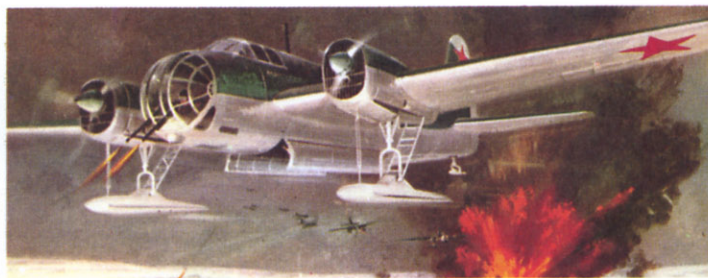
F.176 TUPOLEV SB2 This medium range bomber first flew in December 1934. With a maximum speed of 260 mph and a combat range of 745 miles, it was a difficult target for anti-aircraft fire and it was superior in performance to many of its contemporaries.
