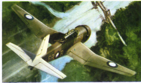
F.199 VULTEE A31-A35 VENGEANCE This single-engined light attack-bomber was adopted by the R.A.F. as a dive-bomber, and was used extensively in Burma. It could carry a bomb load of 2,000 lb. and had a maximum speed of over 270 mph and a combat range of over 600 miles.
