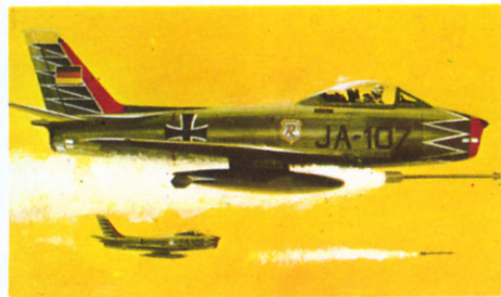
F.267 NORTH AMERICAN SABRE Destined to become one of the truly great combat aircraft of all time, this aircraft, the first swept wing fighter of the USAAF first flew in October 1947. It had a top speed of 680 mph and a range of 920 miles.
