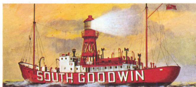
F.138 SOUTH GOODWIN TRINITY LIGHTSHIP This famous lightship was built of construction steel in 1954 and is moored at the South Goodwin Sands. The range of its lights is 12 miles on a clear day. In foggy weather the ship has a diaphone fog signal of two blasts every 60 seconds.
