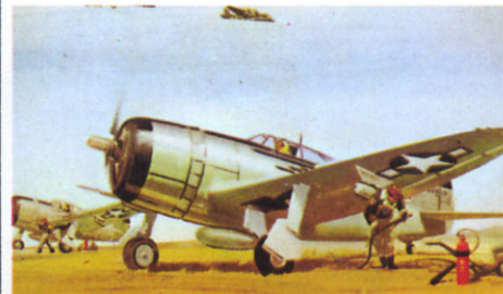
F.210F REPUBLIC THUNDERBOLT P47 The largest and heaviest single-engine single-seater fighter built and flew for the first time in May 1941 and became operational in November 1942. They operated successfully in Europe, the Mediterranean, the South West Pacific and China. A grand total of 15,660 Thunderbolts were produced.
