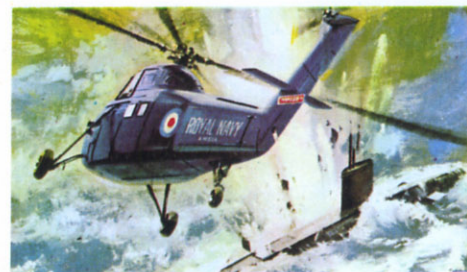
F.335 WESTLAND WESSEX This aircraft was intended primarily for anti-submarine duties and air sea rescue work. It has a crew of four and can carry either two torpedos or four missiles or 2 in. air to surface rockets. There was a Marine Commando version which could carry 16 Commandos or 8 stretchers.
