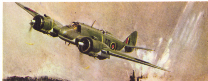
F.191 BRISTOL BEAUFIGHTER Given the nickname of "Whispering Death" by the Japanese, this aircraft was two-seat twin-engined fighter with heavy armament and a maximum speed of over 300 mph which combined to make it one of the most formidable and versatile British combat aircraft of World War II.
