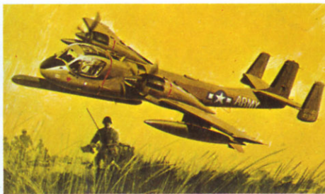
F.270 GRUMMAN OV-1B MOHAWK This aircraft first flew in 1959 and is still operational to-day. Planned solely as a reconnaissance aircraft it has two turbo-prop engines and can travel at low speeds for considerable periods of time. It is equipped with side looking airborne radar.
