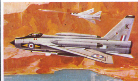
F.266 B.A.C. LIGHTNING F.6 This single-seat twin-engined all weather fighter can exceed the speed of sound in level flight and it was the first fully supersonic aircraft in service with the R.A.F. Armed with cannon, rockets, bombs or missiles and travelling like "Lightning", it is the last word in defence aircraft.
