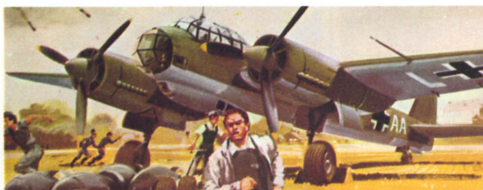
F.160 JUNKERS JU88 A-4 This bomber was the backbone of the Luftwaffe and was developed from the JU 88A-1 incorporating experience gained from the "Battle of Britain". It had an increased defensive armament, greater bomb load and a larger engine. Maximum speed was 293 mph with a combat range of 1,695 miles.
