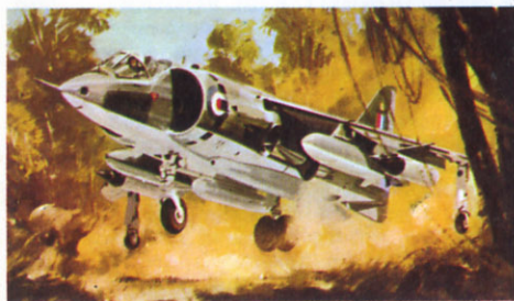
F.273 HAWKER SIDDELEY HARRIER This is an advanced vertical/short take-off and landing close support and armed reconnaissance aircraft which first flew in 1966. It is armed with guns, rockets and bombs and can take off and land vertically. It is designed to be self contained at forward air base needing no ground personnel.
