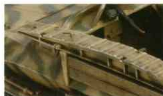
■ New two assault bridge and mounting brackets for Sd.Kfz. 251/7
