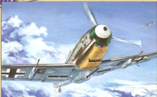
7236 Bf.109G-2/MG 152/20 To attack the enemy bombers, the Bf109 was fitted with auxiliary gun pods which much improved its firepower.
