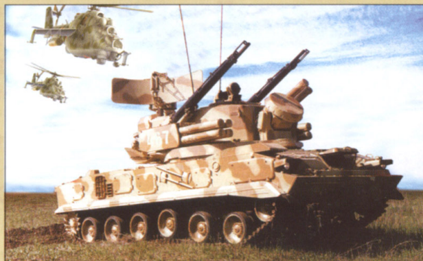
7204 2S6 Tunguska Armed with 4 30-mm guns and 8 missile tubes, the 2S6 is the best mobile AA-system today.
