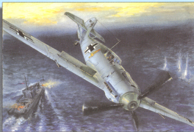
7214 Bf 109T Carrier-born version of the famous Bf 109 featured larger wingspan and a landing hook.
