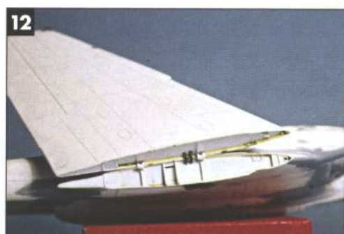
12 The first step in folding is to install bulkheads. Each hinge point actually works. The black "hoses" are stiff wires that help support the folded wings.
