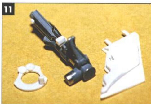
11 Not even the landing gear escaped detailing. The disc is the brake, and the strut was detailed with styrene and wire.
