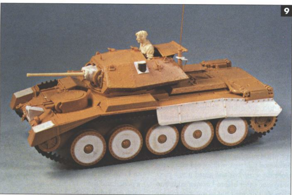
Using a compass and hole punch, Peter made the wheel covers from styrene sheet.
