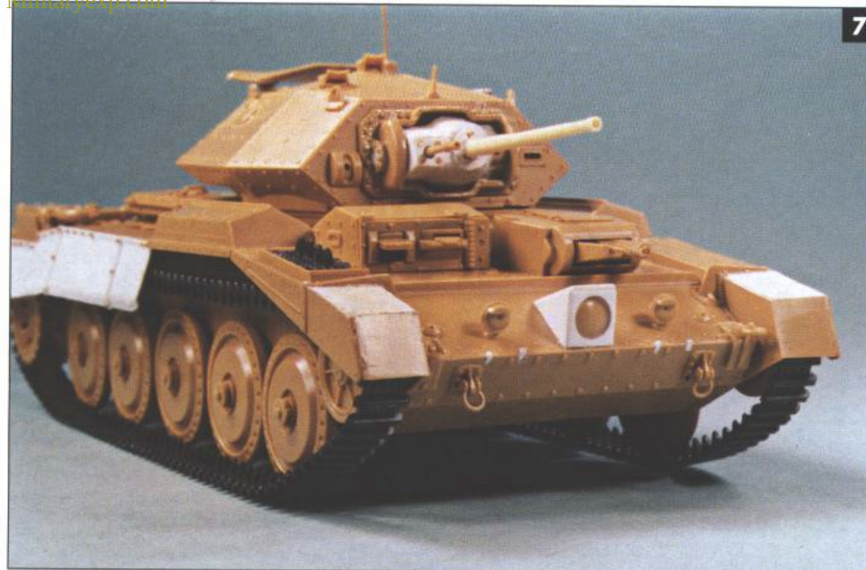
Peter replaced the kit fenders with styrene sheet and thinned them to scale.
