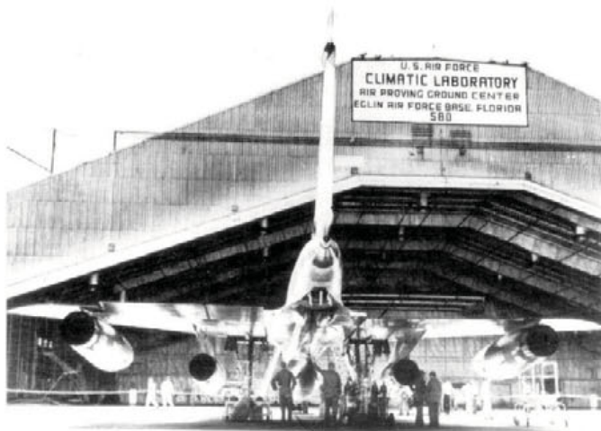
As part of the overall development programme of the Hustler, one of the pre-production aircraft was assigned to the Air Force Proving Ground at Eglin AFB, Florida. This is seen shortly before it entered the climatic laboratory where it was subjected to extremes of temperature designed to test the operational flexibility of the B-58A's complex systems. (Convair)
