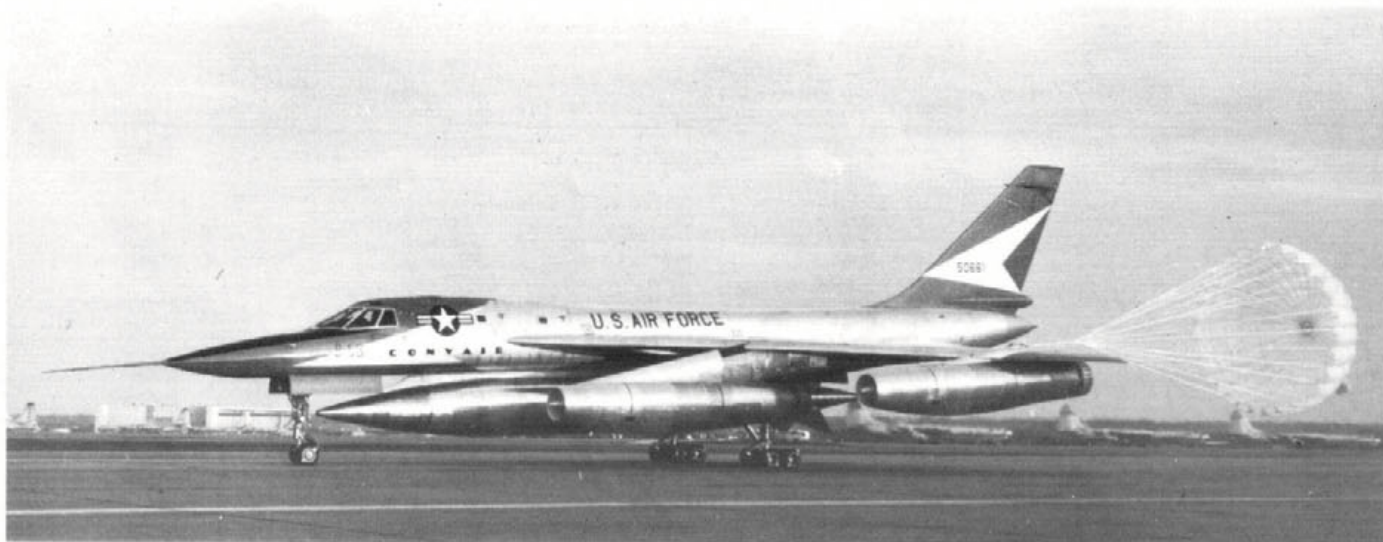
The second XB-58A, 50661, taxiing back to the Convair factory at Fort Worth after a routine test flight. The large braking parachute is clearly visible. Finish is identical to that of the first prototype. (Convair)
