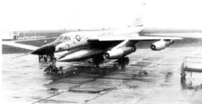
On a rare visit to the UK, B-58A 92434 'Cannonball' of the 43rd Bomb Wing stands on a rain-soaked tarmac at Upper Heyford during the early sixties. This particular aircraft carries the single component MB pod. (A. W. Hall)
