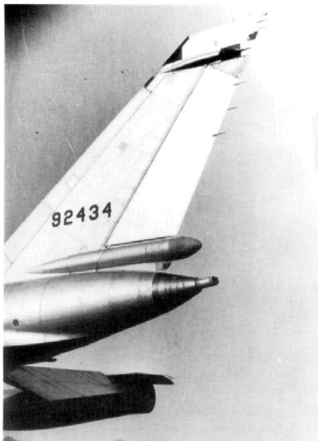
Above: The rearward facing Vulcan rotary cannon armament and its associated gunsight ranging radar are clearly visible in this close up of the fin of 92434. Flexible plates on the cannon installation permitted it to be aimed automatically by the fire control computer. (A. W. Hall) Below: Testing of the XB-70's massive General Electric J93-GE-3 turbojet engine was performed by the AFFTC on a specially modified NB-58A at Edwards AFB. This aircraft, 50662, carried the J93 in a pod beneath the fuselage. (via R. Alexander)
