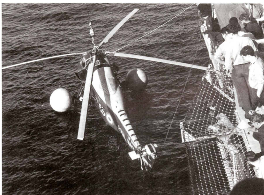
Above: Wessex HAS.1 XS888/E-065 of No.820 NAS being recovered from the sea in December 1968. The Wessex was kept afloat thanks to its inflatable float packs fitted onto the wheel hubs. Below: Wessex HAS.1 XP110/PO-776 of No.737 NAS based at Portland armed with anti-submarine missiles.
