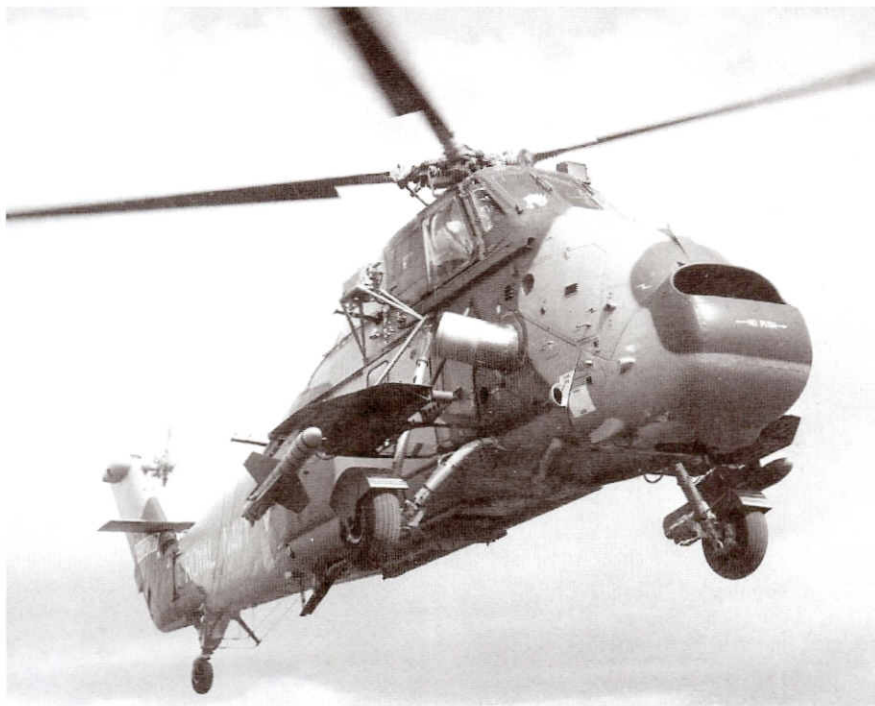
Wessex HU.5 in full battle attire with gun platform, missiles and wheel covers
