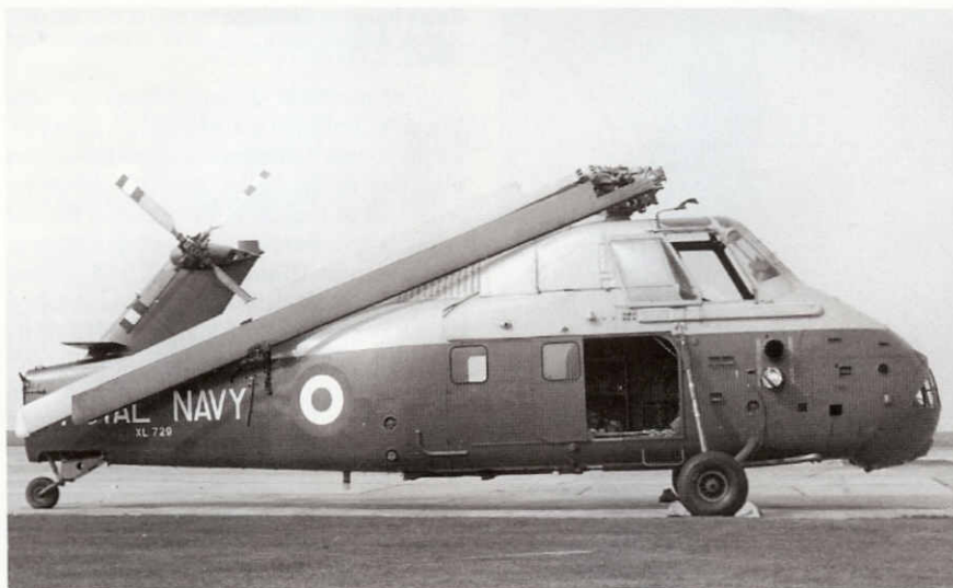
Wessex HAS.1 XL729, the third pre-production example built, fully retracted for easier stowage on ships. XL729's first assignment was with the A&AEE for handling trials in June 1959.
