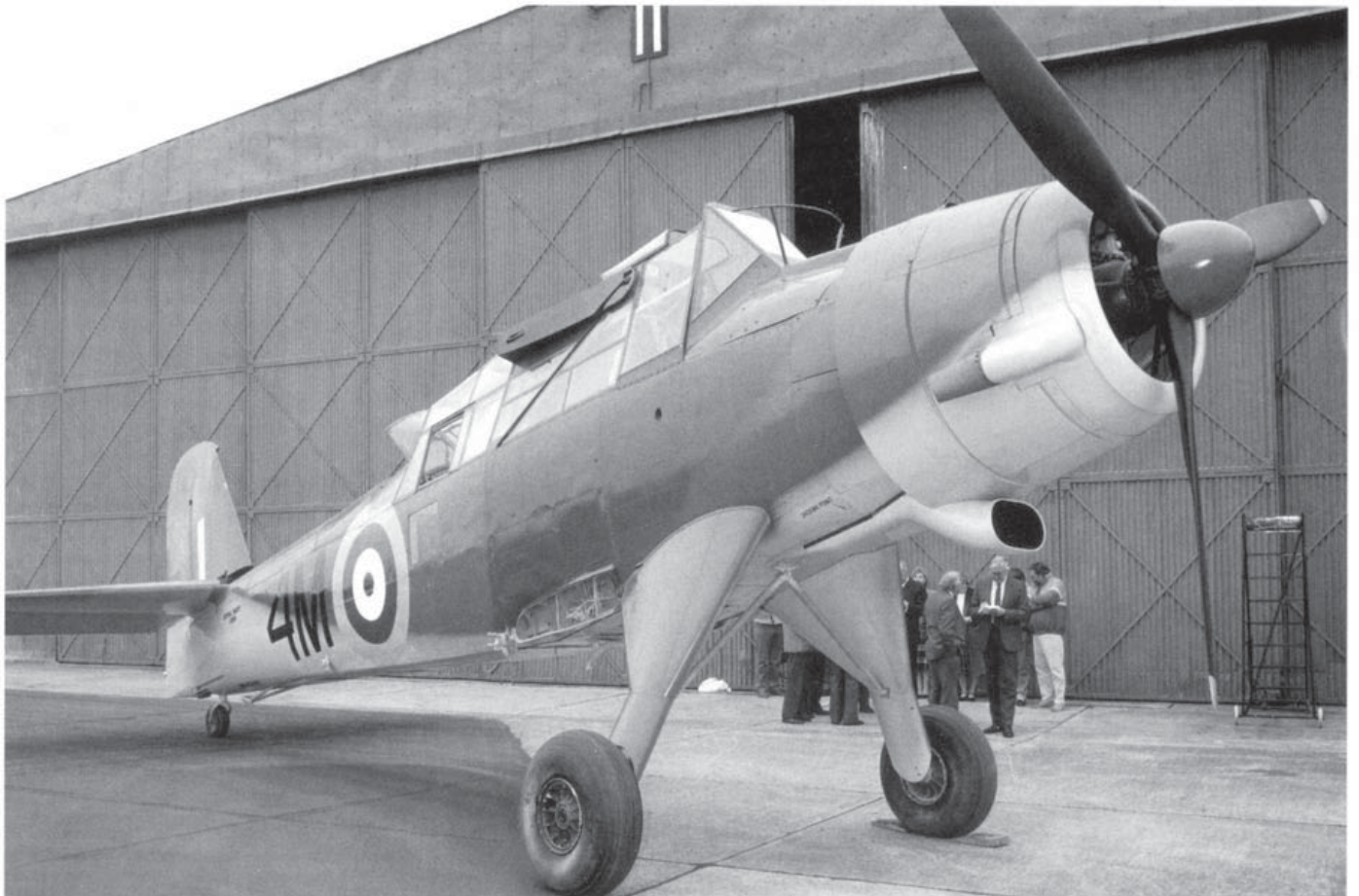
Above: With the wings removed the masses of detail become apparent. The crew door, cockpit glazed area showing the gunner's position, pilot's steps, torpedo sight, torpedo crutch, oil cooler intake and undercarriage stance. Below: A view from the starboard side of the Albacore again with lots of detail including the exhaust manifold and small window just ahead of the roundel. (FAA Museum)
