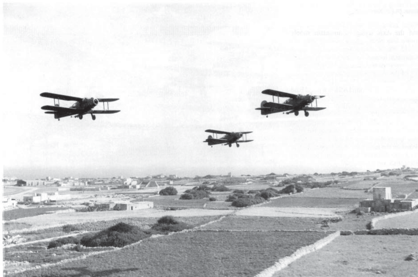
Three Albacores taking off from Malta. All three have a torpedo mounted with the air tail showing. Wartime pictures usually had the air tail censored out. (IWM)
