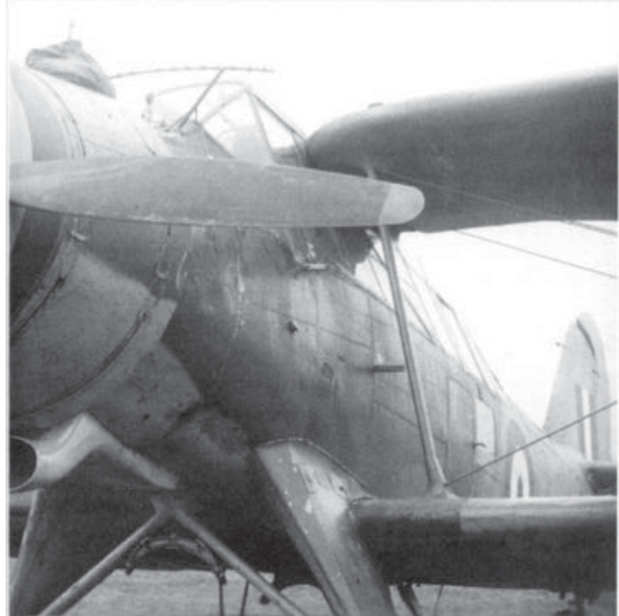
1. Pilot's cockpit from port side showing the windscreen frames. The plate on the cockpit wall is for Taurus II engine limits. 2. A port view of the Albacore cockpit, showing the blind flying panel, control column, throttle box. The seat and P compass have been removed to get a better view. 3. The Albacore's forward section. Torpedo sight not fitted. 4. One Albacore was tested at Boscombe Down with cuffs on the propeller roots to see if they would improve performance – it didn't! 5. Observer's position in Albacore with limited panel showing height, ASI, and air temperature gauge. On the other side of window is a voltage regulator for lights, wireless and compass. Below the fuse panel extreme left is storage area for the navigation instrument holdall. 6. An observer poses in the rear cockpit of Albacore X8954:K of 821 Squadron showing rear cockpit area and entrance (I. Templar) 7. Entry to the rear cockpit of an Albacore of 821 Squadron during its time in the Western Desert. (I. Templar)
