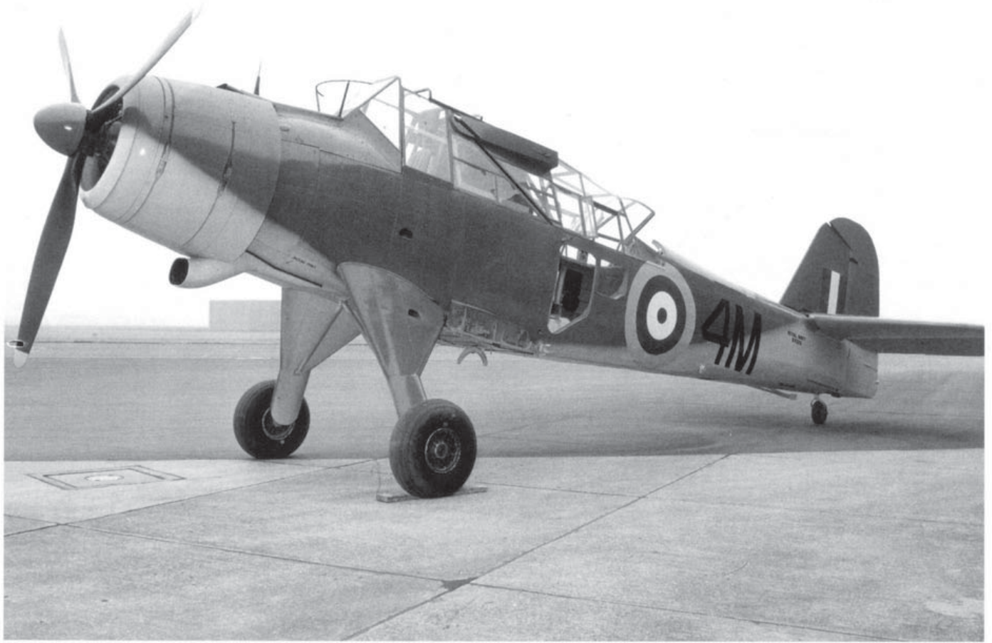
Above: With the wings removed the masses of detail become apparent. The crew door, cockpit glazed area showing the gunner's position, pilot's steps, torpedo sight, torpedo crutch, oil cooler intake and undercarriage stance. Below: A view from the starboard side of the Albacore again with lots of detail including the exhaust manifold and small window just ahead of the roundel. (FAA Museum)
