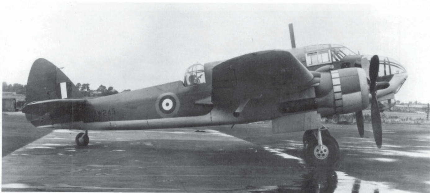
The second production Beaufort Mk.II AW245, brand new and without turret guns, poses for the camera on a wet day. This was one of ten 'Interim' Mk.IIs delivered without ASV radar. Note the different nacelles and spinners from the Mk.I. (Peter Green)
