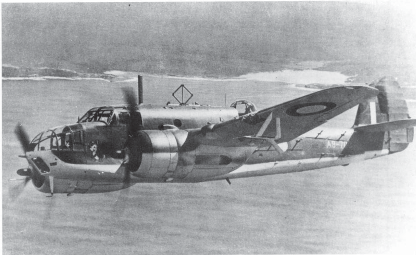
Above: The last Australian-built Beaufort was A9-700 which stayed with the manufacturers and lasted until 1949. Note the complex array of antennae for the sideways-looking ASV IIB radar with its underlying Yagi receiving aerials. This machine also sported 0.5in (12.7mm) wing guns. (Peter Green)
