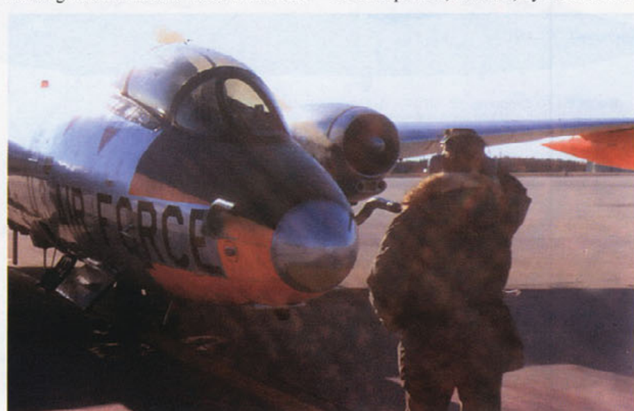
This nose-on view of an EB-57E shows the nose waveguide horns installed later in the type's career. Also clearly defined are the various colours applied to the airframe. (John Harris)
