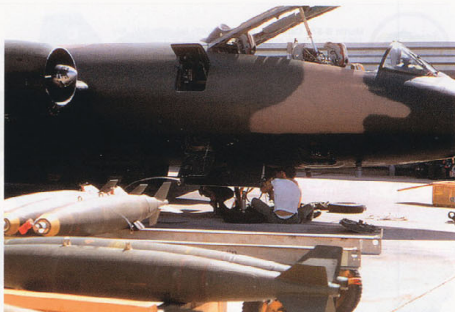
Inside its revetment at Phan Rang AB, this B-57B undergoes rectification of its nose wheels after which a pre-flight including arming was to be carried out. (Mark de Witt)
