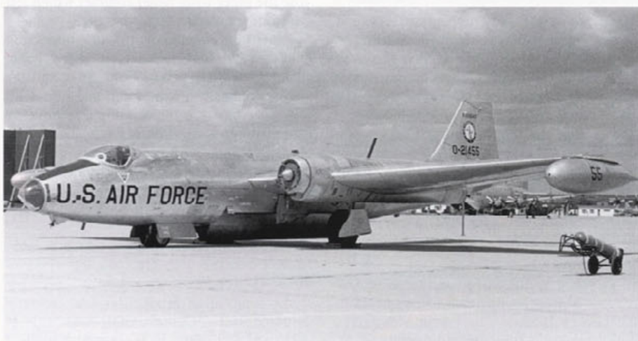
This three-quarter front view of a Kansas Air National Guard RB-57A reveals the extra ailerons under the nose and the bomb door in a partially open position. (BBA archives)
