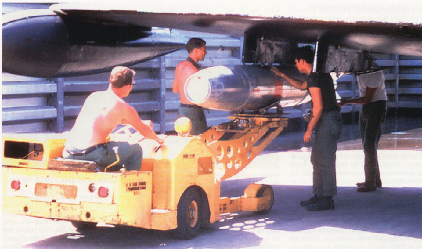
Using a weapons loader the armourers load a silver painted napalm tank under the wing of a B-57 in Vietnam. (Mark de Witt)
