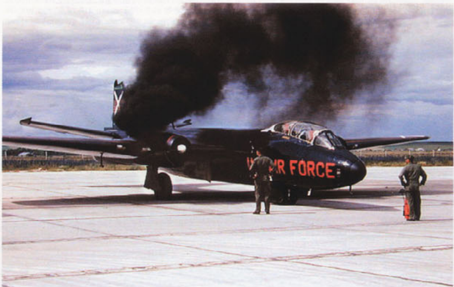
Below: Starting the B-57 was a smoky and messy business as this picture shows. Eventually a cleaner cartridge was developed. The 'X' symbol on the fin and wings indicate that this was an exercise participant, the aircraft actually belonging to the 38th TBG based at Laon, France. (John Harris)
