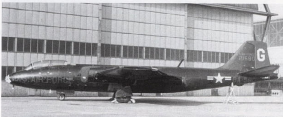
Above: Outside the maintenance hangar at Laon AB, France, this B-57B of the 38th TBG has a trestle under the rear fuselage to support the aircraft when the fuel load was minimal. Below: B-57B showing the variety of underwing stores that could be carried. These included rockets and in this case napalm tanks as well as the internal bomb bay (BBA Archives)
