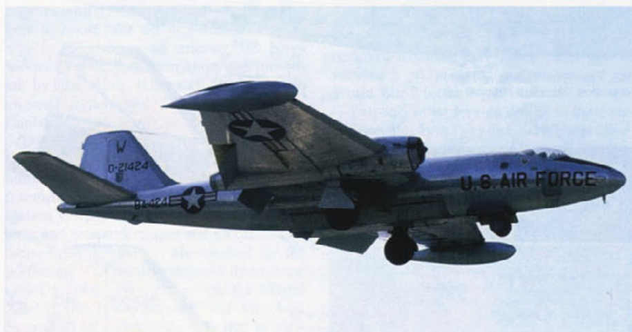
Complete with solid nose that replaced the original transparent one, this B-57A, 52-1424, has its undercarriage and flaps lowered in preparation for landing. (BBA archives)
