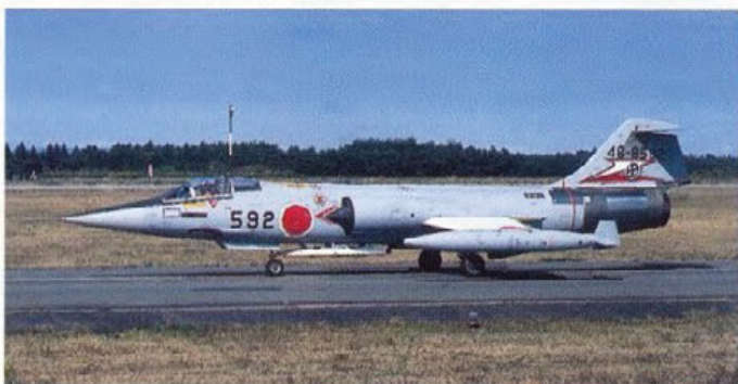
Below: This interesting picture shows 46-8592, of the 207 Hikotai with an attachment under the forward fuselage for carriage of cameras or additional fuel tanks. (via Terry Panopalis)
