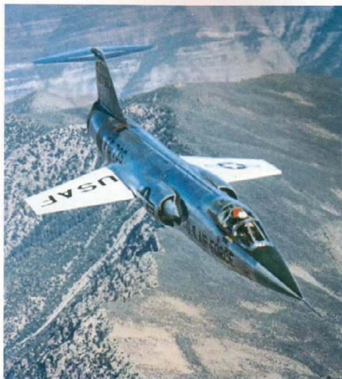
F-104A Starfighter 56-736 was the seventh Starfighter to fly and was used throughout its career as an experimental aircraft with Lockheed. This picture graphically illustrates the white upper wing surfaces (via T. Panopalis)
