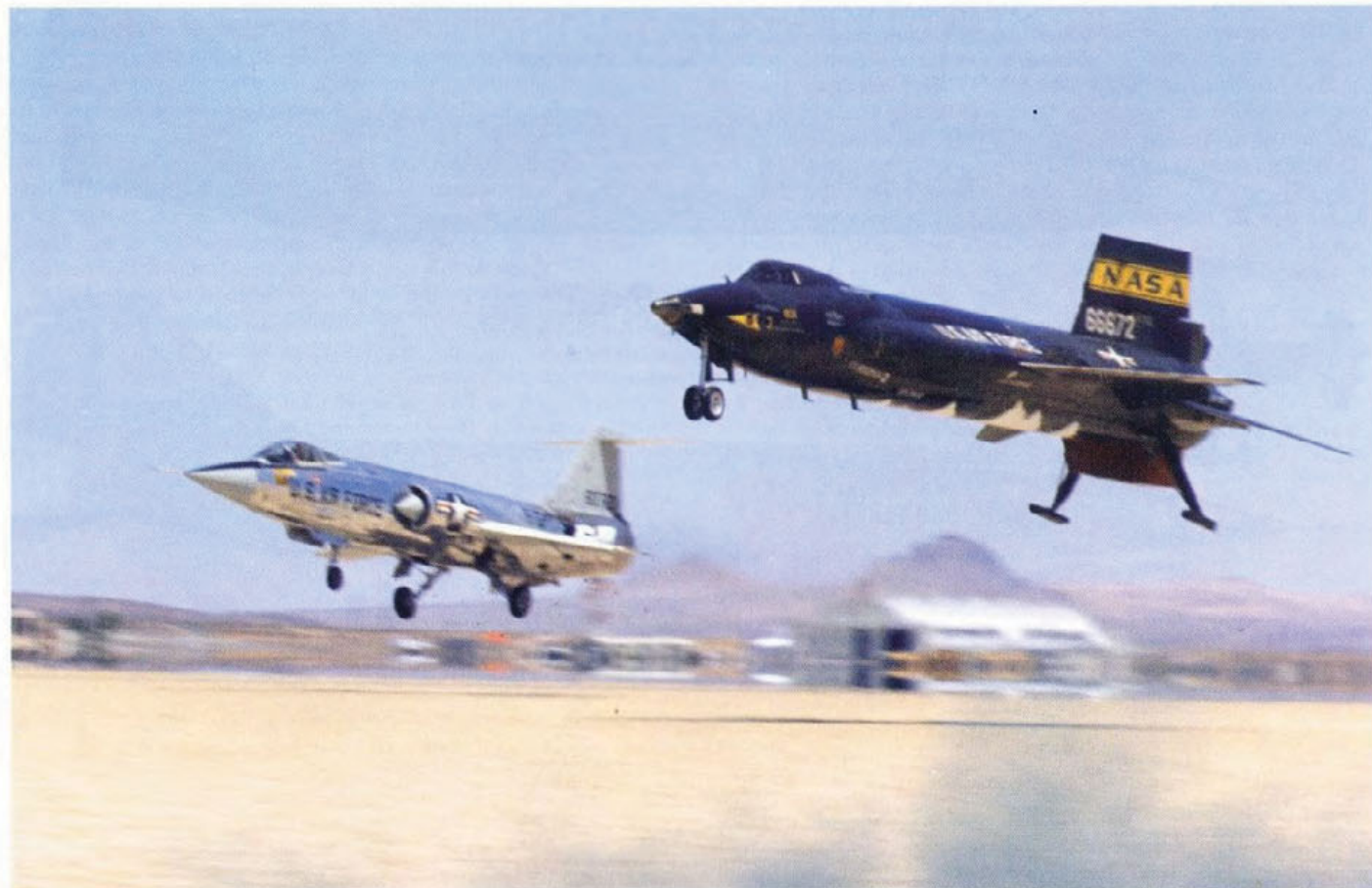
Above: One of four NF-104As converted for the Aerospace Pilots School which featured an additional 6,000 lb thrust Rocketdyne LR121-NA-1 in the tail and used to train pilots for the critical re-entry point after a space flight. Below: The F-104A used as a chase aircraft in this case of the X-15 research aircraft. (via Terry Panopolis)
