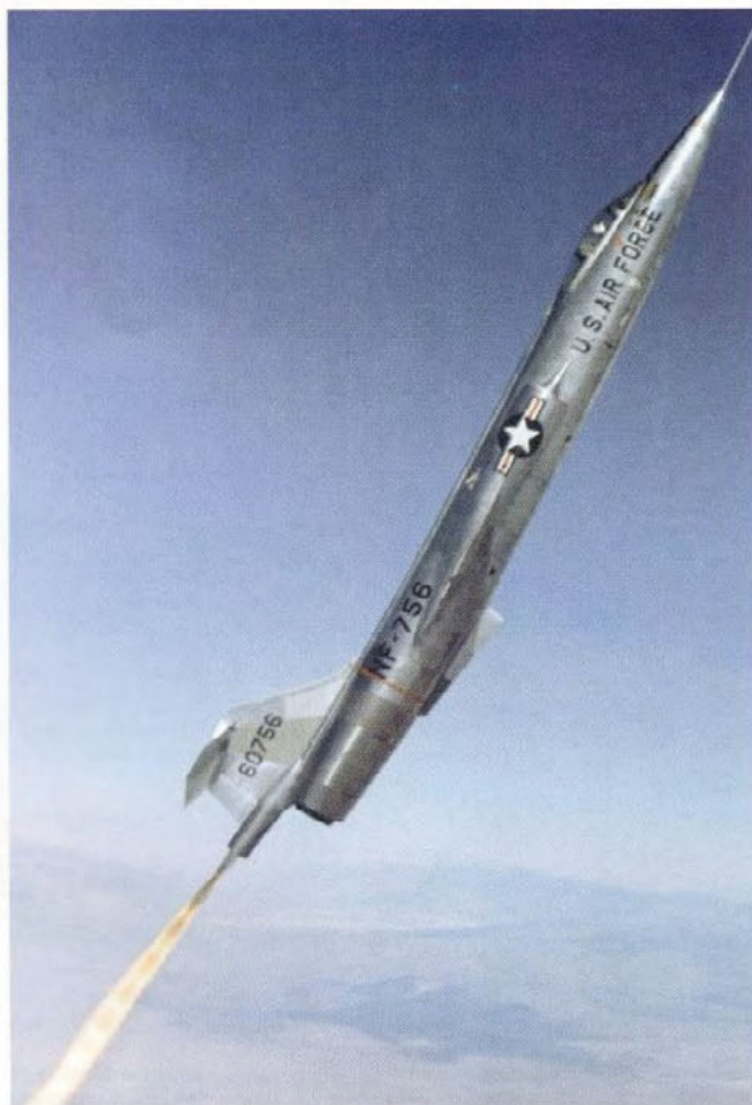
Above: One of four NF-104As converted for the Aerospace Pilots School which featured an additional 6,000 lb thrust Rocketdyne LR121-NA-1 in the tail and used to train pilots for the critical re-entry point after a space flight. Below: The F-104A used as a chase aircraft in this case of the X-15 research aircraft. (via Terry Panopolis)
