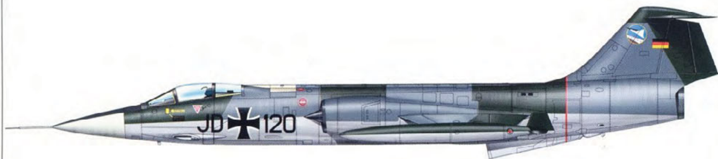
F-104G Starfighter JD+120 of JG 74, Federal German Air Force (Luftwaffe), Neuburg, 1966. Dark Grey RAL 7012 (FS.26152) and Dark Green (FS.34079) RAL 6014 upper surfaces with Aluminum RAL 9006 undersides. National markings in standard six positions.
