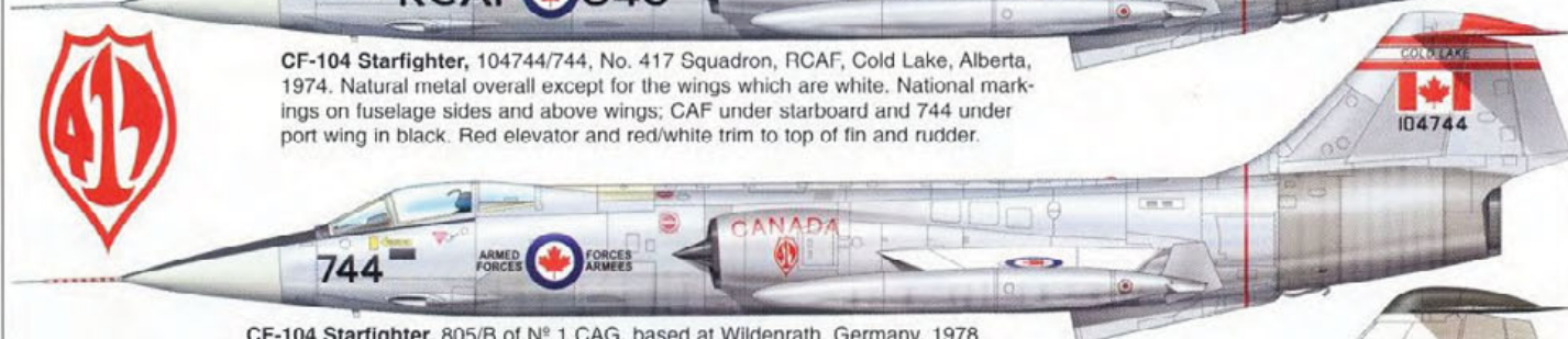
CF-104 Starfighter, 805/B of N° 1 CAG, based at Wildenrath, Germany, 1978. Scheme is Dark Green (FS.34016) overall with the national markings on fuselage sides and above wings; CAF under starboard and 805 under port wing in black. The white tail and red Maple Leaf were painted for a special exercise in June of that year.
