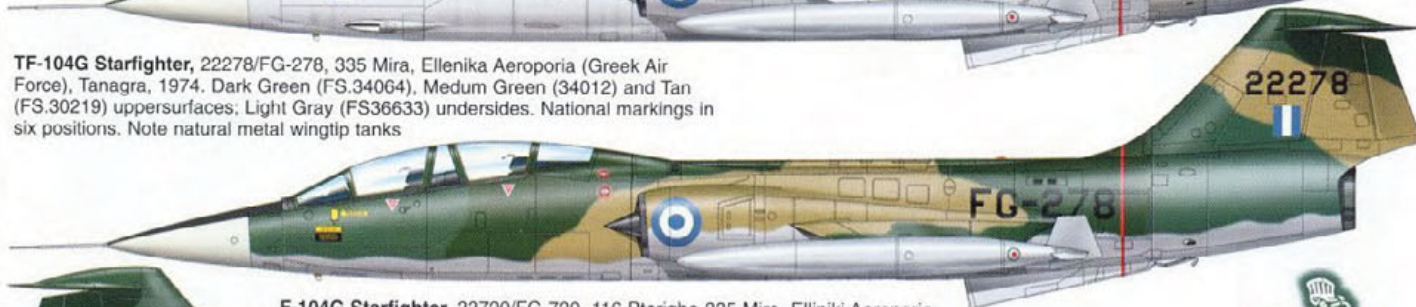
F-104G Starfighter , 33720/FG-720, 116 Pterighe-335 Mira, Elliniki Aeroporia, during a visit to Volkel AB in July 1970. Dark Green (FS.34064), Medium Green (34012) and Tan (FS.30219) uppersurfaces; Light Gray (FS36633) undersides. National markings in six positions. Note 'Dusty' character in white
